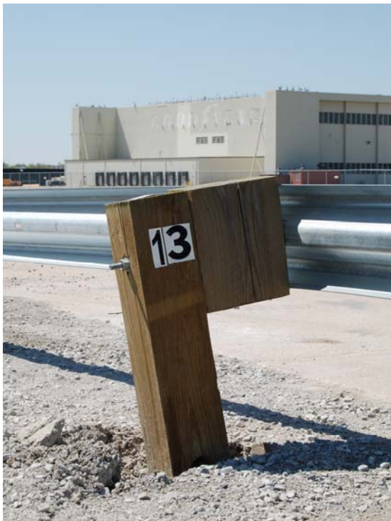
Figure 33. System Post Damage, Test No. LSC-1
