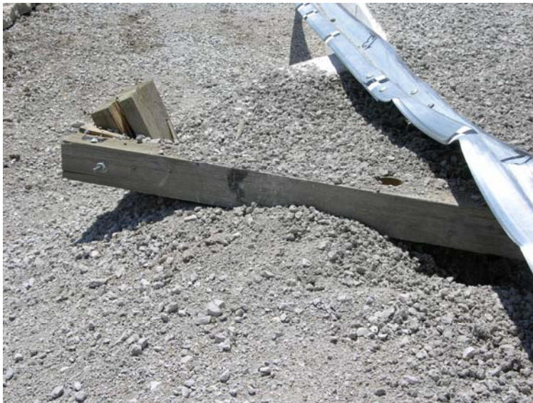
Figure 61. System Post Damage, Test No. LSC-2
