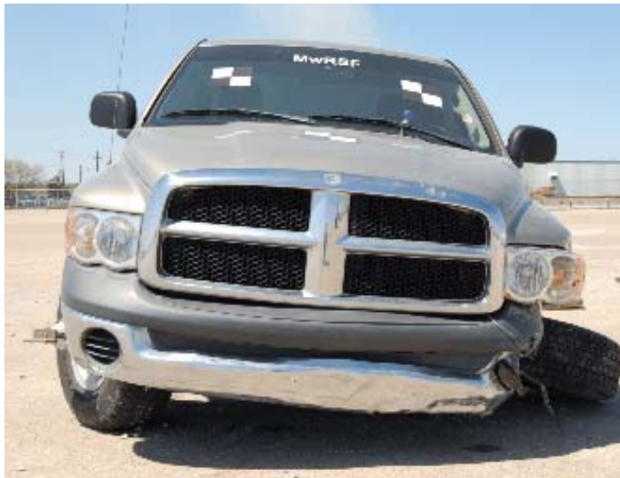
Figure 37. Vehicle Damage, Test No. LSC-1
