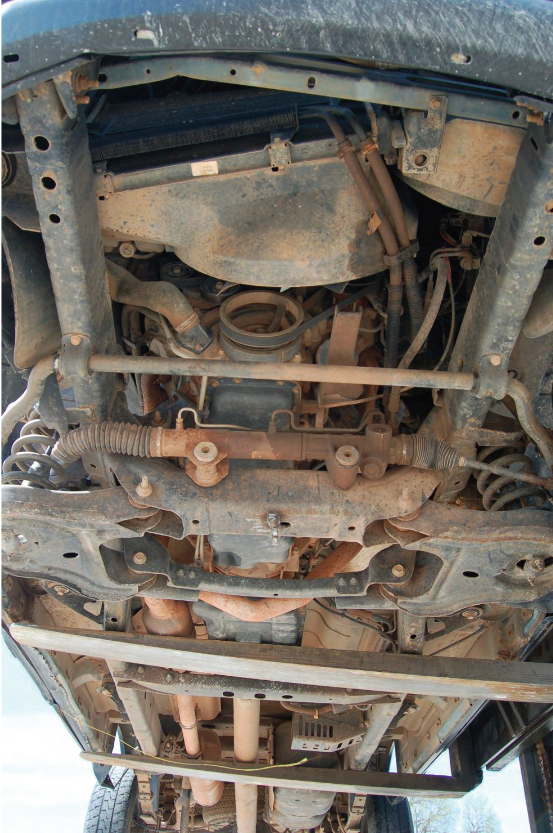
Figure 40. Vehicle Undercarriage Damage, Test No. MGSWP-1
