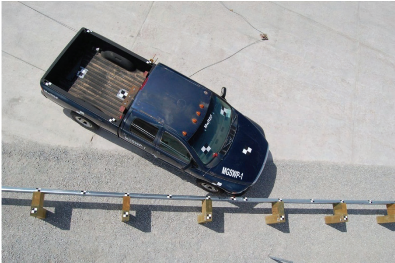
Figure 27. Impact Location, Test No. MGSWP-1
