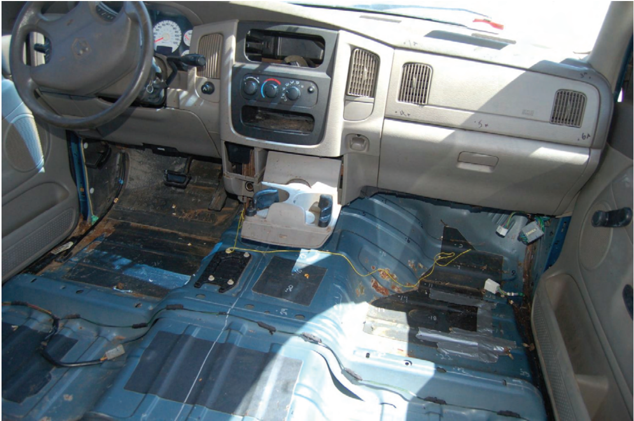
Figure 41. Occupant Compartment Damage, Test No. MGSWP-1
