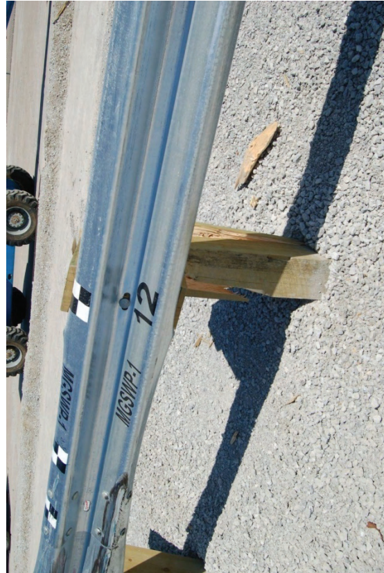
Figure 34. Post Nos. 11 and 12 Damage, Test No. MGSWP-1
