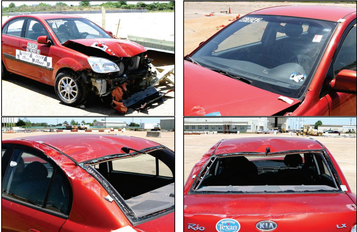
Figure 4.9. Vehicle after Test No. 467824-2.
