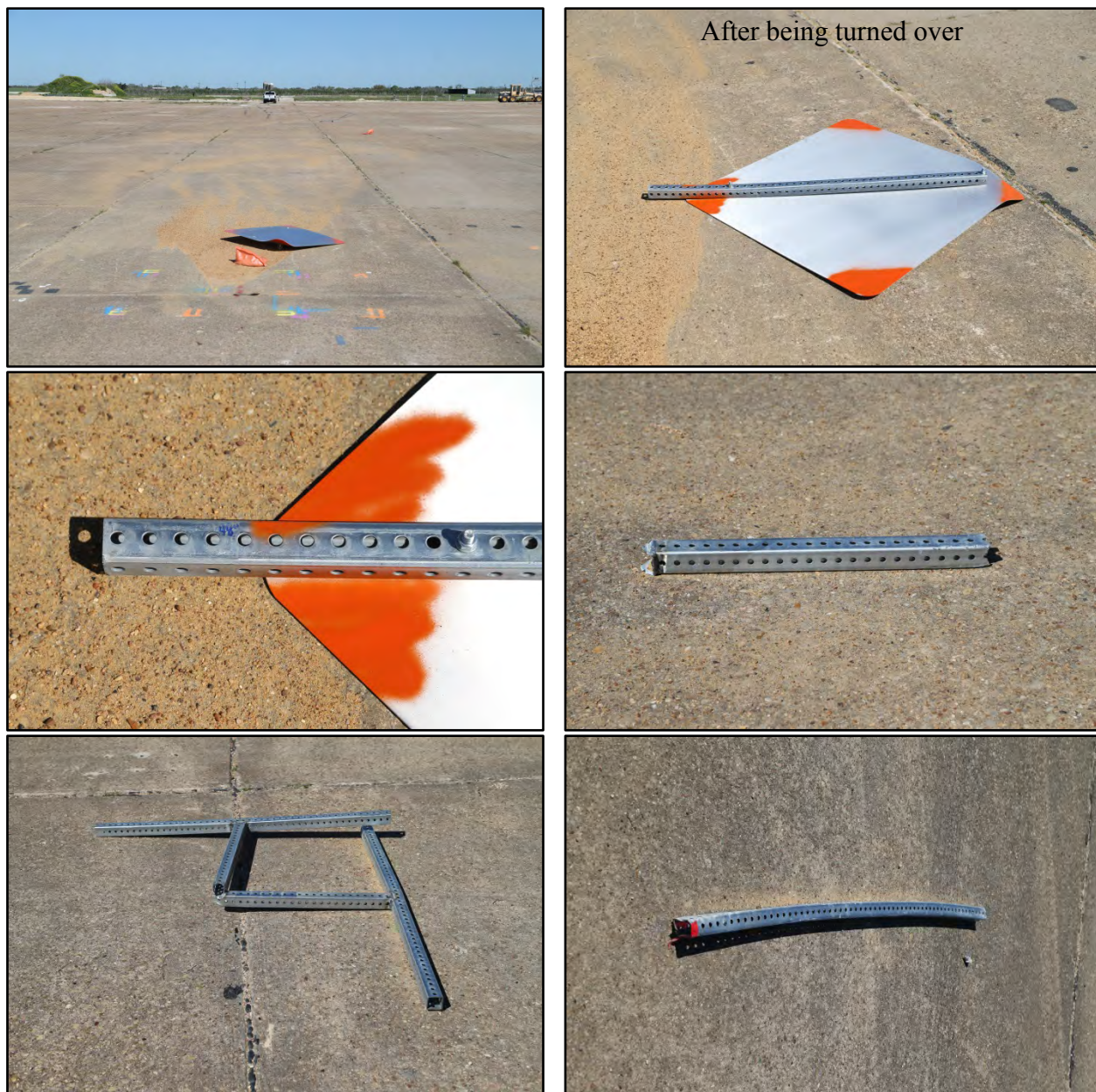
Figure 7.22. Option C Temporary Work Zone Sign Support after Test No. 490026-2-9.
