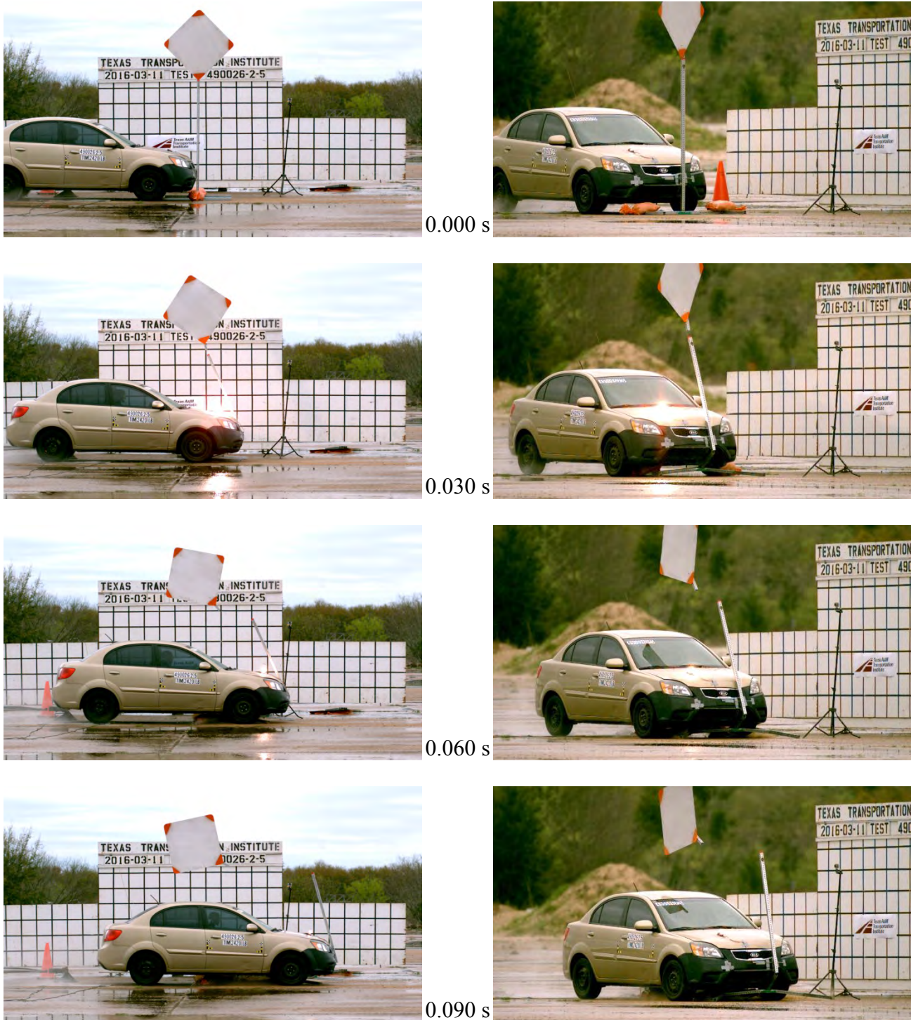
Figure G.1. Sequential Photographs for Test No. 490026-2-5 (Perpendicular and Oblique Views).
