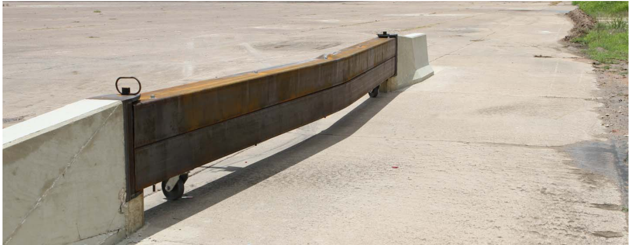
Figure 7.4. TxDOT Median Barrier Gate after Test No. 420020-7.
