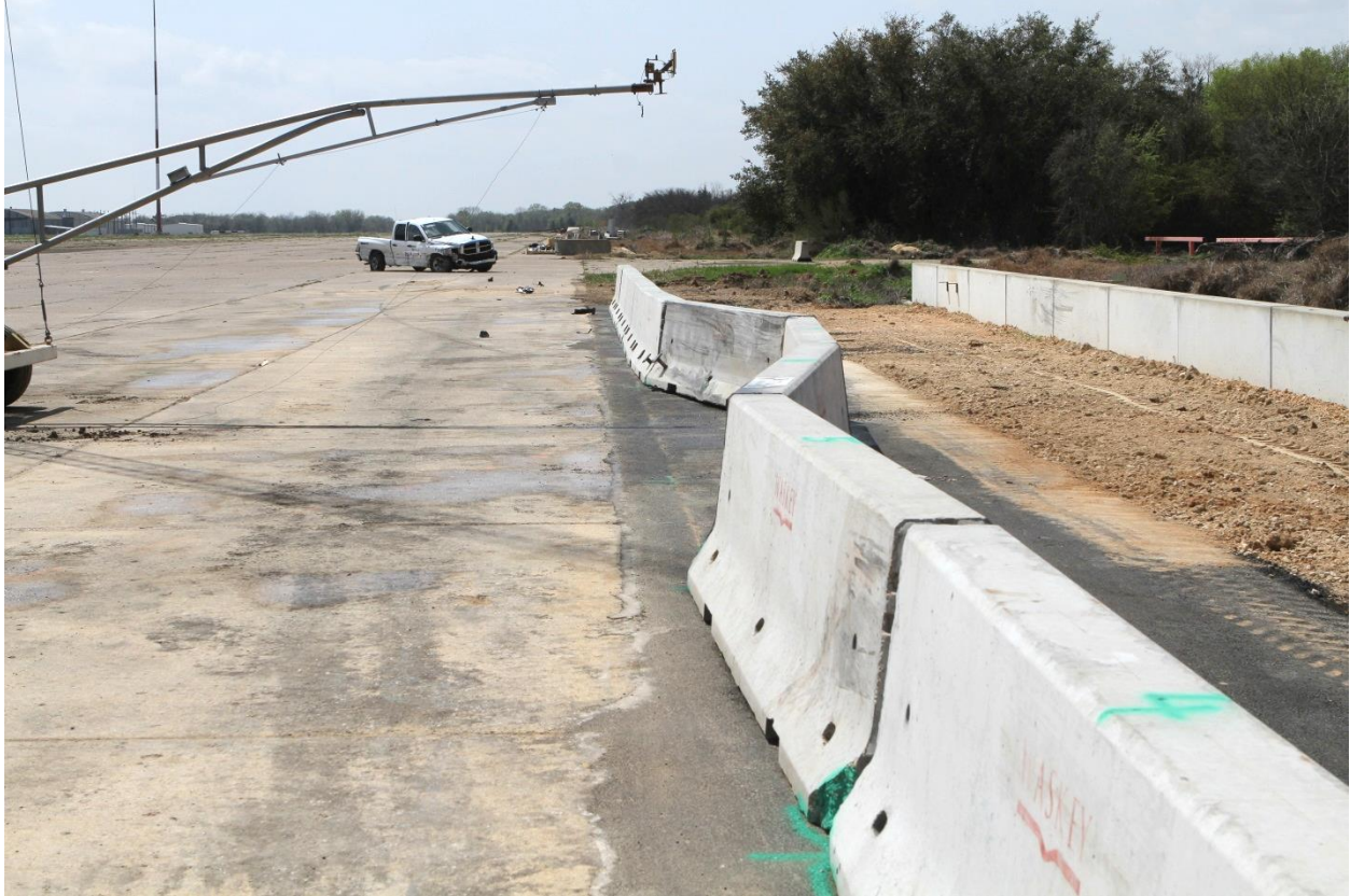
Figure 5.9. Vehicle and installation positions after test 601651-1.
