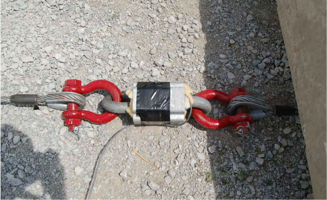
Figure 6. Tensile Load Cell Location, Test No. MGSEA-1
