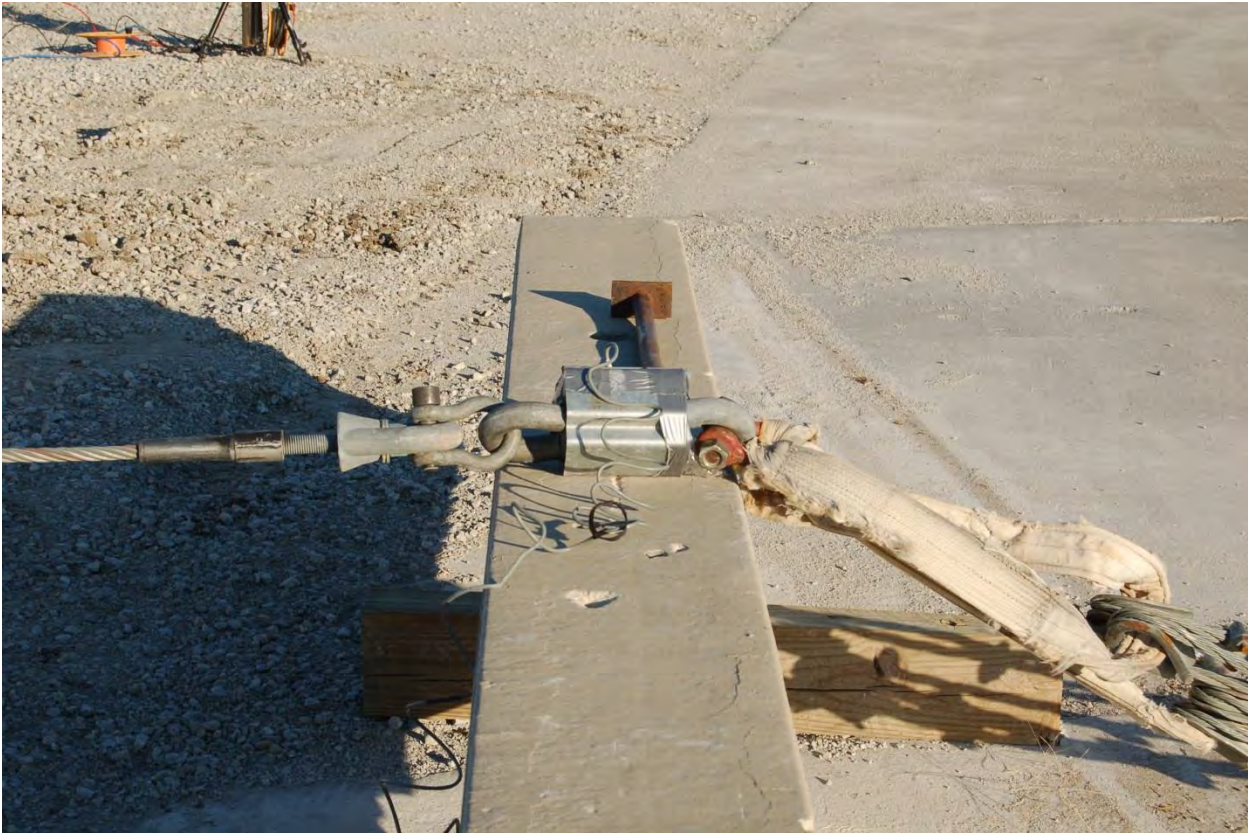
Figure 52. Load Cell Setup, Test Nos. DSAP-1 and DSAP-2
