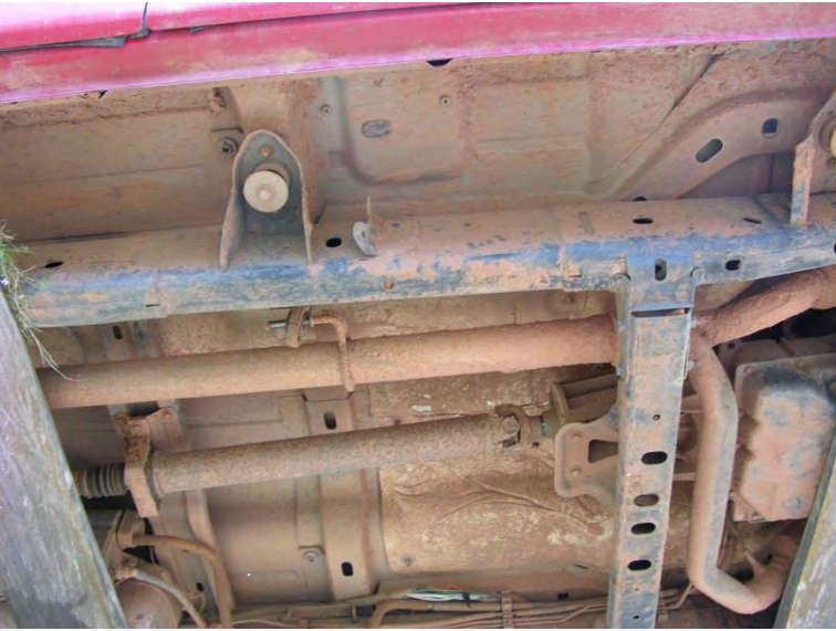
Figure 144. Undercarriage and Suspension Damage, Test No. WIDA-1
