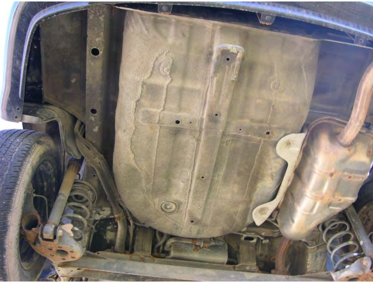
Figure 161. Vehicle Undercarriage Damage, Test No. WIDA-2
