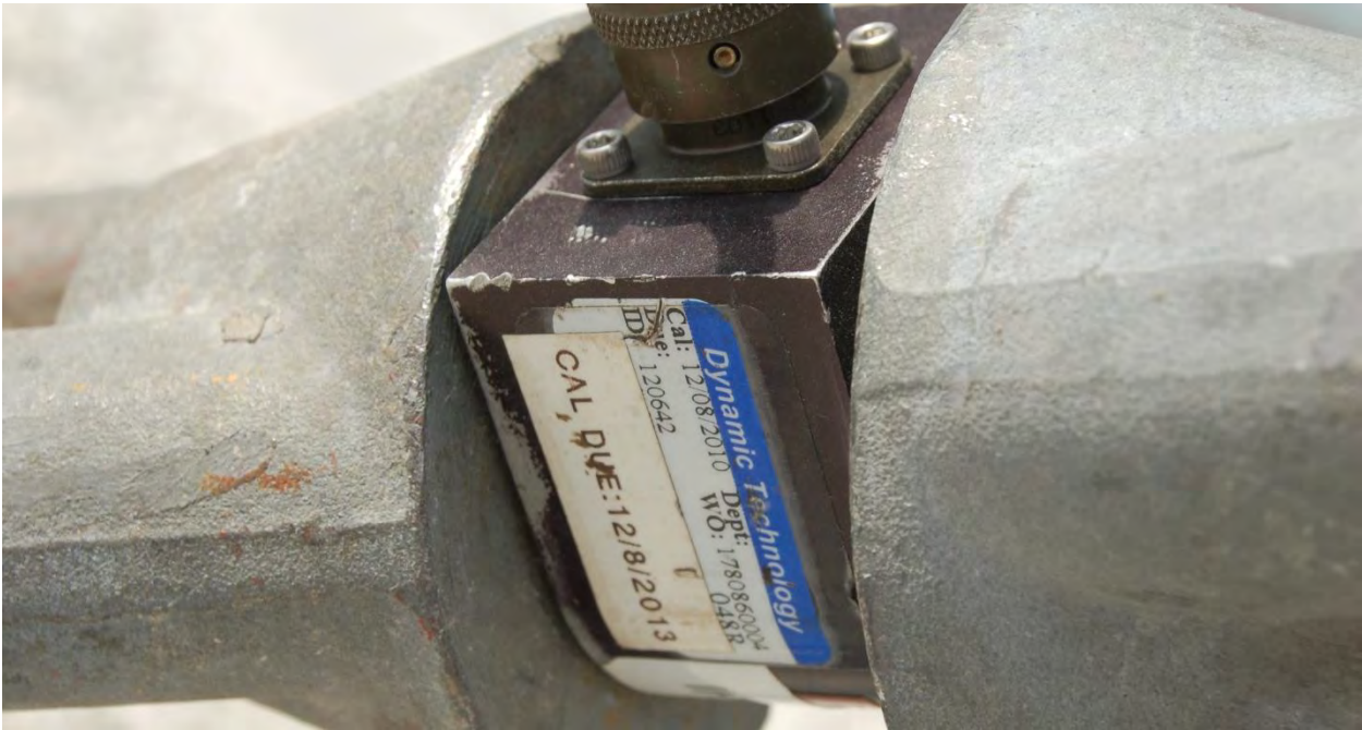
Figure 101. Load Cell Setup, Test No. WIDA-1
