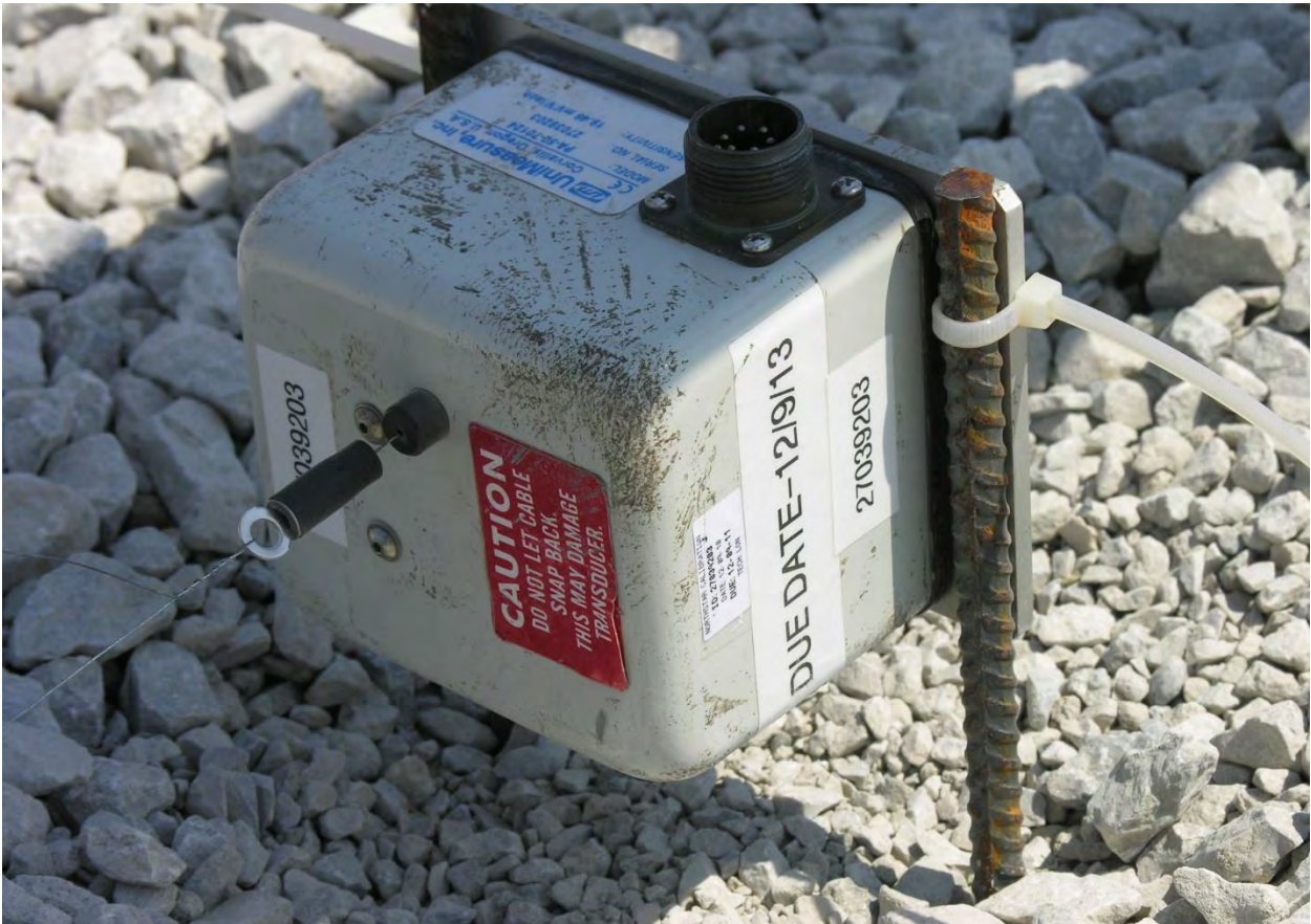
Figure 102. String Pot Setup, Test No. WIDA-1
