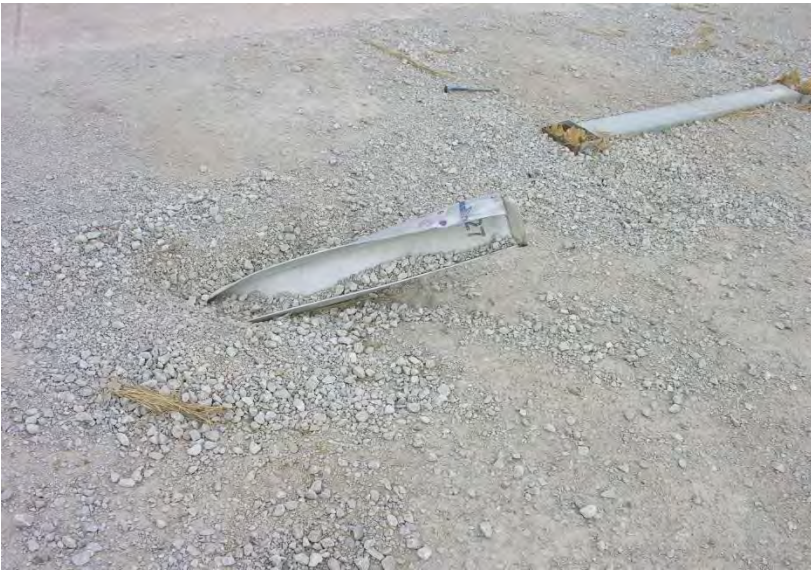
Figure 140. System Damage at Post Nos. 25 through 29, Test No. WIDA-1
