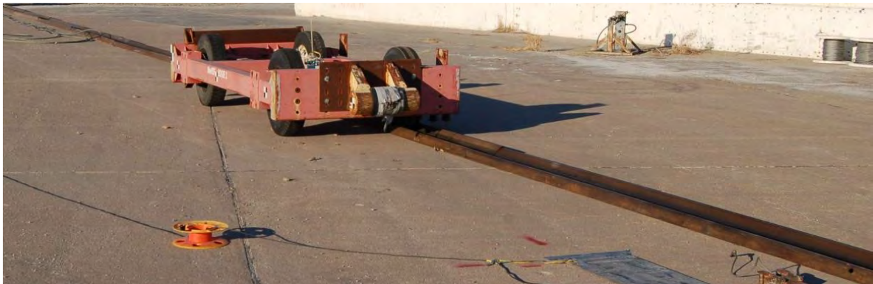
Figure 5. Rigid-Frame Bogie used for Test Nos. MGSEA-1, DSAP-1, and DSAP-2
