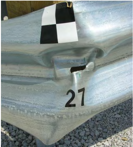
Figure 154. Rail Damage, Test No. WIDA-2
