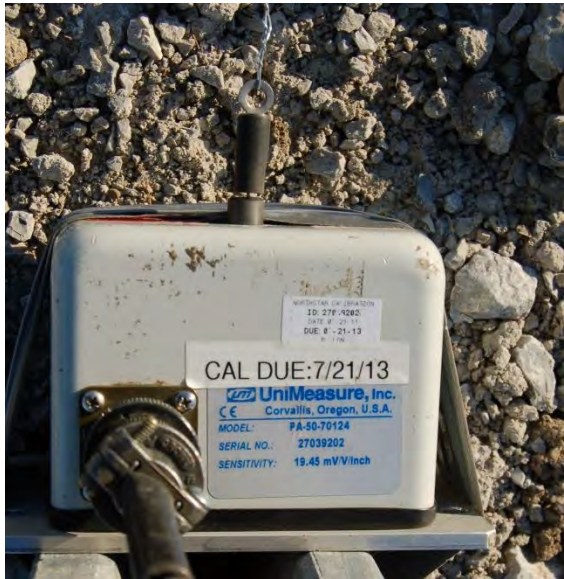
Figure 9. String Pot Backup Structure and Attachment Location, Test Nos. MGSEA-1, DSAP-1 and DSAP-2
