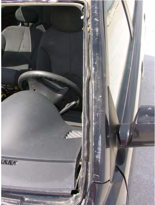
Figure 160. Vehicle Damage - Windshield, Test No. WIDA-2
