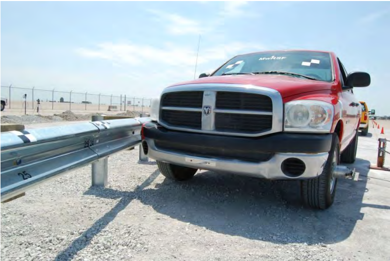
Figure 134. Impact Location, Test No. WIDA-1
