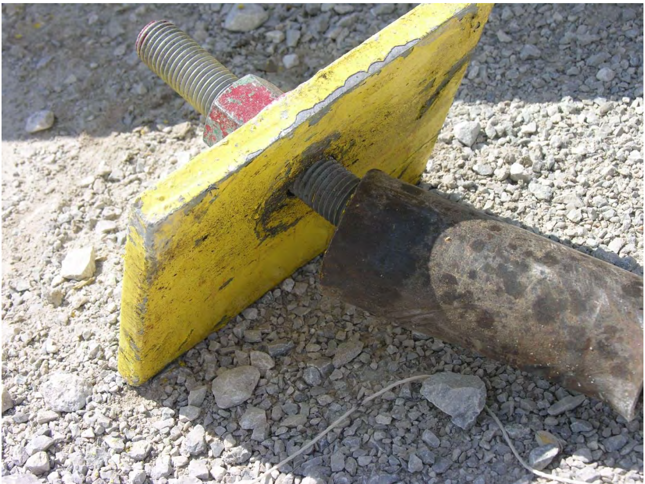
Figure 156. Anchor Cable Damage, Test No. WIDA-2
