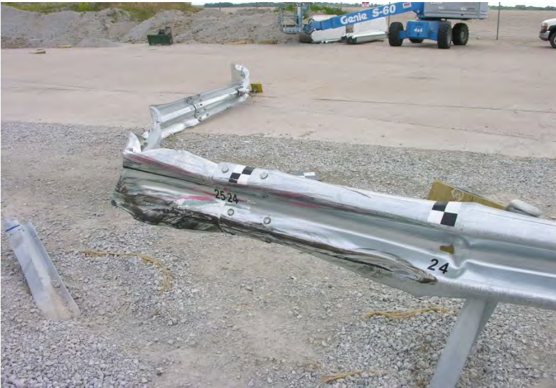
Figure 138. Details of Rail Damage, Test No. WIDA-1
