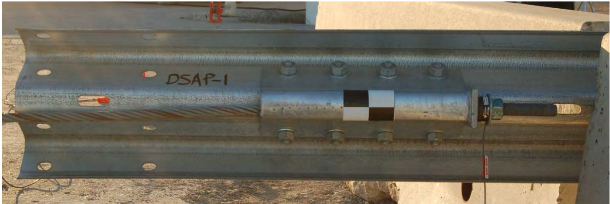
Figure 8. Compressive Load Cell Placement, Test No. DSAP-1
