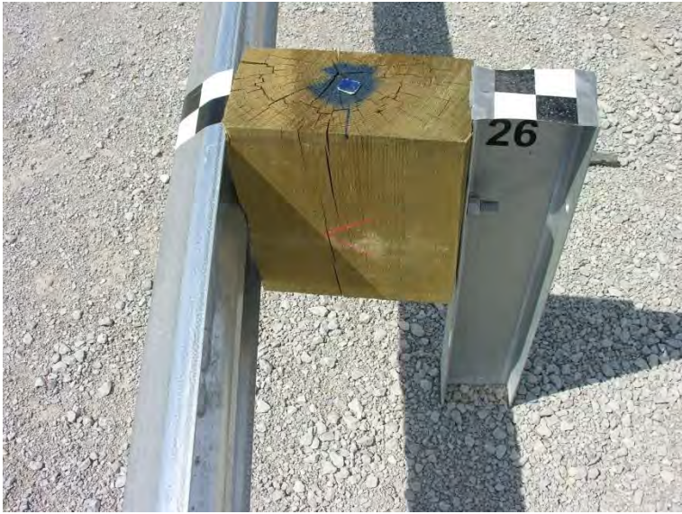
Figure 155. System Damage at Post Nos. 25 through 29, Test No. WIDA-2
