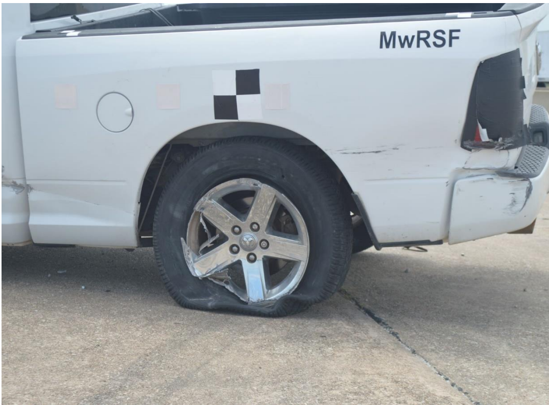
Figure 81. Left-Side Vehicle Damage, Test No. GSH-2
