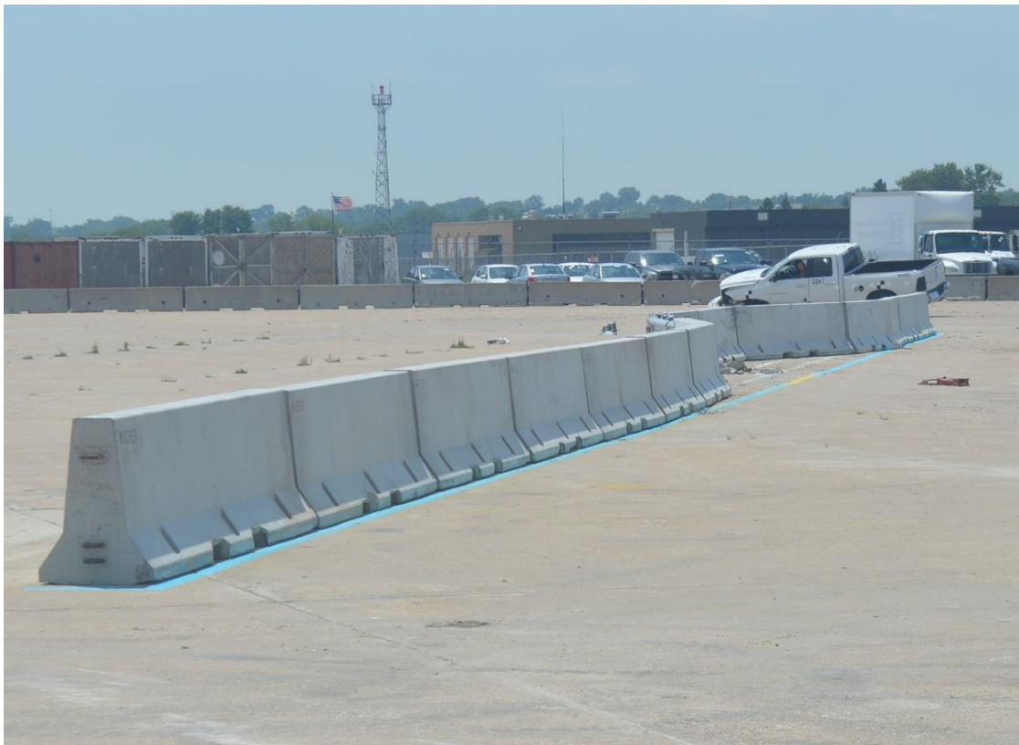
Figure 36. Overall System Damage, Test No. GSH-1
