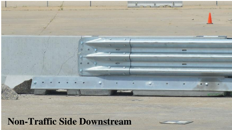
Figure 76. PCB Gap-Spanning Hardware Connection Damage, Test No. GSH-2
