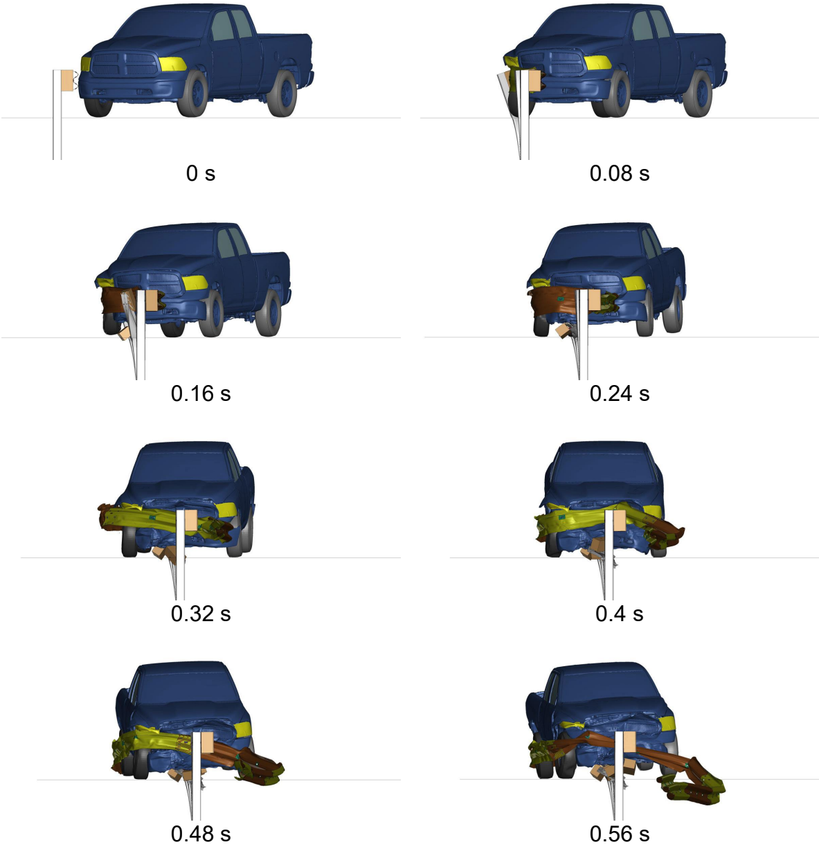
Figure 7.41. 137.5-ft Guardrail System with Refined Slot Mesh – Downstream View of MASH Test 3-11
