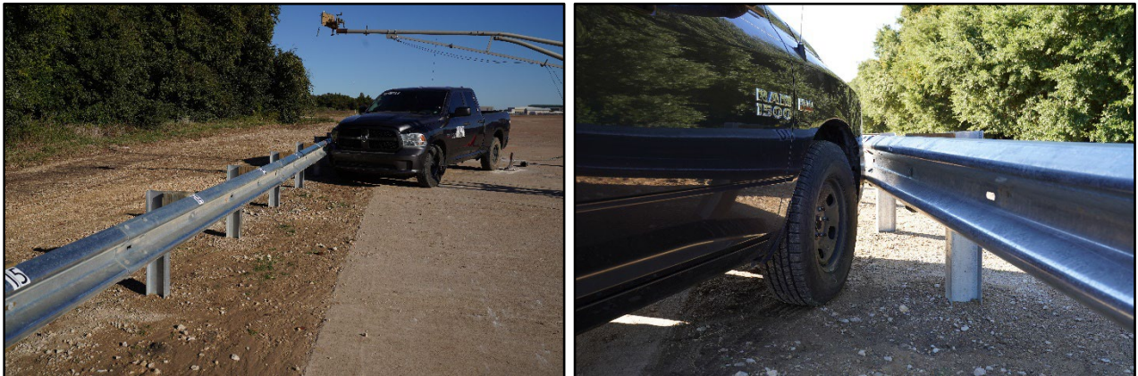
Figure 8.1. Guardrail without downstream anchorage/Test Vehicle Geometrics for Test No. 614721-01-1.
