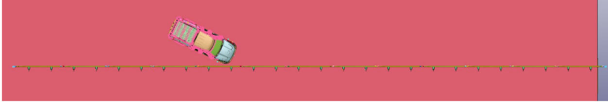
Figure 2.2. Overhead View of Impact Point for 162.5-ft Long Guardrail System Simulation
