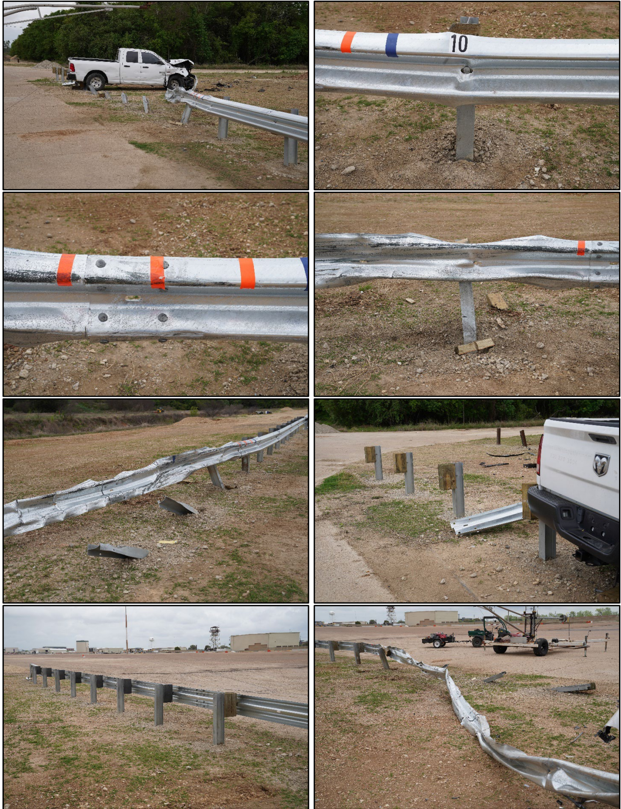
Figure 6.3. Guardrail without downstream anchorage after Test No. 614721-01-2.
