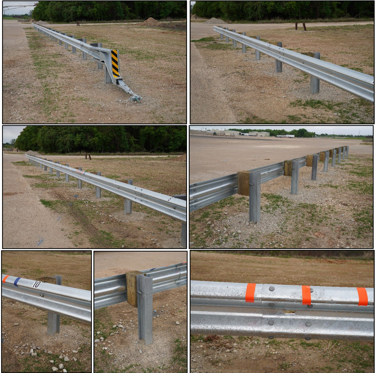
Figure 3.2. Guardrail without downstream anchorage prior to Testing.
