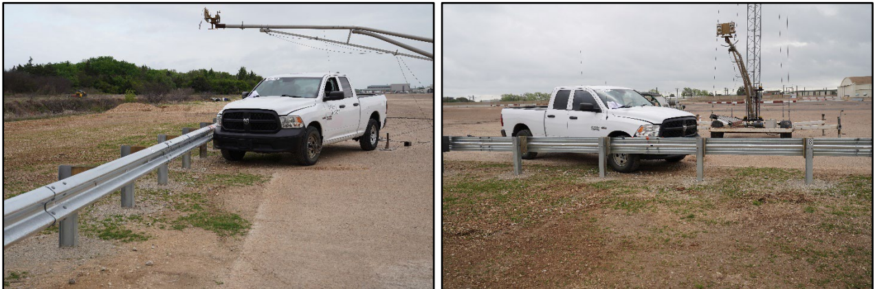
Figure 6.1. Guardrail without downstream anchorage/Test Vehicle Geometrics for Test No. 614721-01-2.
