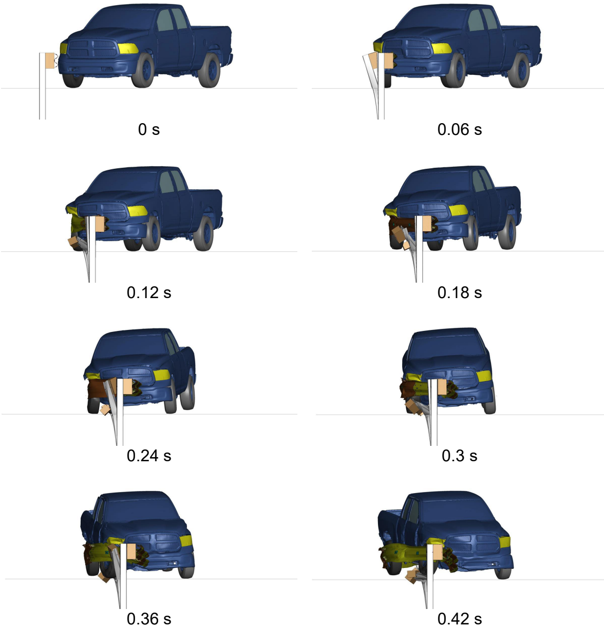
Figure 7.71. 225-ft Guardrail System with Refined Slot – Downstream View of MASH Test 3-11
