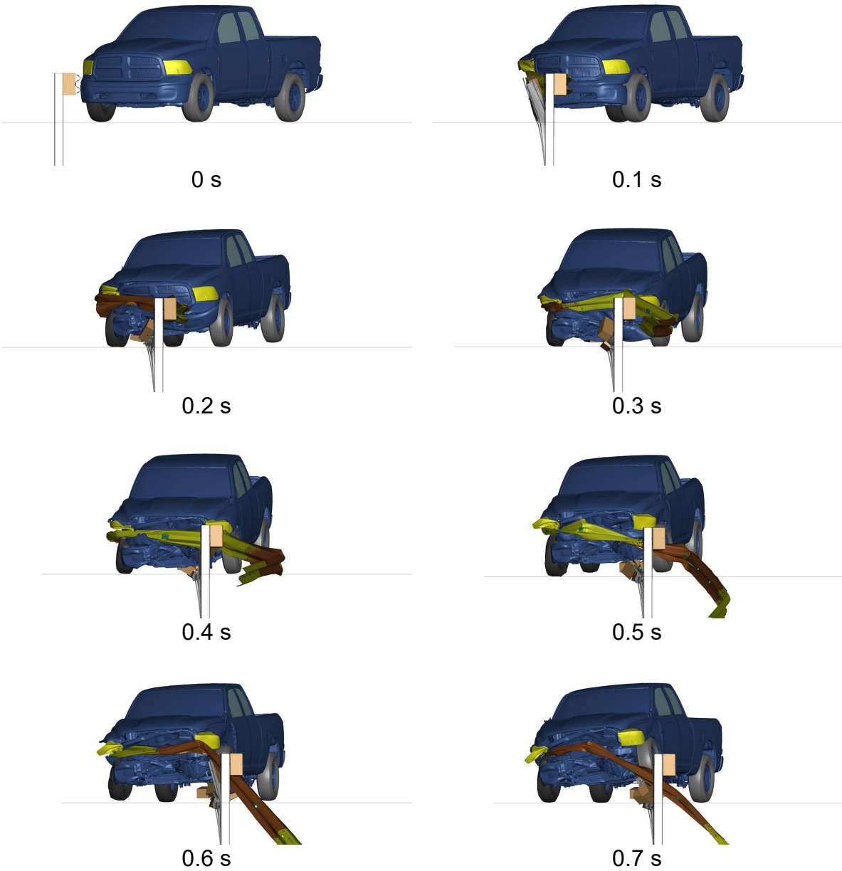
Figure 7.17. 87.5-ft Guardrail System with 2.5 mm Slot Elements – Downstream View of MASH Test 3-11
