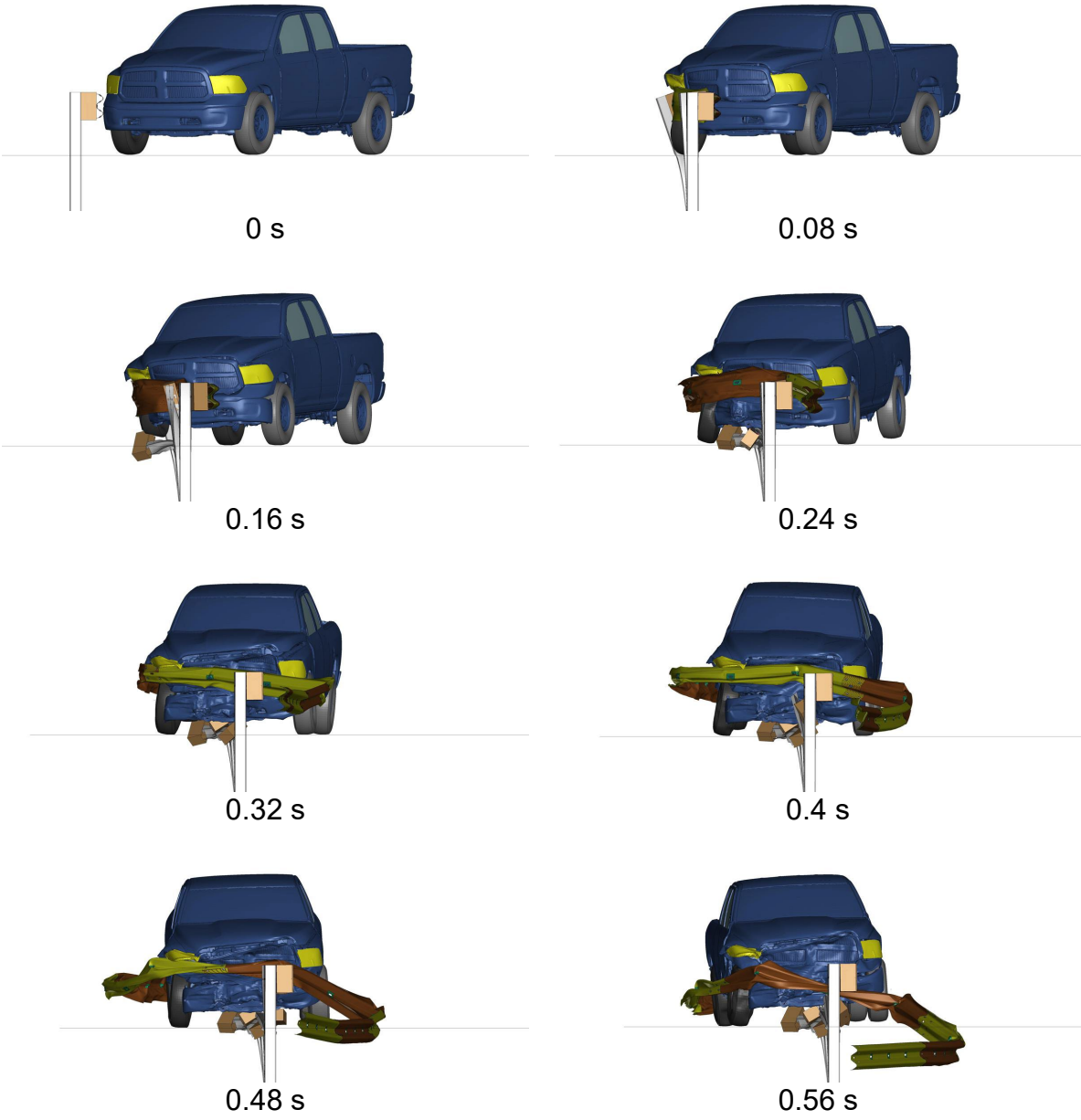
Figure 7.35. 112.5-ft Guardrail System with Refined Slot Mesh – Downstream View of MASH Test 3-11
