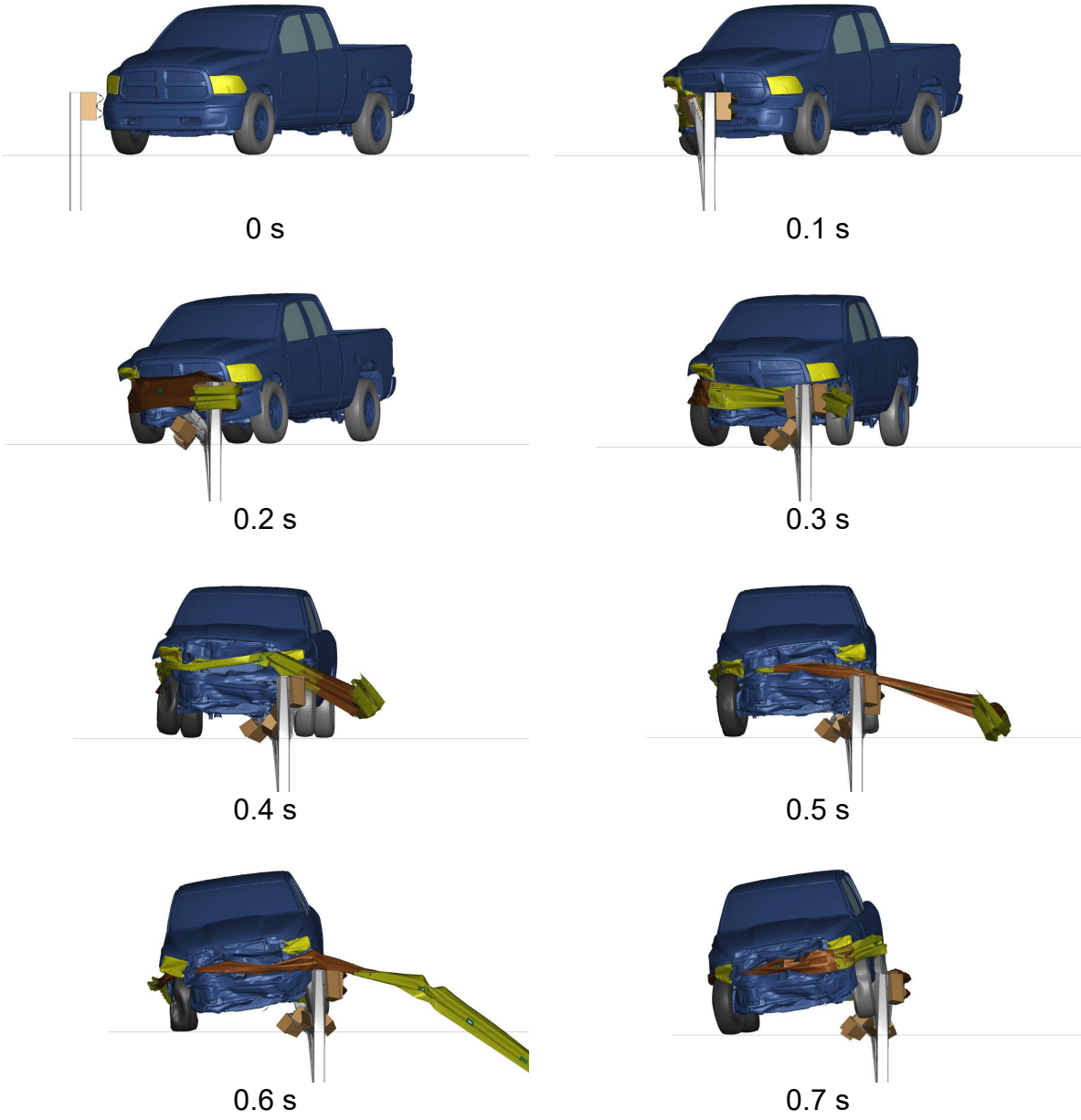
Figure 7.29. 87.5-ft Guardrail System with 1 mm Slot Elements – Downstream View of MASH Test 3-11
