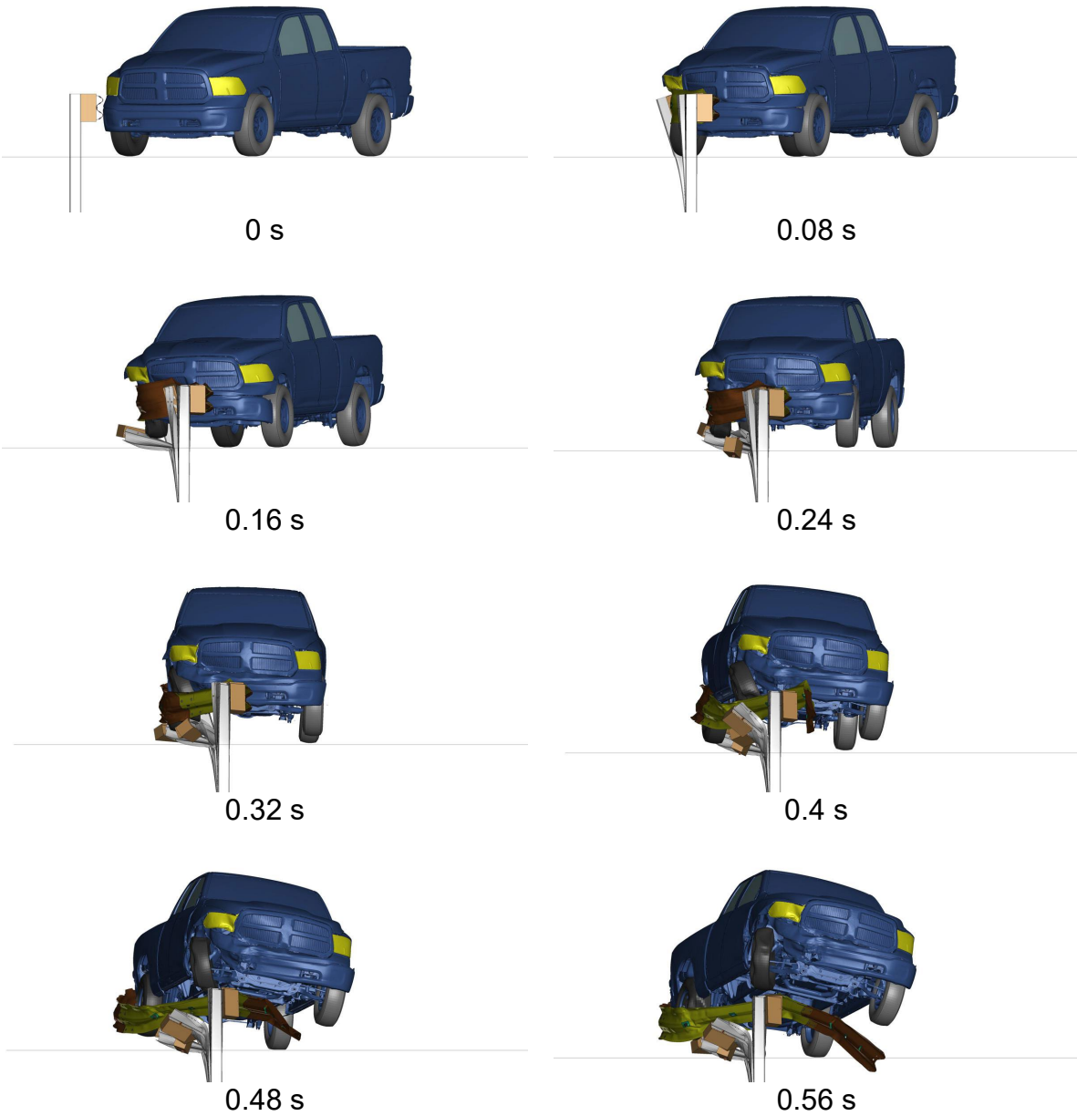
Figure 7.120. 75-ft Guardrail System with Refined Slot and Two End Washers – Downstream View of MASH Test 3-11
