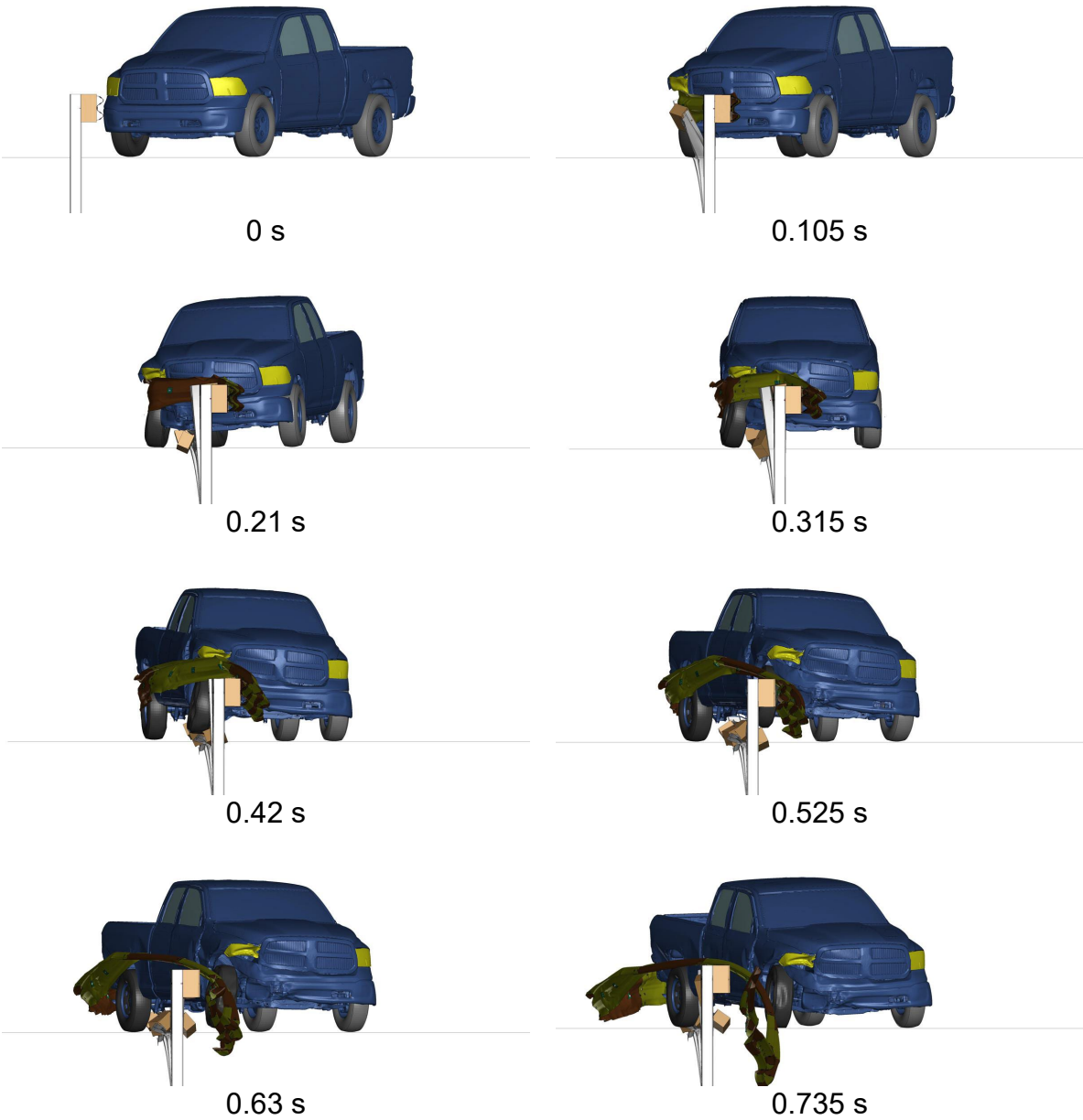
Figure 7.89. 250-ft Guardrail System with Refined Slot – Downstream View of MASH Test 3-11
