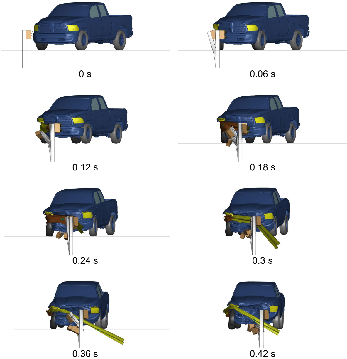
Figure 7.126. 62.5-ft Guardrail System with Refined Slot and Two End Washers – Downstream View of MASH Test 3-11
