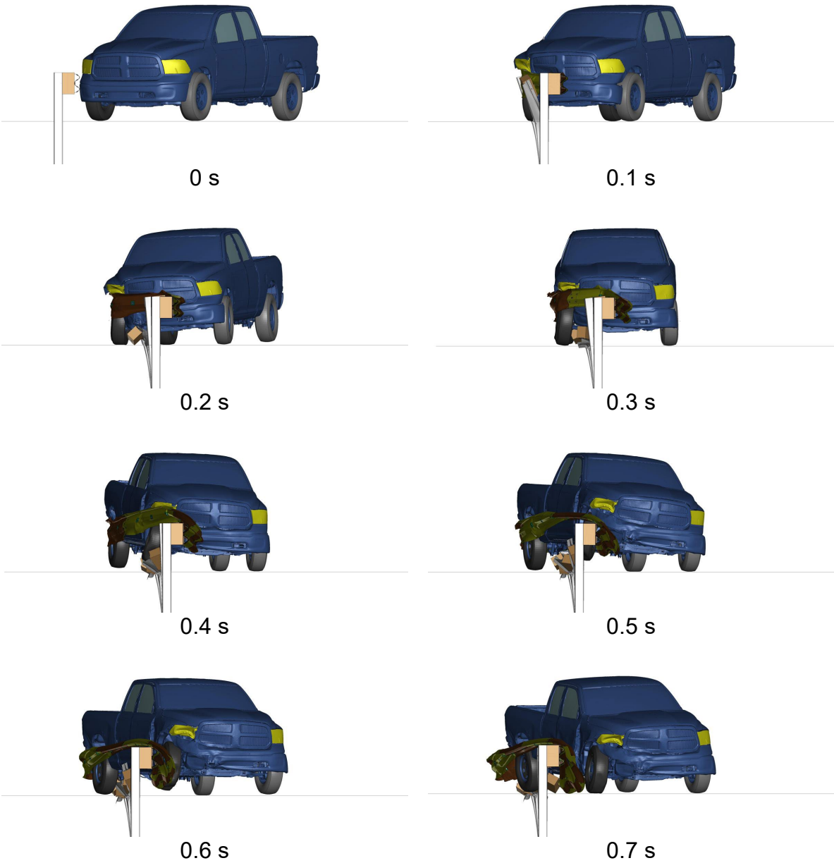
Figure 7.95. 262.5-ft Guardrail System with Refined Slot Mesh – Downstream View of MASH Test 3-11
