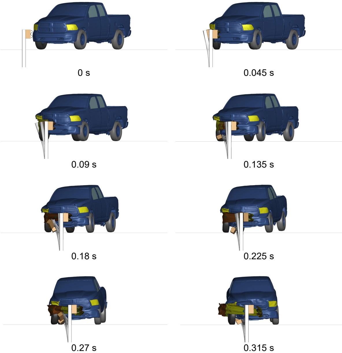
Figure 7.53. 175-ft Guardrail System with Refined Slot Mesh – Downstream View of MASH Test 3-11
