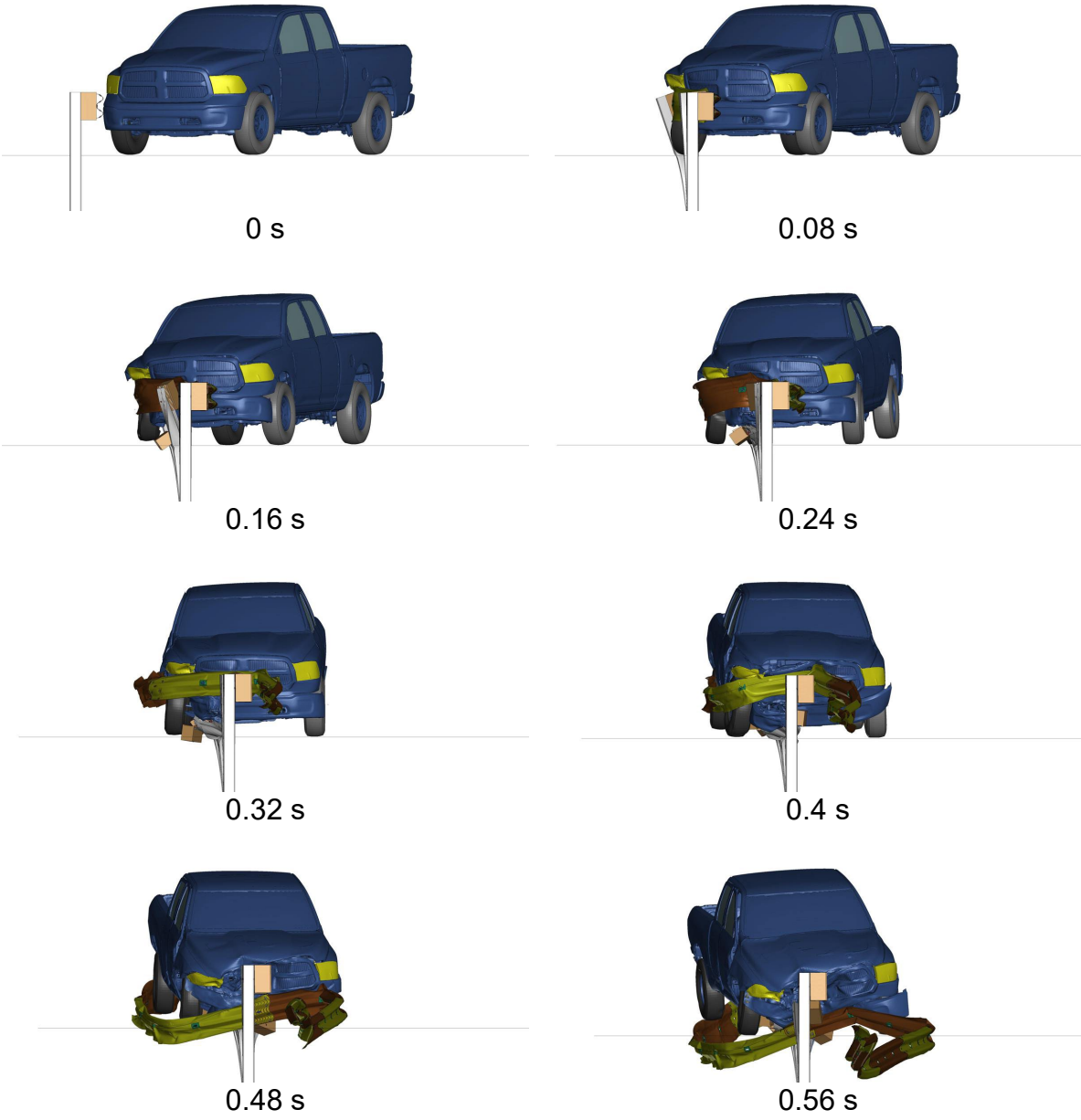
Figure 7.47. 162.5-ft Guardrail System with Refined Slot – Gut View of MASH Test 3-11
