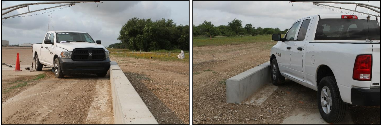
Figure 7.1 Permanent Low-Profile Barrier/Test Vehicle Geometrics for Test 616151-01-1.
