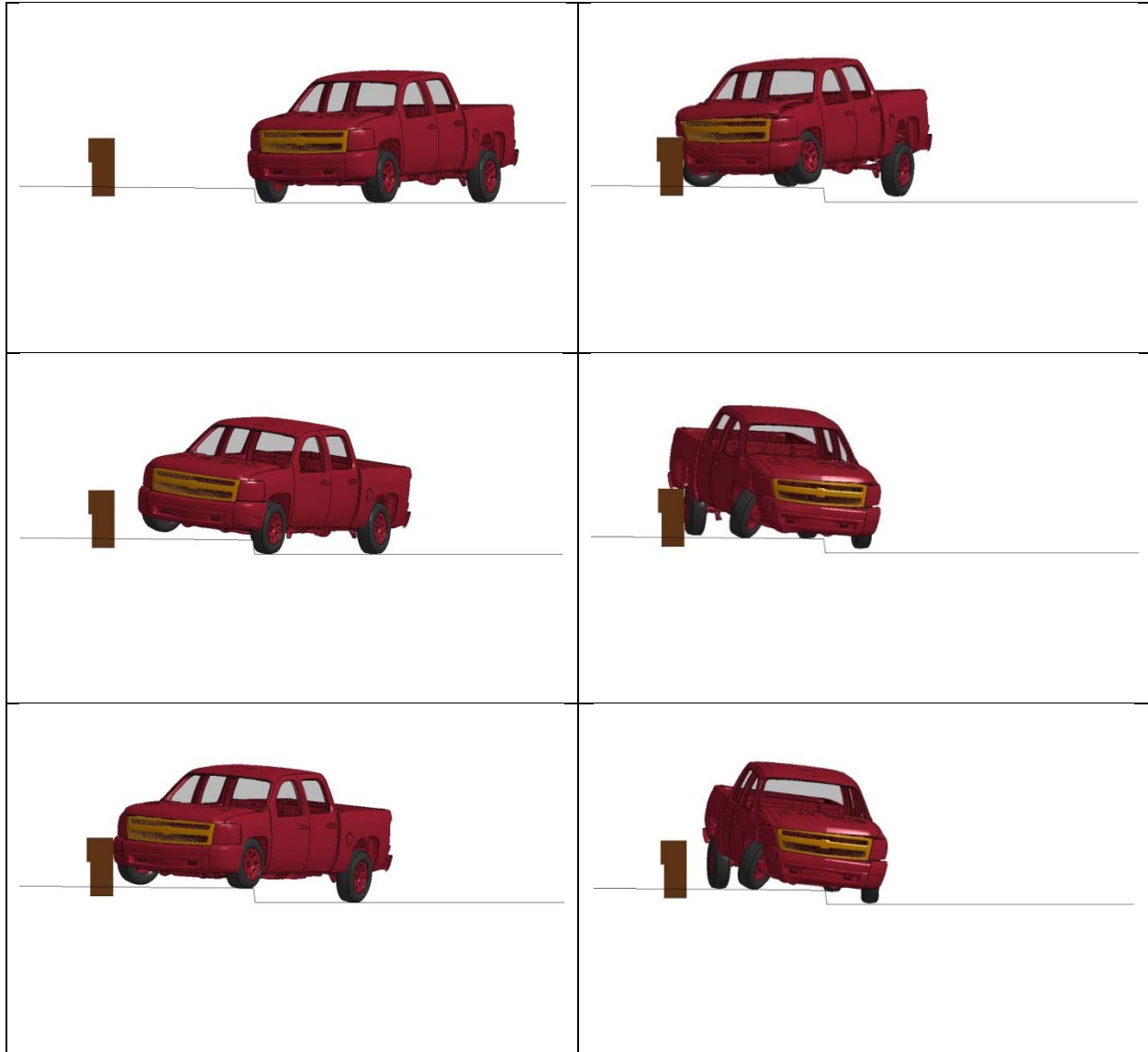
Figure 3-7 Pickup impact with 8-inch Curb, MnDOT parapet placed 80-inch inch from sidewalk edge (35 mph, 25 degrees)
