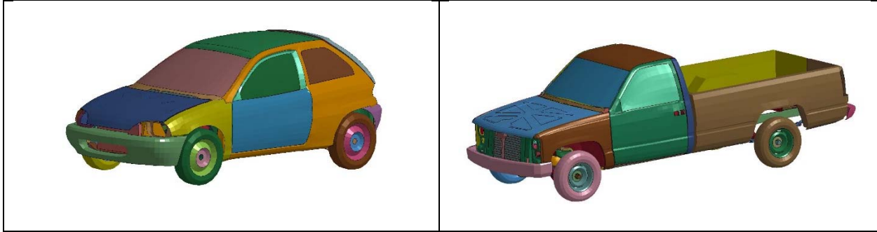
Figure 2-8 Finite Element Models of the Geo Metro and the Chevy C2500 ( NCHRP REPORT 350 Test Vehicles 820c and 2000P, Respectively)
