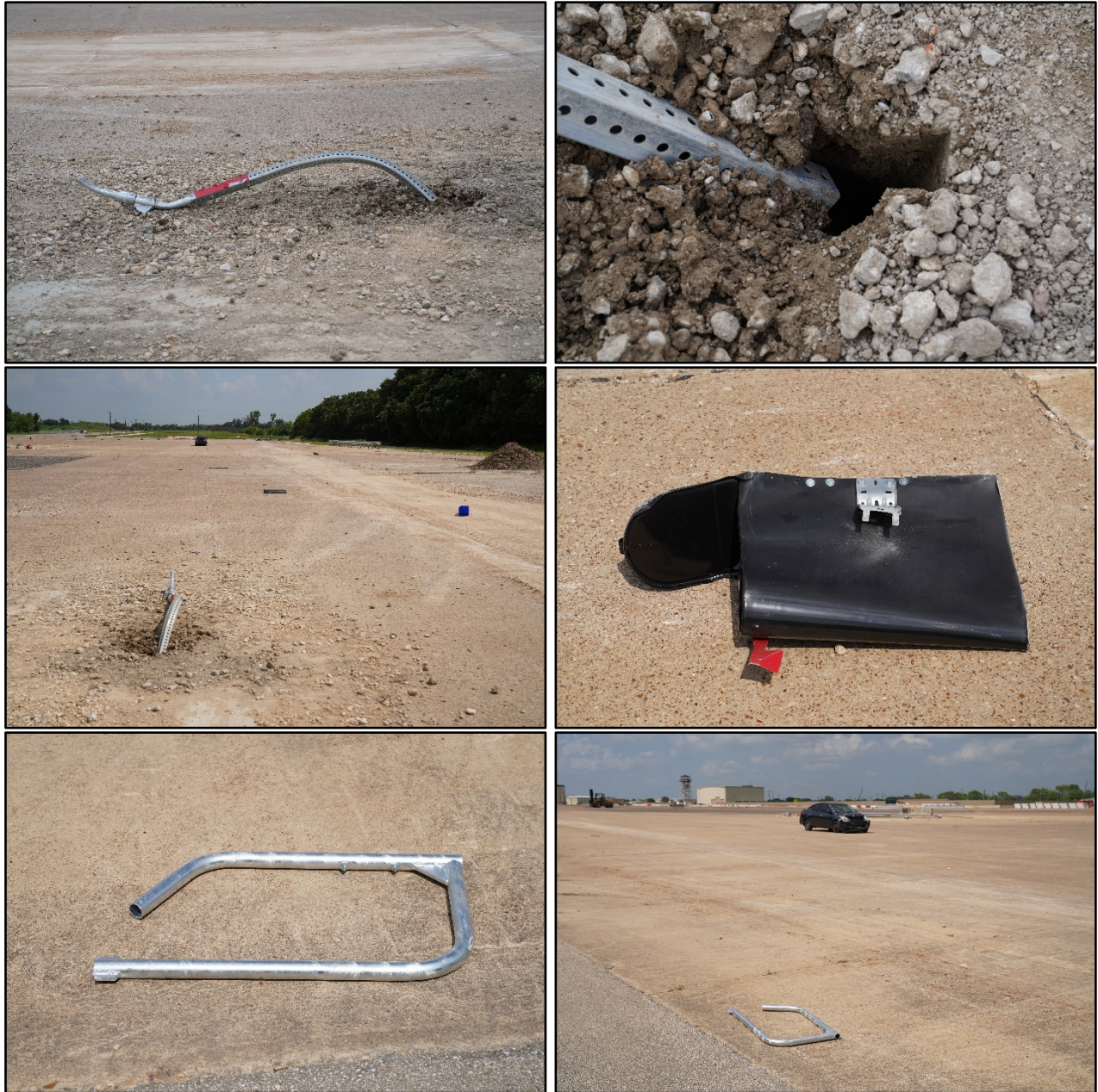
Figure 6.2. Mailbox after Test No. 609731-6.
