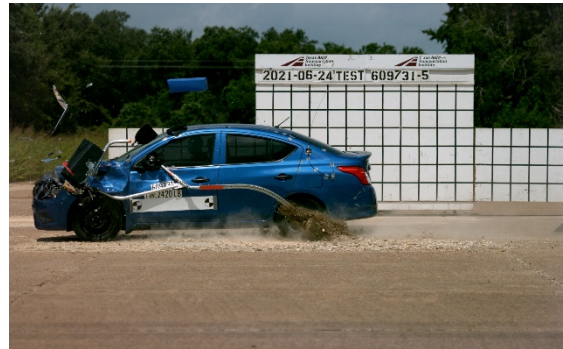
Figure C.1. Sequential Photographs for Test No. 609731-5 (Oblique and Perpendicular Views).
