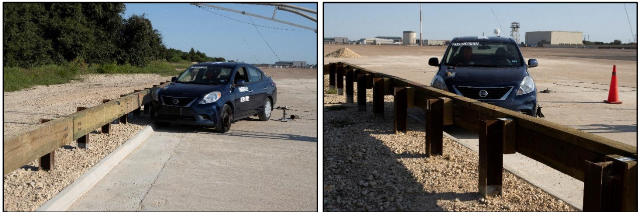
Figure 5.11. Modified Merritt Parkway Guiderail/Test Vehicle Geometrics for Test No. 612061-03-1.
