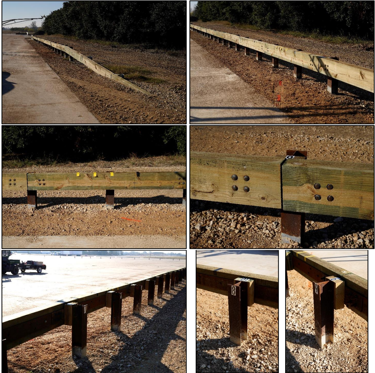
Figure 4.2. Merritt Parkway Guiderail with No Curb prior to Testing.
