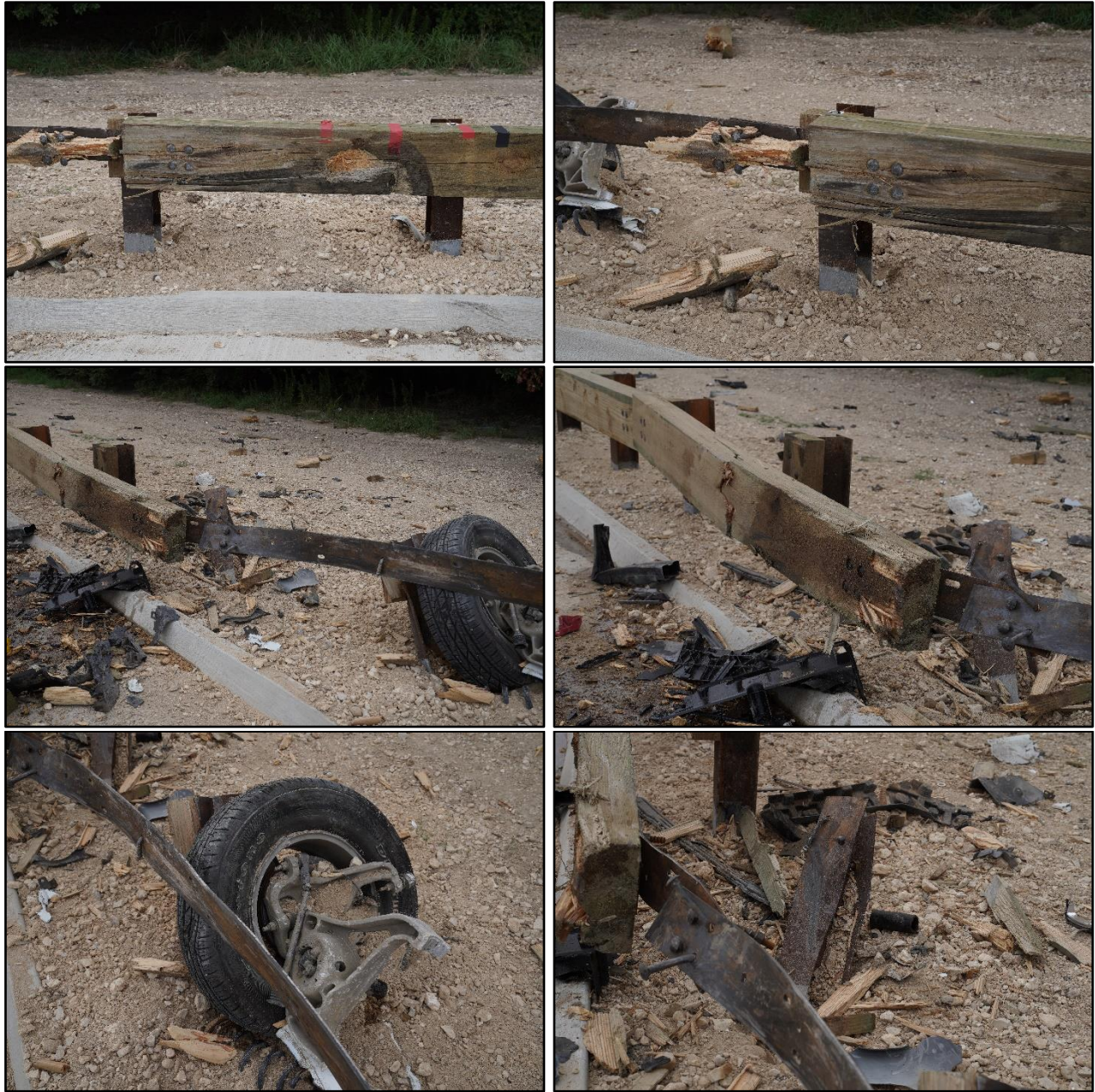
Figure 5.6. Damage at Posts 5 through 8 after Test No. 612061-02-1A.
