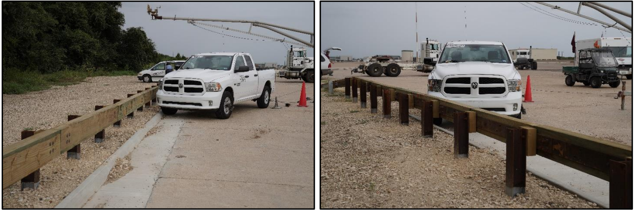
Figure 5.3. Modified Merritt Parkway Guiderail with No Curb/Test Vehicle Geometrics for Test No. 612061-02-1A.
