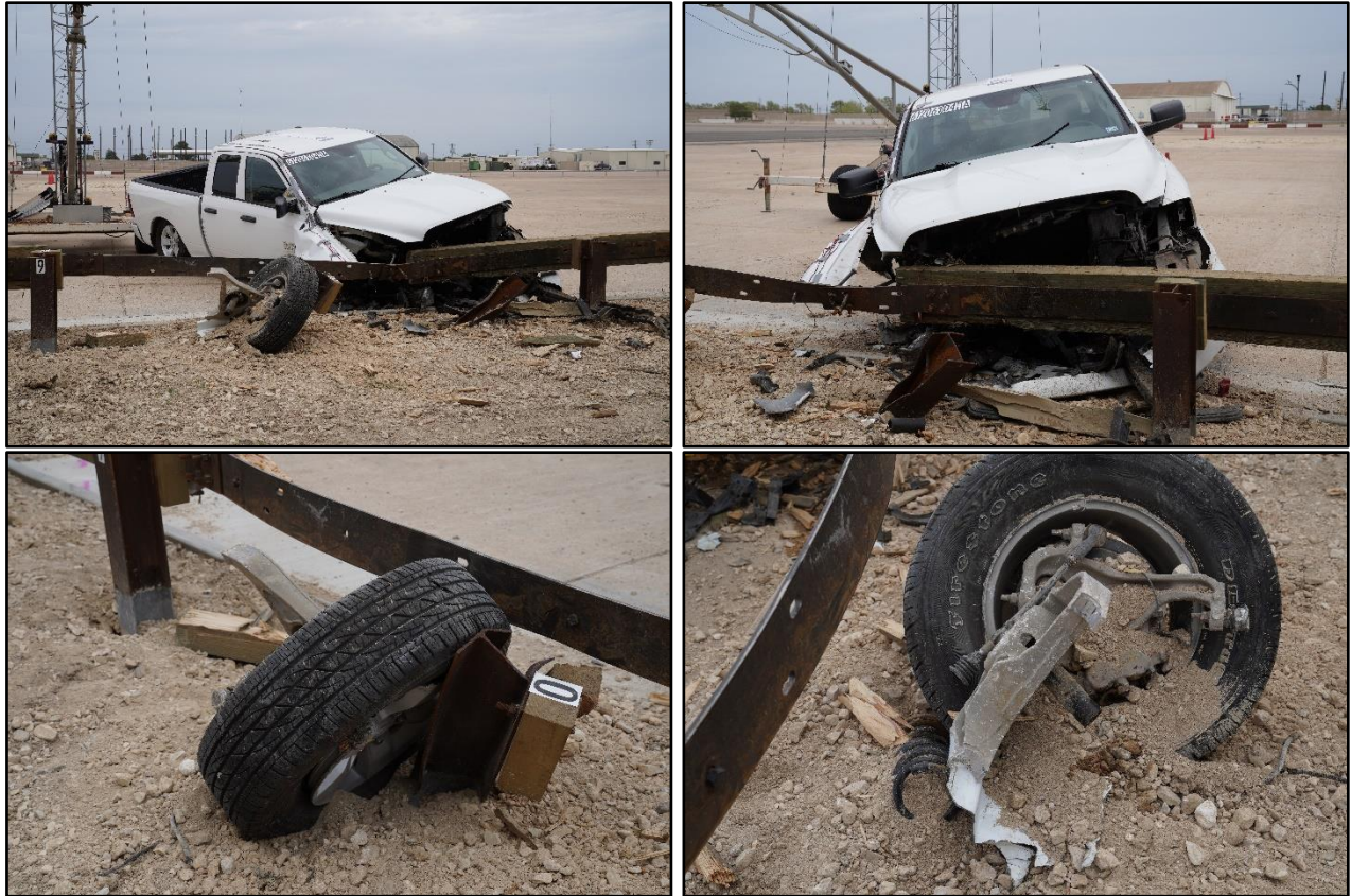
Figure 5.7. Field Side of Guiderail after Test No. 612061-02-1A.
