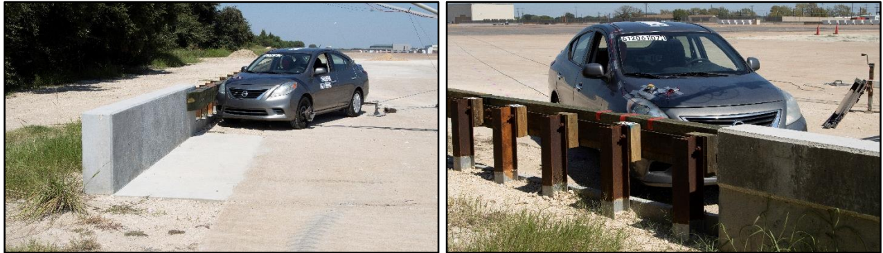
Figure 6.3. Transition/Test Vehicle Geometrics for Test No. 612061-07-1.
