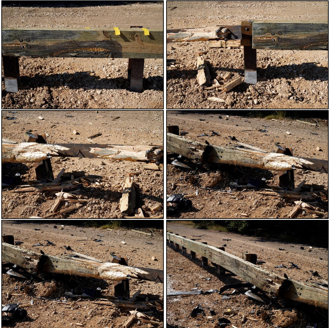
Figure 4.6. Damage at Posts 8 through 13 after Test No. 612061-02-1.
