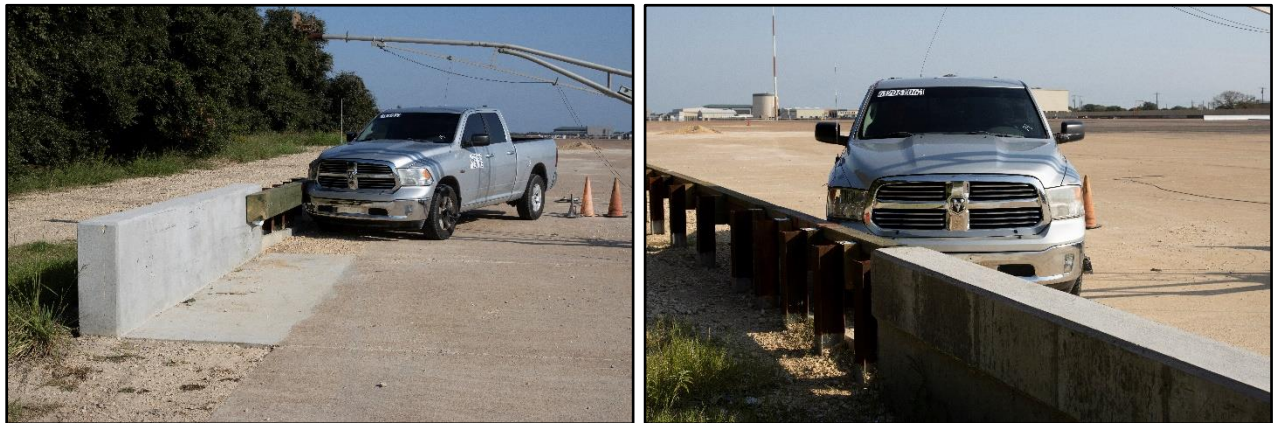
Figure 6.9. Transition/Test Vehicle Geometrics for Test No. 612061-06-1.
