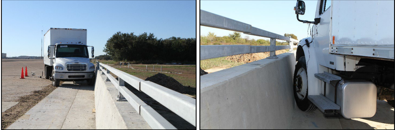
Figure 6.1 Bicycle Railing on a Constant Slope Parapet Test Vehicle Geometrics for Test 616221-01.
