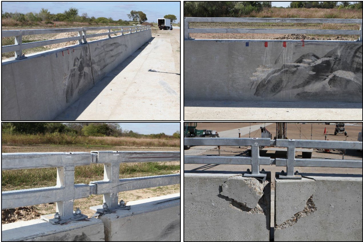
Figure 6.3 Bicycle Railing on a Constant Slope Parapet after Test 616221-01.
