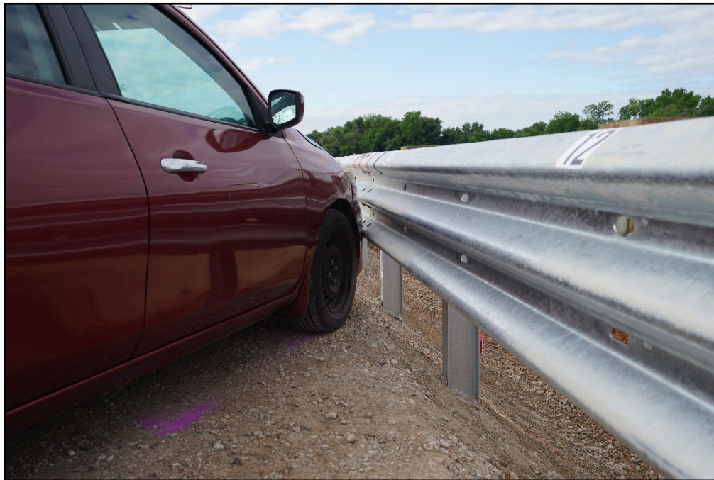
Figure 6.2. Guardrail System on 1:1 Slope/Test Vehicle Impact Location 617771-01-1.
