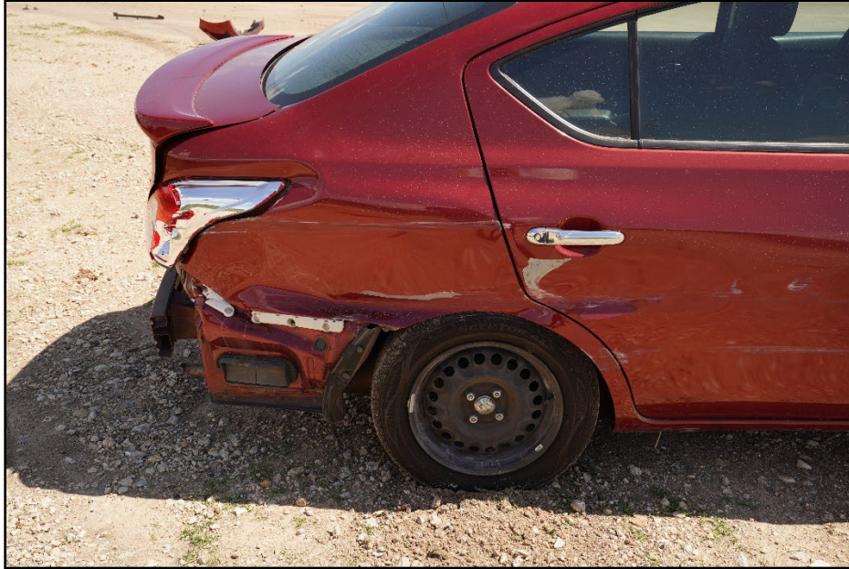
Figure 6.8. Opposite Rear Impact Side of Test Vehicle after Test 617771-01-1
