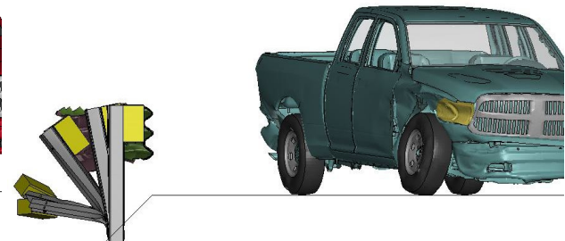
Figure 2.8. Sequential Images of Truck Simulations with 34-inch Thrie-beam Guardrail.
