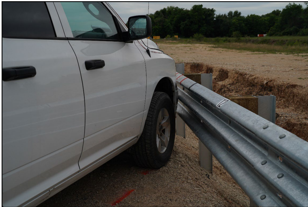
Figure 7.2. Guardrail System on 1:1 Slope/Test Vehicle Impact Location 617771-02-2.
