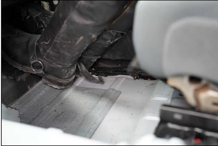
Figure 7.11. Interior of Test Vehicle on Impact Side after Test 617771-01-2.
