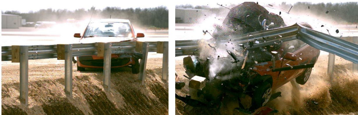
Figure 1.4. MASH 3-10 Test Resulted in Rupture of the W-Beam Rail Element (5).
