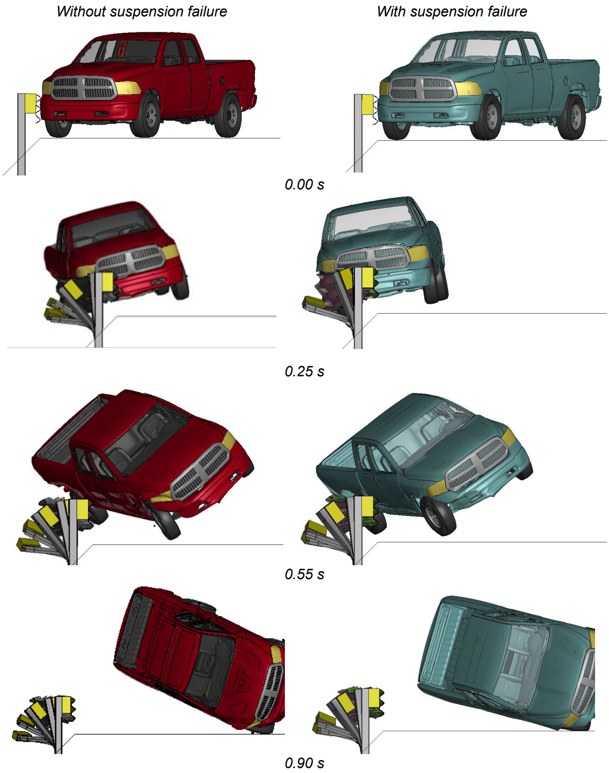
Figure 2.6 Sequential Images of Truck Simulation with 31-inch Thrie-beam Guardrail.
