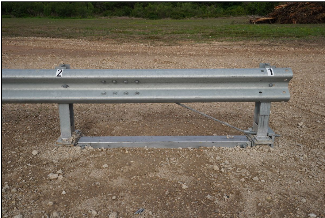
Figure 3.7. The Guardrail System on 1:1 Slope End Terminal Prior to Testing.
