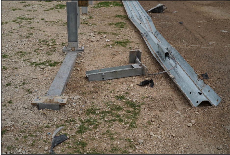
Figure 7.7. Guardrail System on 1:1 Slope at the Downstream Anchor after Test 617771-01-2.
