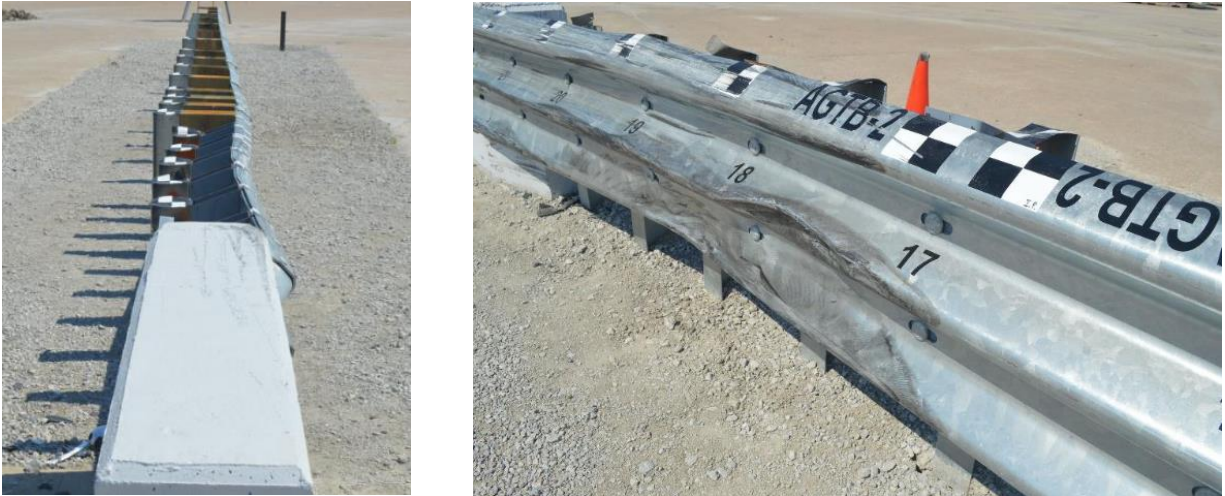
Figure 4. Transition Damage After Test 3-21 (Source: MwRSF Report TRP-03-369-20).
