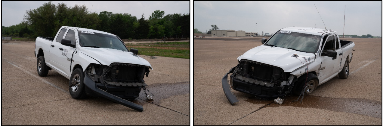
Figure 6.4. Test Vehicle after Test No. 610461-01-4.
