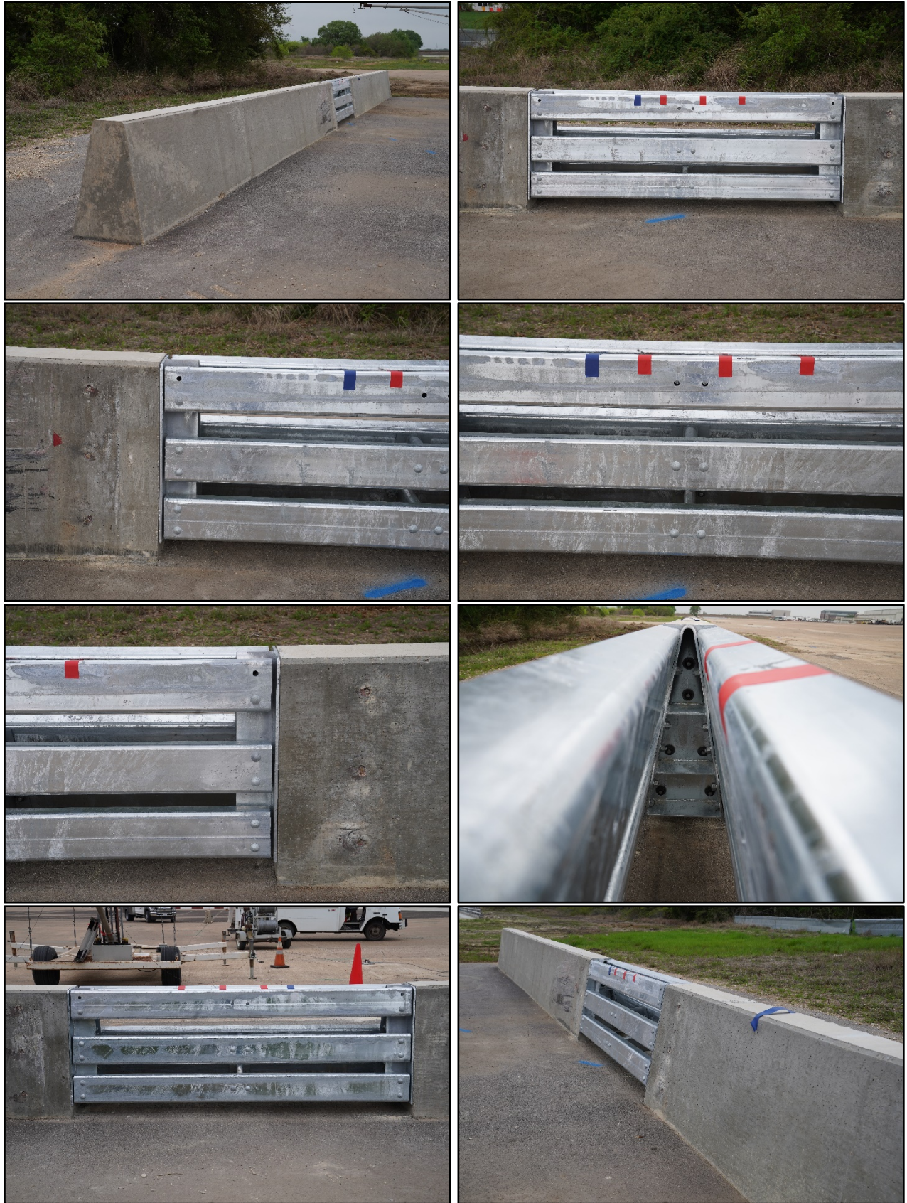
Figure 2.2. Redesigned Barrier Gap Rail prior to Testing.
