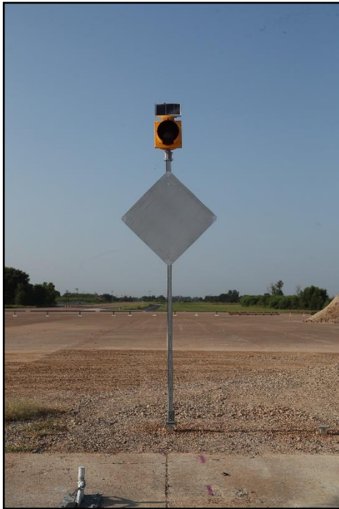
Figure 3.2. Breakaway Sign Support System with Flashing Equipment prior to Testing.
