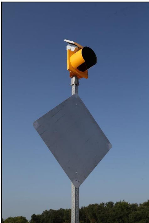
Figure 3.3. Close Up View of Sign Panel of Breakaway Sign Support System with Flashing Equipment prior to Testing.
