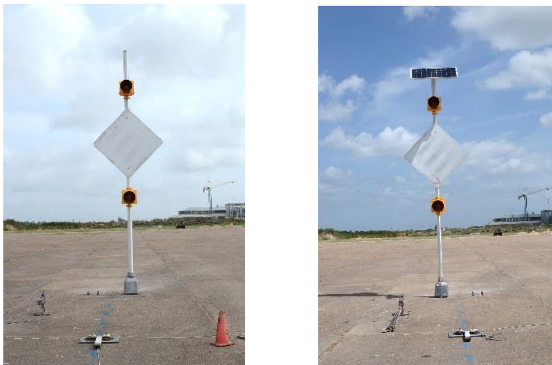
Figure 2.1. Flashing Beacon Assemblies without Solar Panel (left) and with Solar Panel (right). (2)
