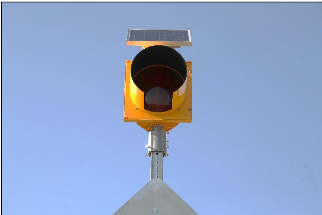
Figure 3.5. Close Up Parallel View of Flashing Beacon of Breakaway Sign Support System with Flashing Equipment prior to Testing.
