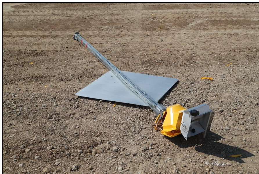
Figure 6.7. Breakaway Sign Support System with Flashing Equipment at Resting Location after Test 619541-01-1.
