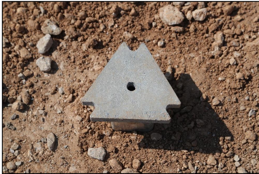
Figure 6.6. Breakaway Sign Support System with Flashing Equipment at Impact Location after Test 619541-01-1.
