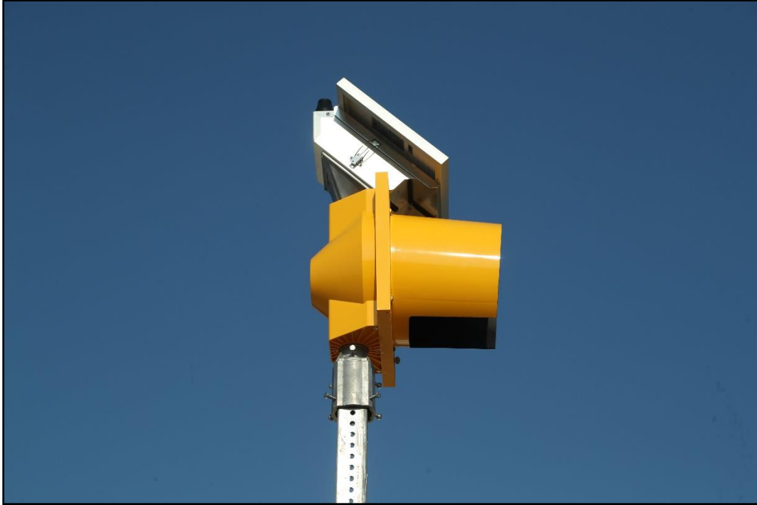
Figure 3.4. Close-Up Right-Angle View of Flashing Beacon of Breakaway Sign Support System with Flashing Equipment prior to Testing.
