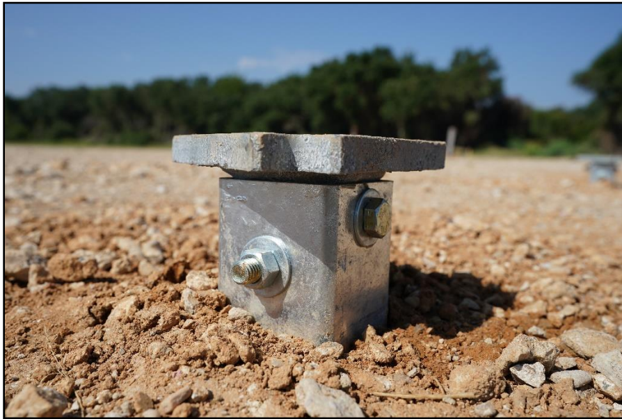
Figure 7.6. Breakaway Sign Support System with Flashing Equipment at Impact Location after Test 619541-01-2.
