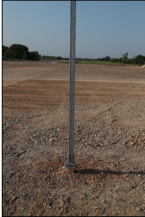
Figure 3.6. Breakaway Sign Support System with Flashing Equipment prior to Testing.
