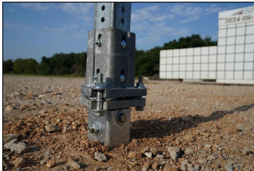
Figure 3.7. Breakaway Sign Support System with Flashing Equipment Perforated Steel Tubing prior to Testing.
