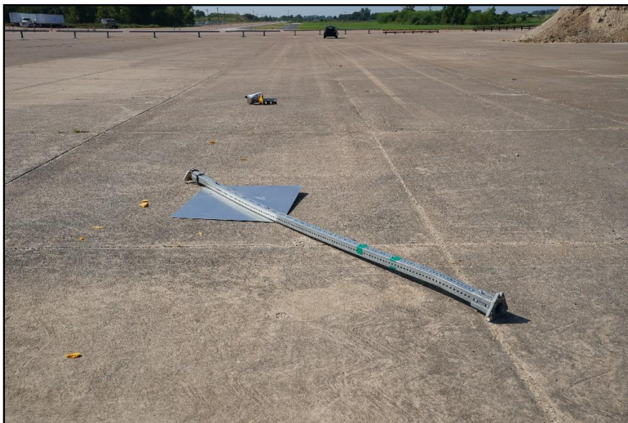
Figure 7.7. Breakaway Sign Support System with Flashing Equipment at Resting Location after Test 619541-01-2.
