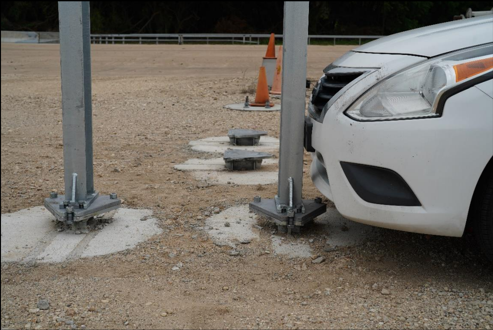
Figure 8-2. Route Marker Assembly Sign with Large Sign Supports /Test Vehicle Impact Location 616401-01-2.
