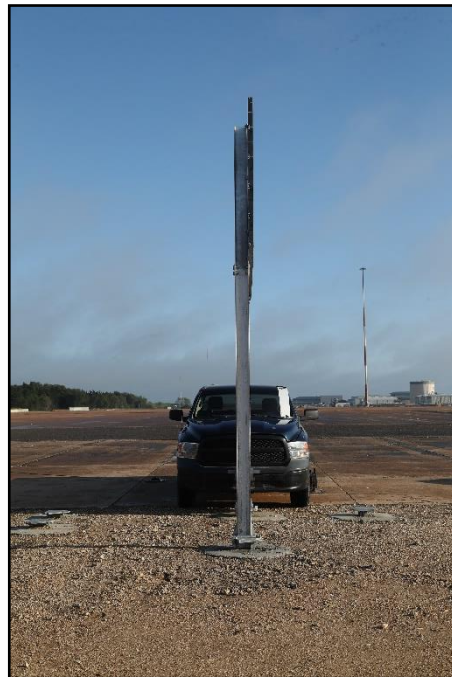
Figure 12-2. Guide Sign with Large Sign Supports /Test Vehicle Impact Location 616401-01-8.
