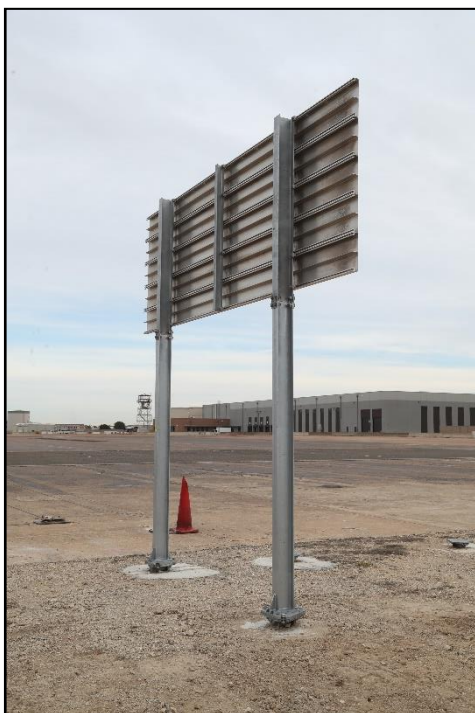
Figure 4-20. Back Side of the Guide Sign with Large Sign Supports prior to Test 616401-01-4.
