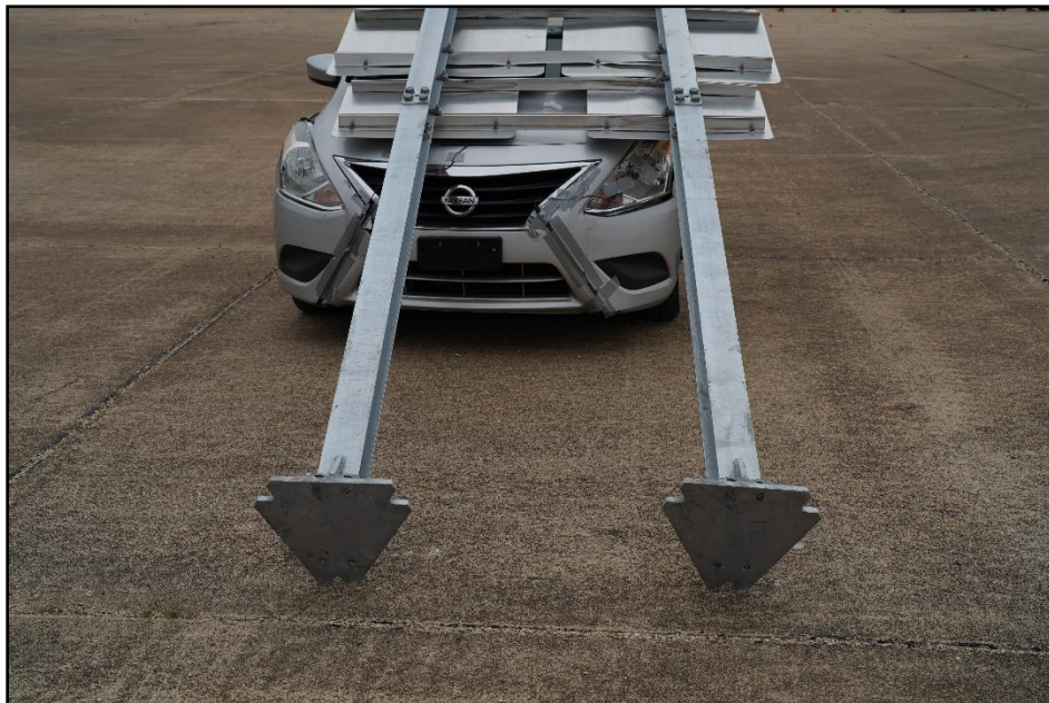
Figure 7-5. Route Marker Assembly Sign with Large Sign Supports after Test 616401-01-1.
