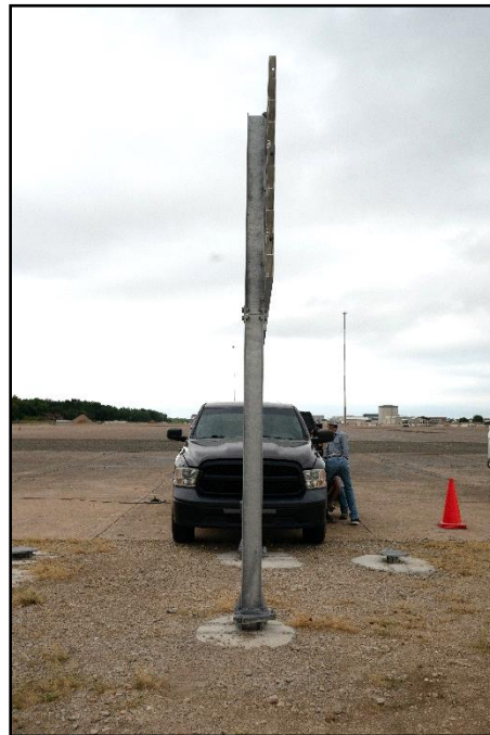
Figure 10-2. Guide Sign with Large Sign Supports /Test Vehicle Impact Location 616401-01-9.
