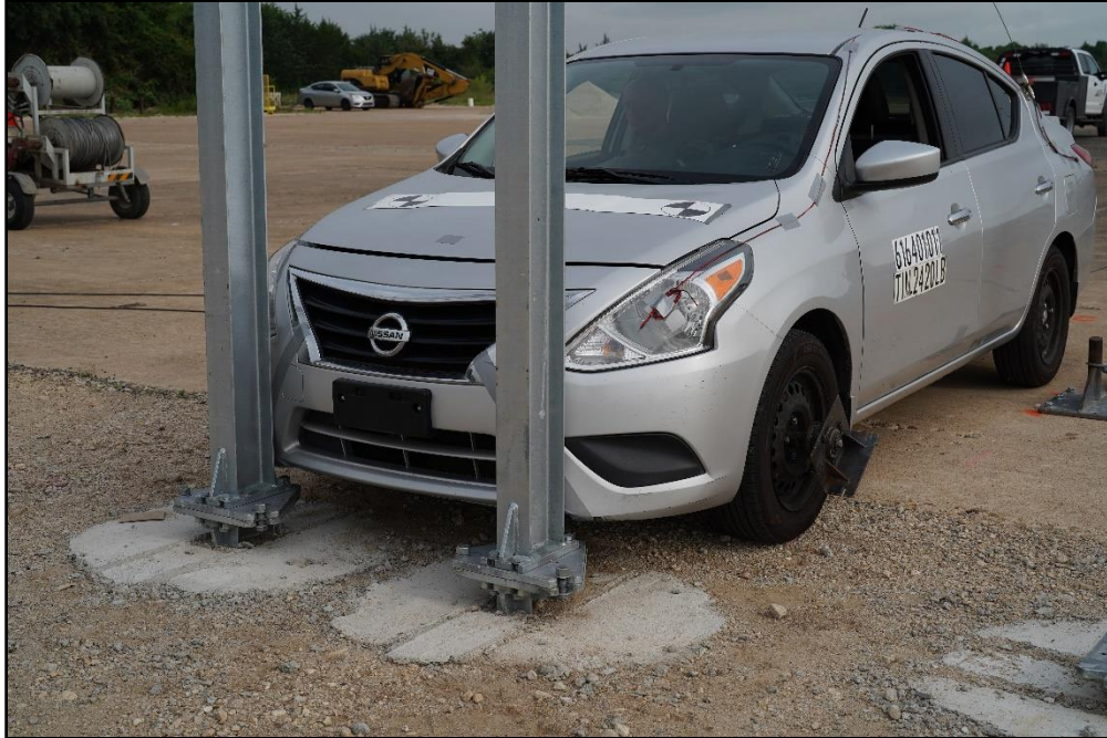
Figure 7-1. Route Marker Assembly Sign with Large Sign Supports /Test Vehicle Geometrics for Test 616401-01-1.
