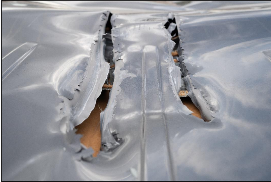
Figure 10-9. Detail of Roof Damage on the Test Vehicle after Test 616401-01-9.
