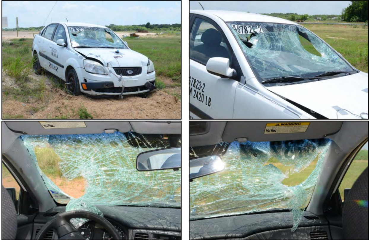
Figure 2-2. Direct Embedded Wood Support Temporary Guide Sign System 3-61 Test Vehicle Failure Damage (3)
