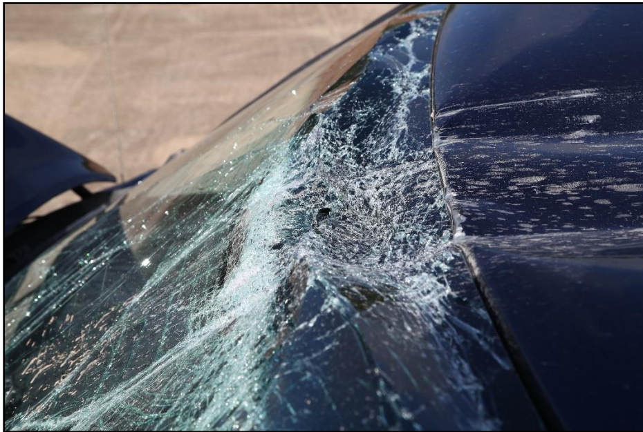
Figure 12-9. Test Vehicle Windshield Damage after Test 616401-01-8.
