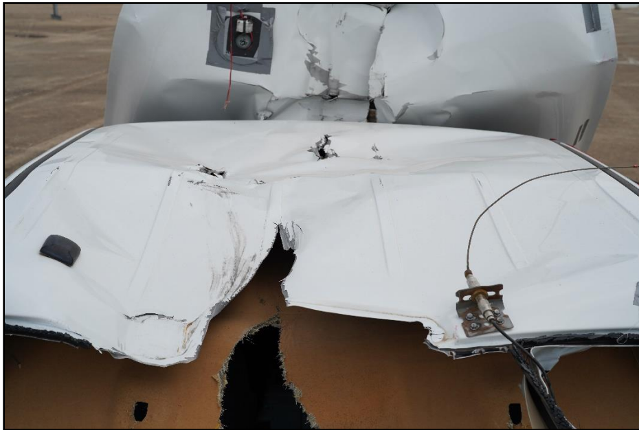
Figure 9-9. Roof of the Test Vehicle after Test 616401-01-3.
