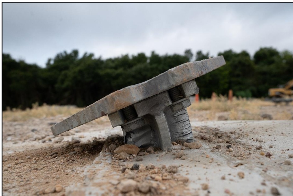
Figure 10-6. Footer for the Guide Sign with Large Sign after Test 616401-01-9.
