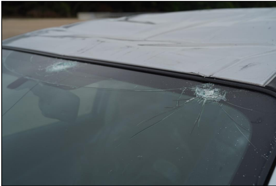
Figure 7-9. Test Vehicle Windshield Damage after Test 616401-01-1.
