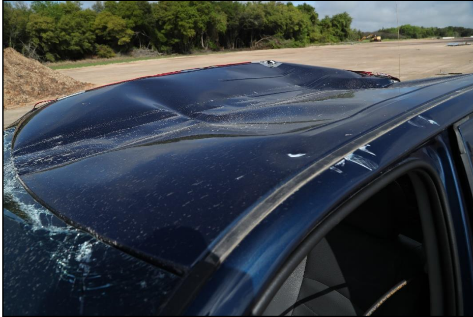
Figure 12-10. Roof of the Test Vehicle after Test 616401-01-8.
