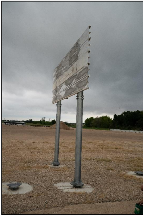
Figure 4-14. Impact Side of the Guide Sign with Large Sign Supports prior to Test 616401-01-9.
