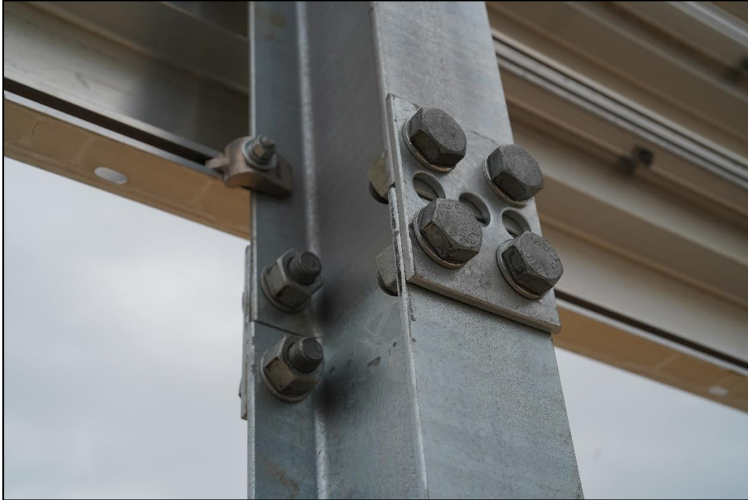
Figure 4-11. Fuse plate on the Guide Sign with Large Sign Supports prior to Test 616401-01-3.
