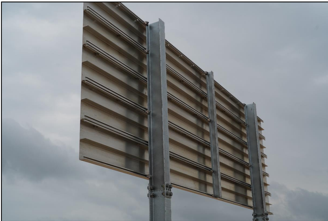
Figure 4-10. Back Side of the Guide Sign with Large Sign prior to Test 616401-01-3.
