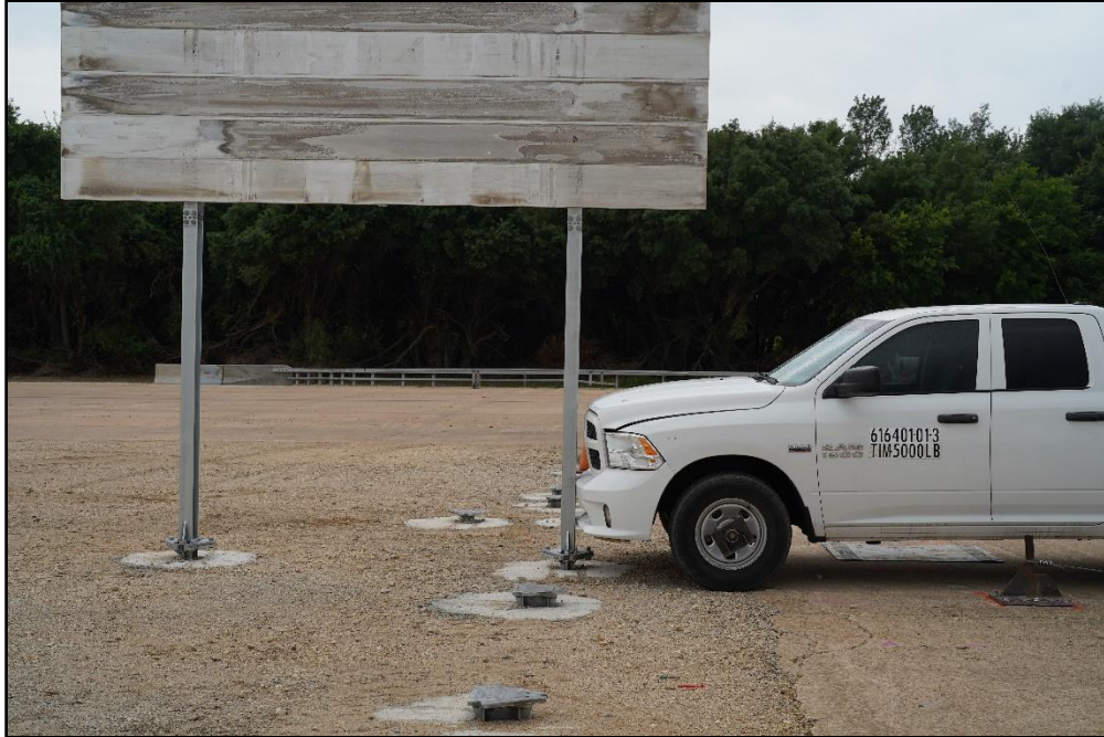
Figure 9-1. Guide Sign with Large Sign Supports /Test Vehicle Geometrics for Test 616401-01-3.
