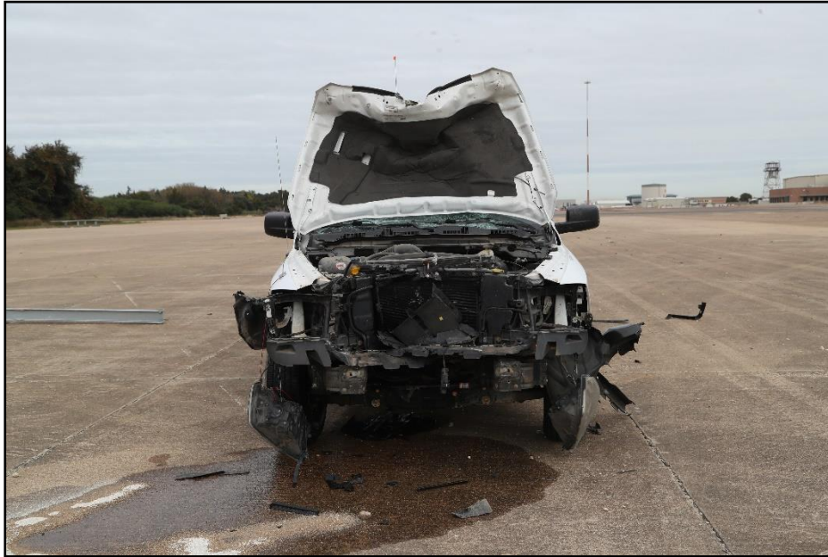
Figure 11-7. Impact Side of Test Vehicle after Test 616401-01-4.
