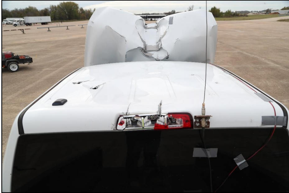
Figure 11-9. Roof of the Test Vehicle after Test 616401-01-4.
