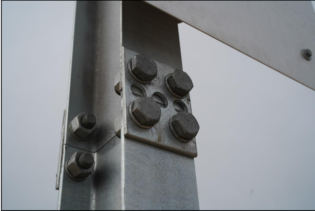
Figure 4-6. Fuse plate on the Route Marker Assembly with Large Sign Supports prior to Testing.
