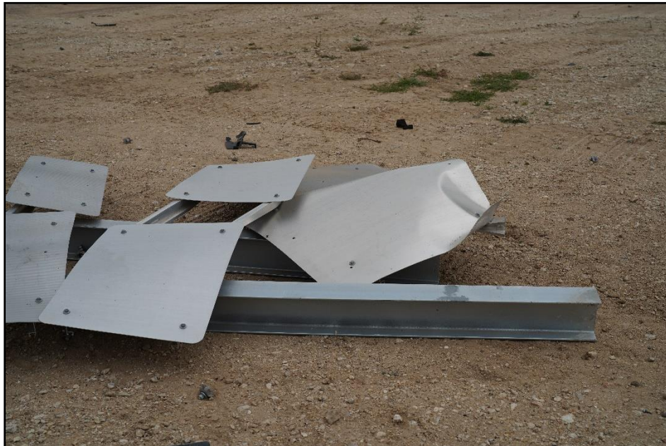
Figure 8-5. Route Marker Assembly Sign with Large Sign Supports after Test 616401-01-2.
