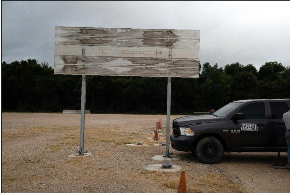
Figure 10-1. Guide Sign with Large Sign Supports /Test Vehicle Geometrics for Test 616401-01-9.
