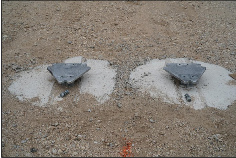
Figure 7-6. Footers for the Route Marker Assembly Sign with Large Sign Supports after Test 616401-01-1.
