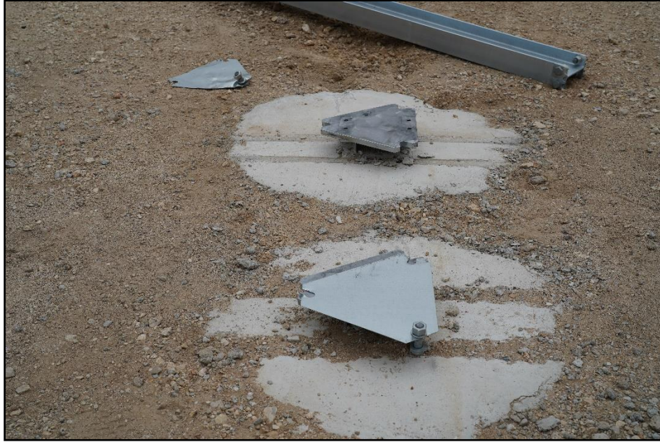
Figure 8-6. Footers for the Route Marker Assembly Sign with Large Sign Supports after Test 616401-01-2.
