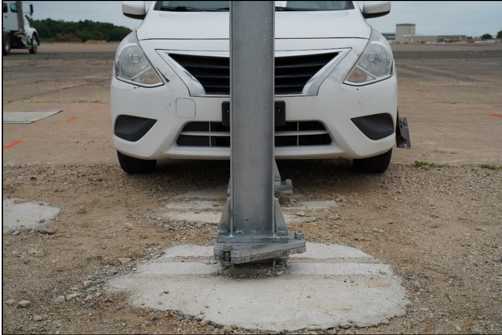
Figure 8-1. Route Marker Assembly Sign with Large Sign Supports /Test Vehicle Geometrics for Test 616401-01-2.
