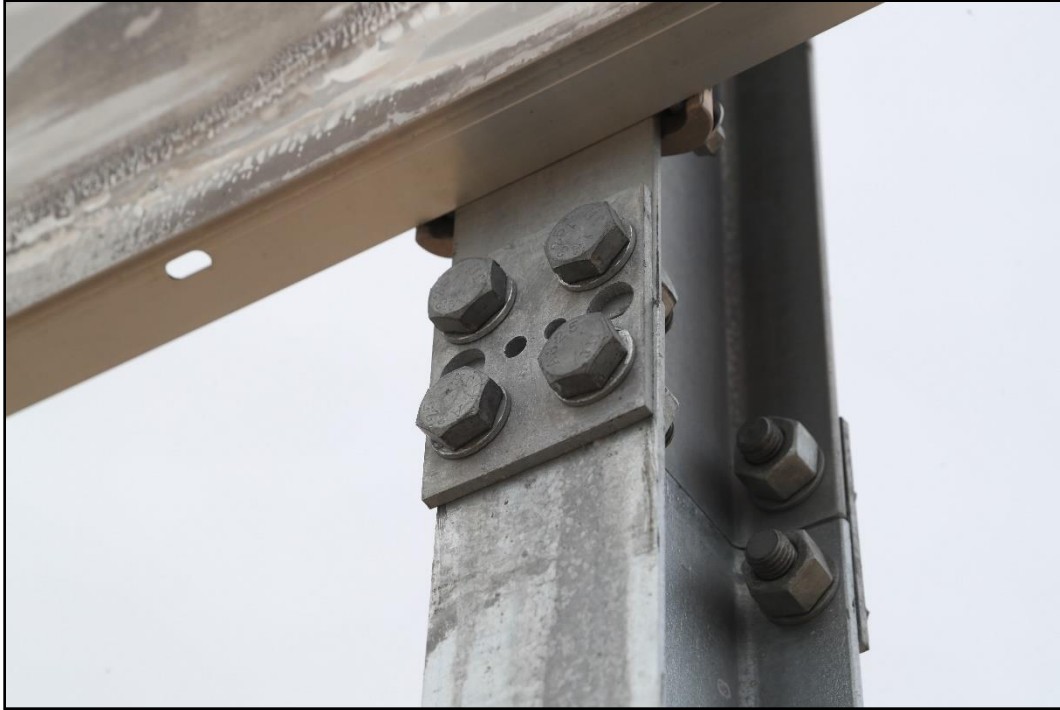
Figure 4-21. Fuse plate on the Guide Sign with Large Sign Supports prior to Test 616401-01-4.
