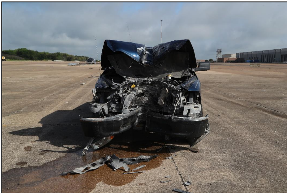
Figure 12-7. Impact Side of Test Vehicle after Test 616401-01-8.
