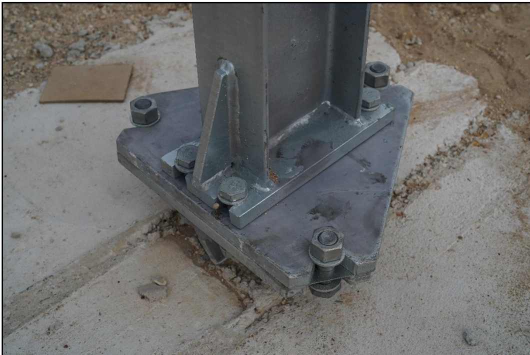
Figure 4-7. Slip Base on the Route Marker Assembly with Large Sign Supports prior to Testing.
