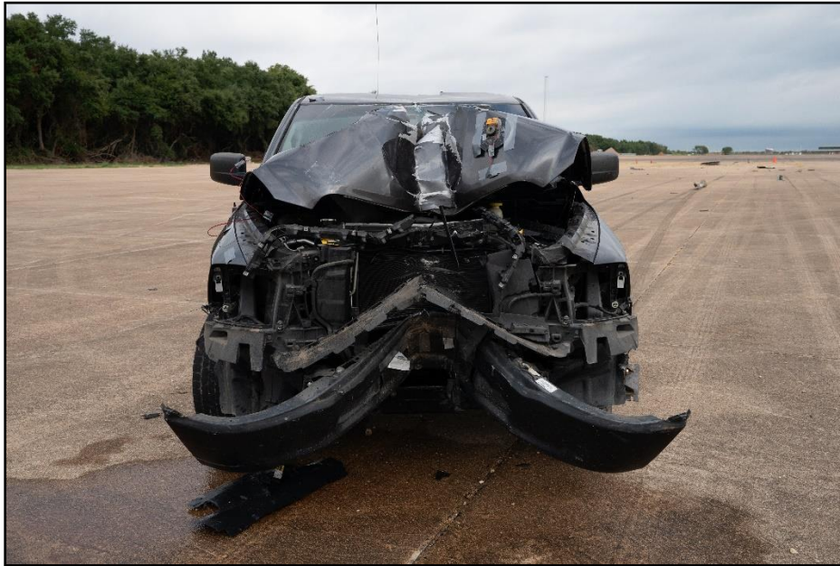
Figure 10-7. Impact Side of Test Vehicle after Test 616401-01-9.
