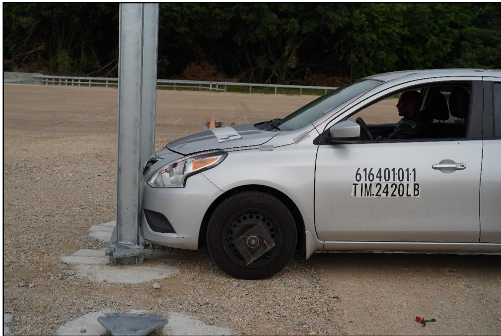
Figure 7-2. Route Marker Assembly Sign with Large Sign Supports /Test Vehicle Impact Location 616401-01-1.
