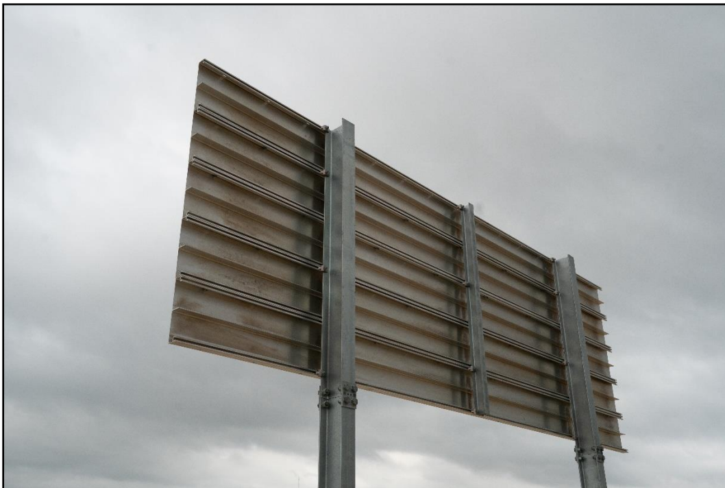
Figure 4-15. Back Side of the Guide Sign with Large Sign Supports prior to Test 616401-01-9.
