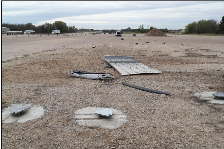
Figure 11-5. Guide Sign with Large Sign Supports at Impact Location after Test 616401-01-4.
