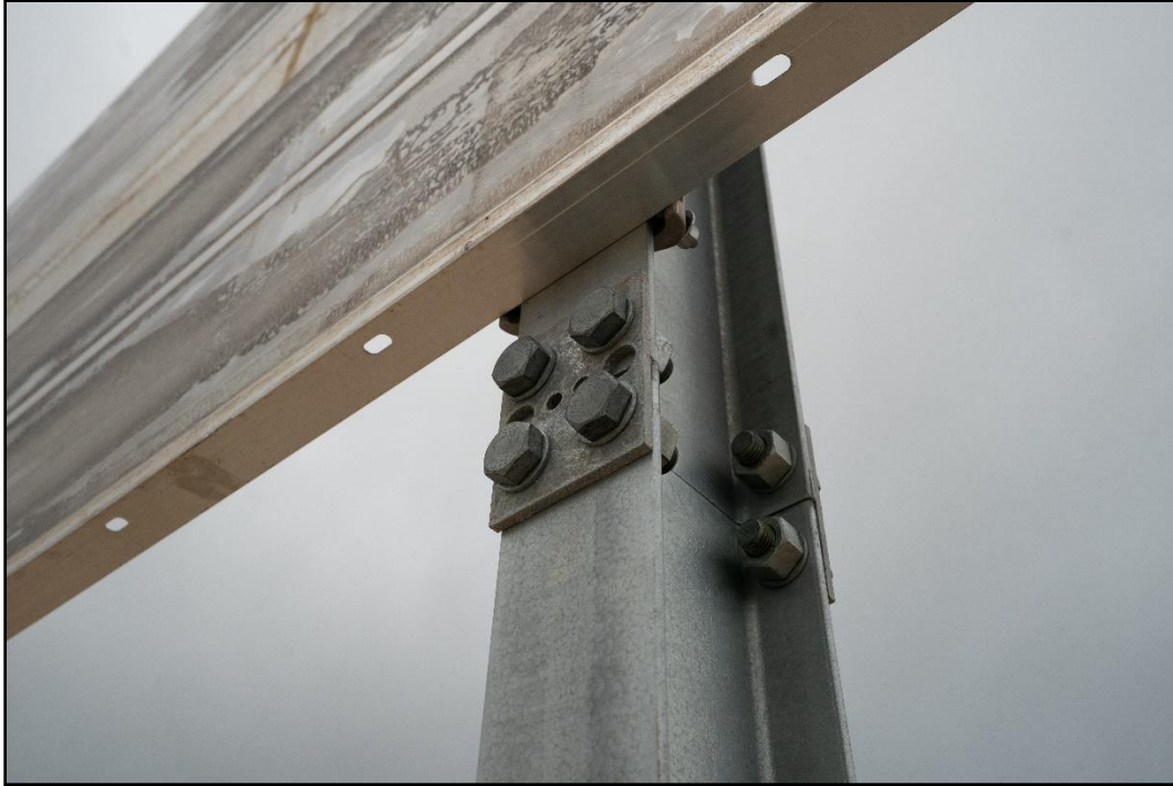
Figure 4-16. Fuse plate on the Guide Sign with Large Sign Supports prior to Test 616401-01-9.
