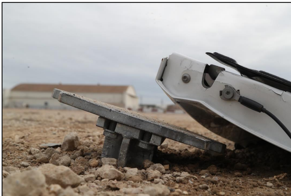
Figure 11-6. Downstream Footer for the Guide Sign with Large Sign Supports after Test 616401-01-4.
