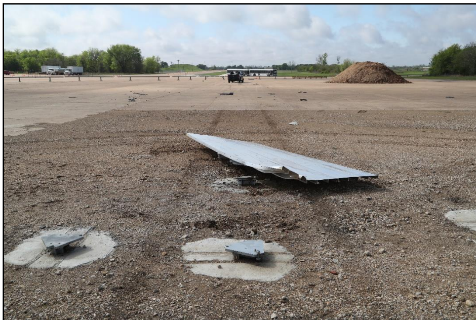
Figure 12-5. Guide Sign with Large Sign Supports at Impact Location after Test 616401-01-8.
