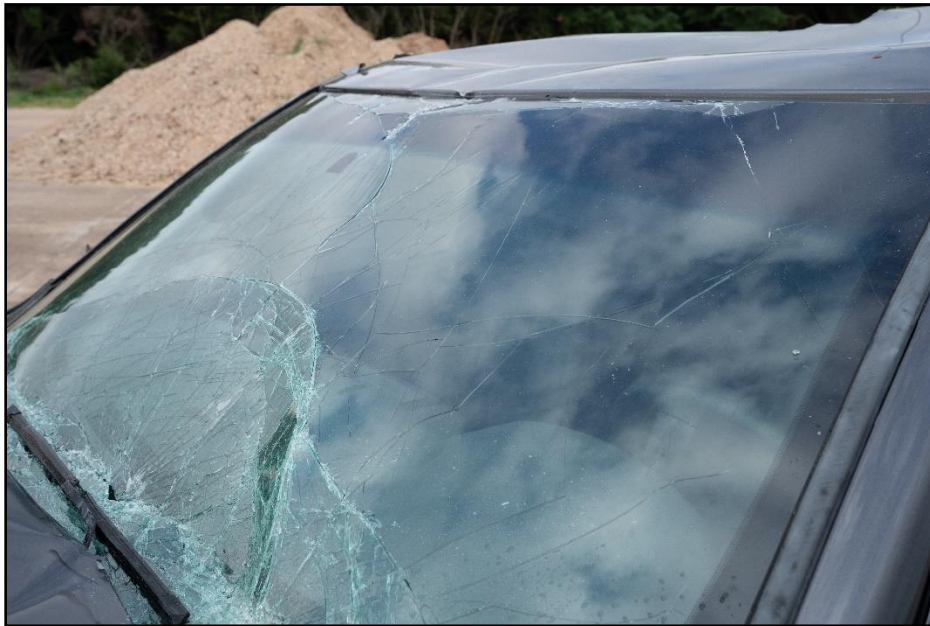
Figure 10-10. Test Vehicle Windshield Damage after Test 616401-01-9.
