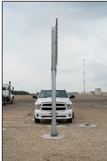
Figure 9-2. Guide Sign with Large Sign Supports /Test Vehicle Impact Location 616401-01-3.
