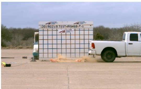
Figure 2.88. Skid-Mounted Single-Post Perforated Steel Tube Temporary Sign Support Test 3-72, 0-degree Impact Sequential Photos (Continued) (4)
