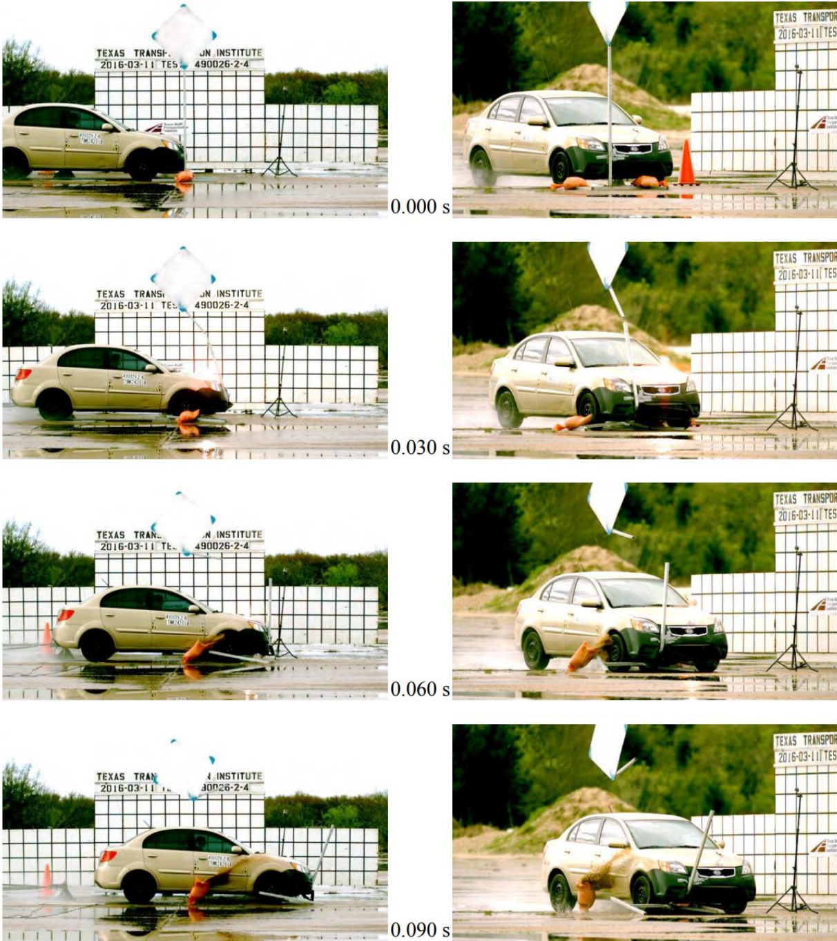
Figure 2.17. Temporary High-Mounting Sign Support, Option B Test 3-71, 90-degree Impact Sequential Photos (2)
