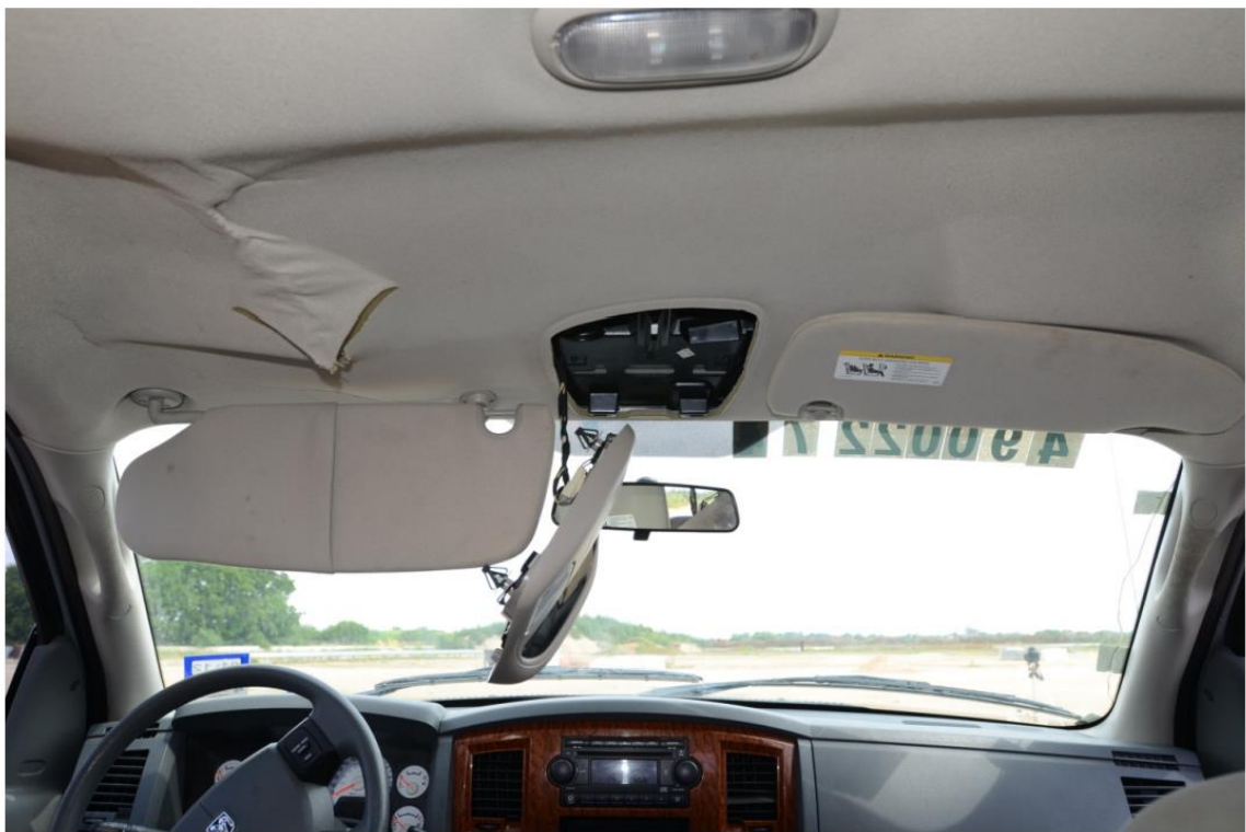
Figure 2.67. High-Mounting-Height Temporary Single Sign Support, Modified Design 2 Test 3-72 Vehicle Interior Damage (3)
