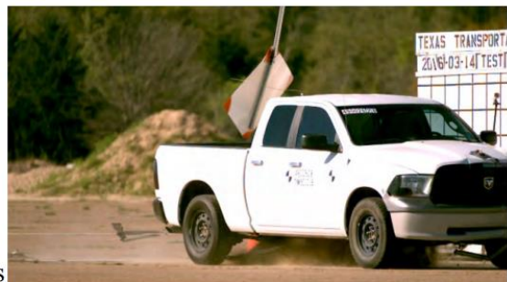
Figure 2.26. Temporary High-Mounting Sign Support, Option B Test 3-72, 0-degree Impact Sequential Photos (Continued) (2)
