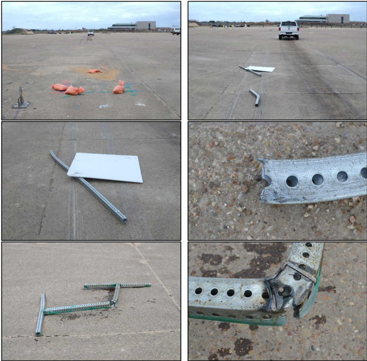
Figure 2.94. Skid-Mounted Single-Post Perforated Steel Tube Temporary Sign Support Test 3-72, 90-degree Impact System Damage (4)
