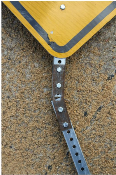
Figure 2.82. High-Mounting-Height Temporary Single Sign Support, Modified Design 8 Test 3-71, 90-degree Impact System Damage (3)
