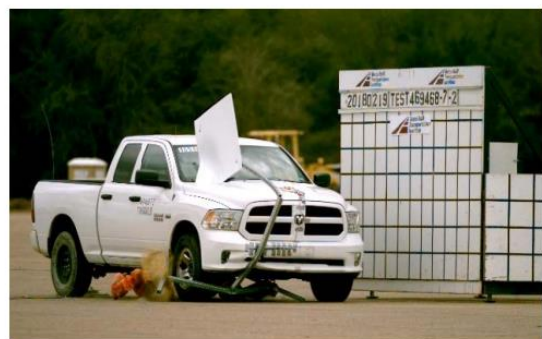
Figure 2.92. Skid-Mounted Single-Post Perforated Steel Tube Temporary Sign Support Test 3-72, 90-degree Impact Sequential Photos (4)
