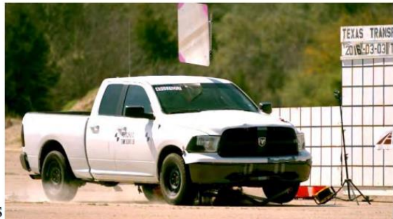
Figure 2.13. Temporary High-Mounting Sign Support, Option B Test 3-72, 90-degree Impact Sequential Photos (2)
