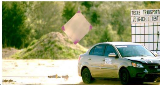
Figure 2.45. Temporary High-Mounting Sign Support, Option C Test 3-71, 0-degree Impact Sequential Photos (Continued) (2)
