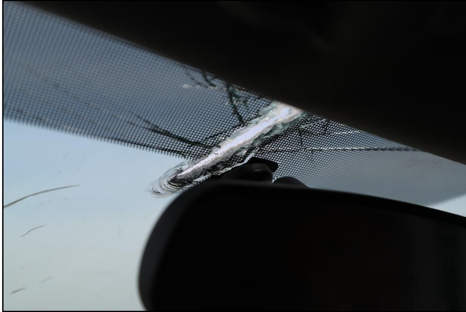
Figure 12.10. Interior of Test Vehicle at the Windshield Damage after Test 618901-01-2-7.
