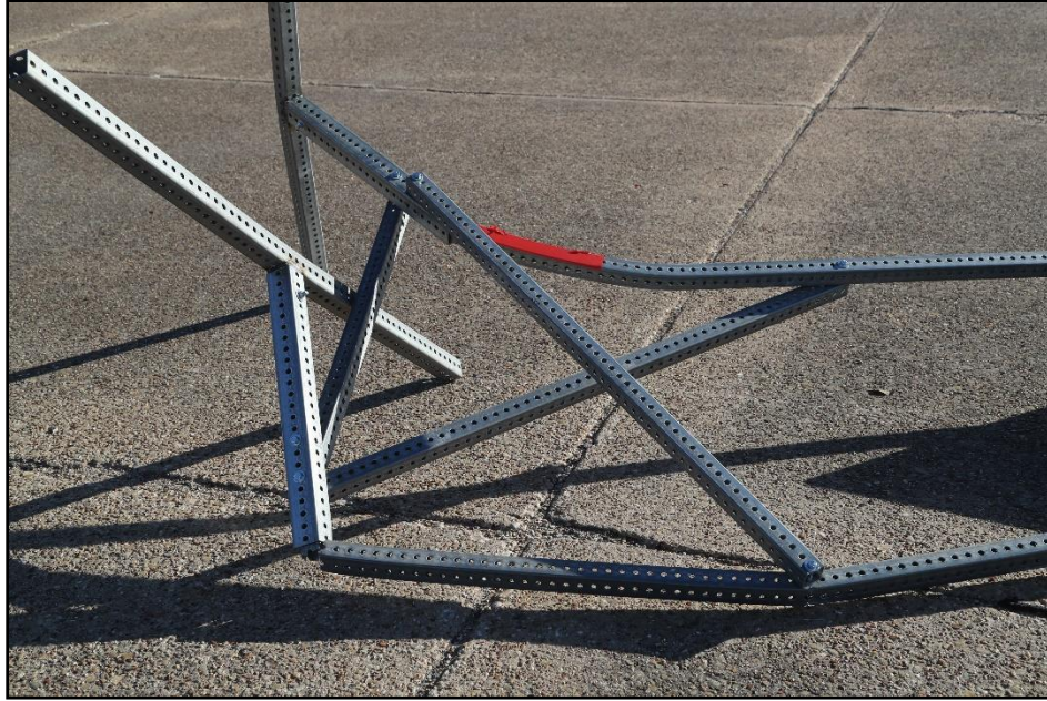
Figure 9.6. Lower Half of the Tall Sign Supports for Aluminum Signs at Resting Position after Test 618901-01-2-4.
