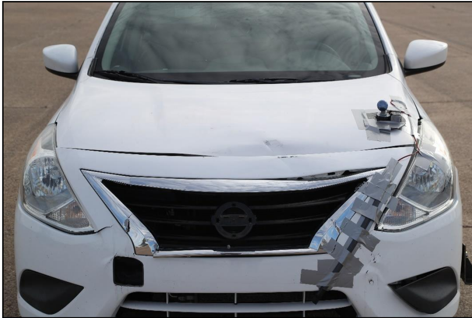
Figure 7.7. Impact Side of Test Vehicle after Test 618901-01-2-2.
