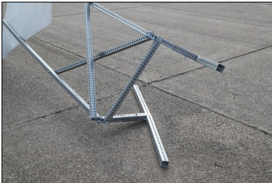
Figure 7.6. Lower Half of the Tall Sign Supports for Aluminum Signs at Resting Position after Test 618901-01-2-2.
