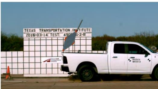
Figure 2.26. Temporary High-Mounting Sign Support, Option B Test 3-72, 0-degree Impact Sequential Photos (Continued) (2)
