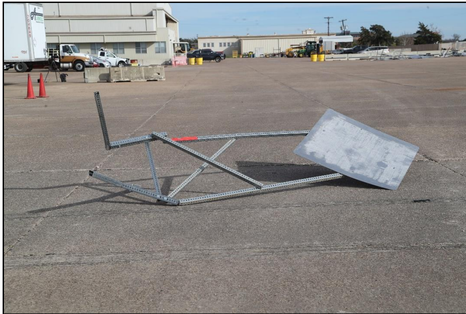
Figure 11.5. Tall Sign Supports for Aluminum Signs at Resting Position after Test 618901-01-2-6.
