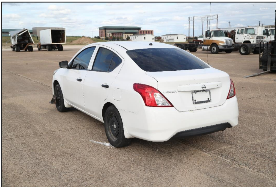
Figure 7.8. Rear Impact Side of Test Vehicle after Test 618901-01-2-2.
