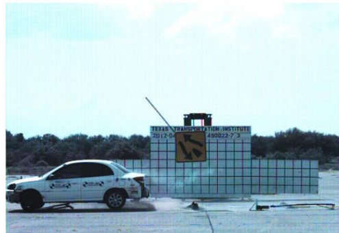
Figure 2.81. High-Mounting-Height Temporary Single Sign Support, Modified Design 8 Test 3-71, 90-degree Impact Sequential Photos (3)
