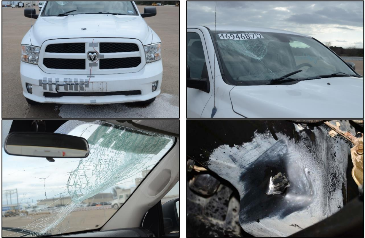
Figure 2.95. Skid-Mounted Single-Post Perforated Steel Tube Temporary Sign Support Test 3-72, 90-degree Impact Vehicle Damage (4)
