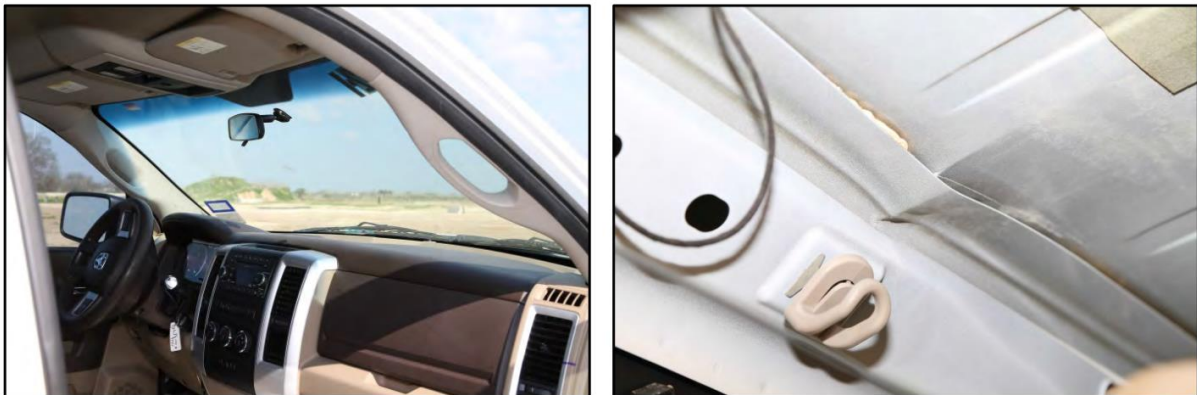
Figure 2.8. Temporary High-Mounting Sign Support, Option A Test 3-72, 90-degree Impact Vehicle Interior Damage (2)
