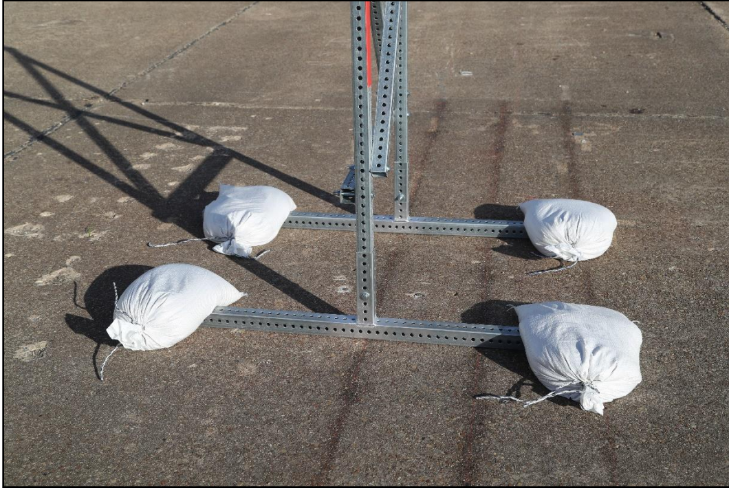
Figure 3.6. Feet with Sandbags of Tall Sign Supports for Aluminum Signs prior to Tests 618901-01-2-1-3.
