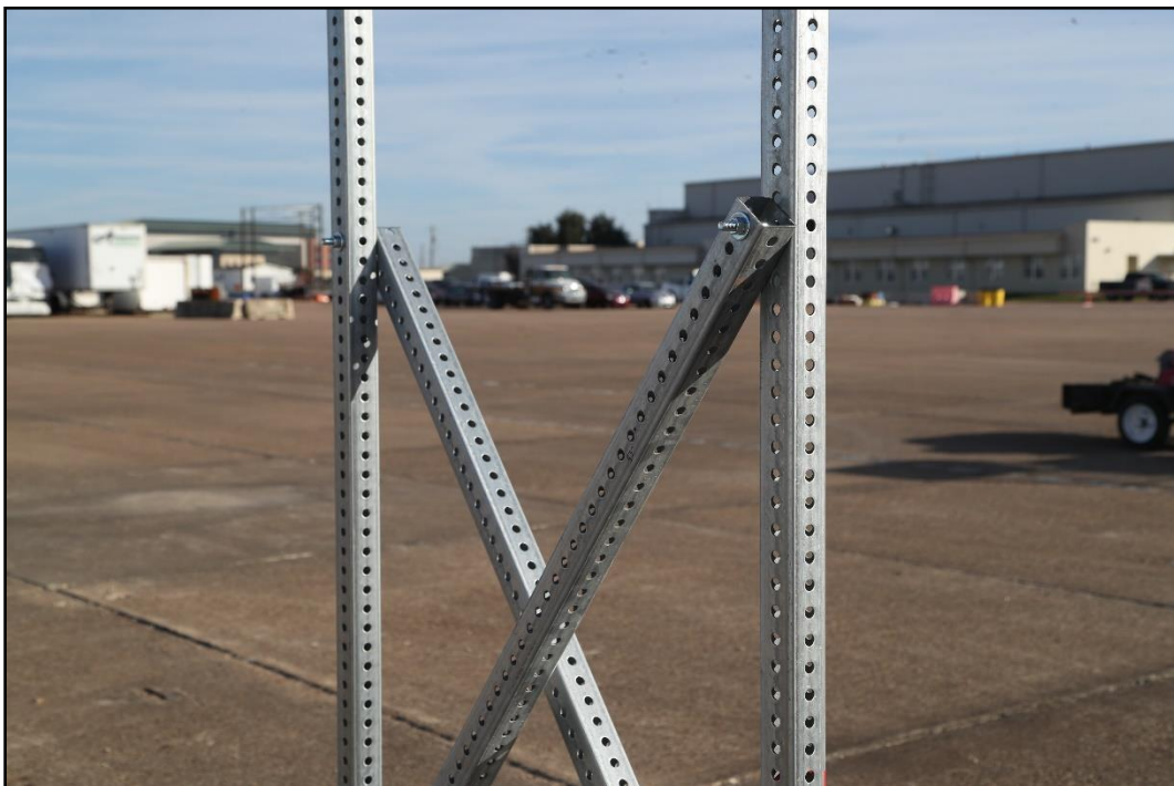
Figure 3.7. Oblique View of Cross Section of Tall Sign Supports for Aluminum Signs prior to Tests 618901-01-2-1-3.
