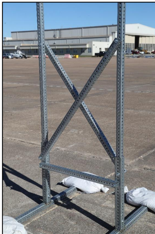
Figure 3.10. Tall Sign Supports for Aluminum Signs prior to Tests 618901-01-2-4 - 6.
