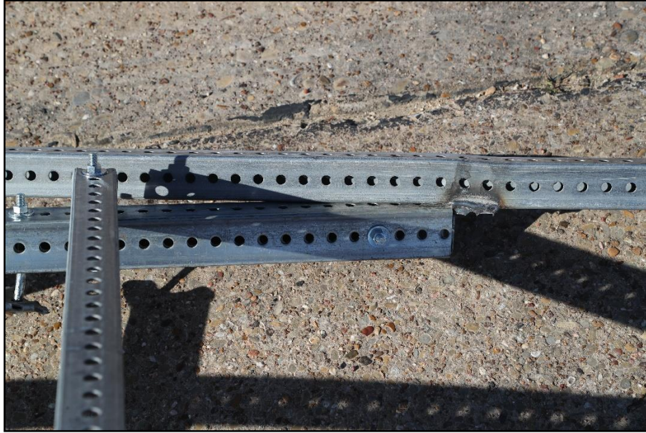
Figure 10.6. Damaged Base on the Tall Sign Supports for Aluminum Signs after Test 618901-01-2-5.
