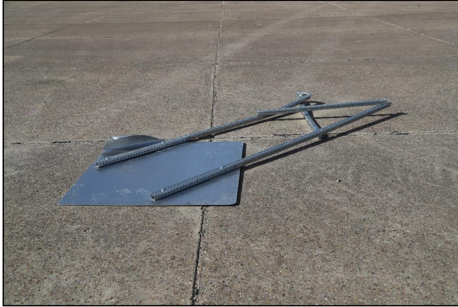
Figure 6.6. Tall Sign Supports for Aluminum Signs at Resting Position after Test 618901-01-2-1.
