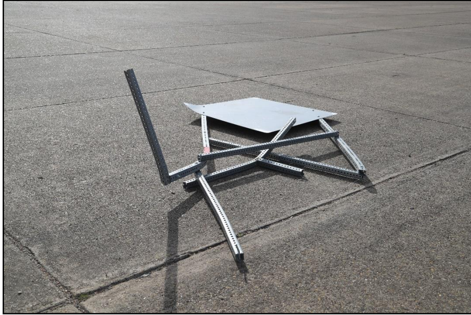
Figure 12.6. Closeup of the Tall Sign Supports for Aluminum Signs after Test 618901-01-2-7.
