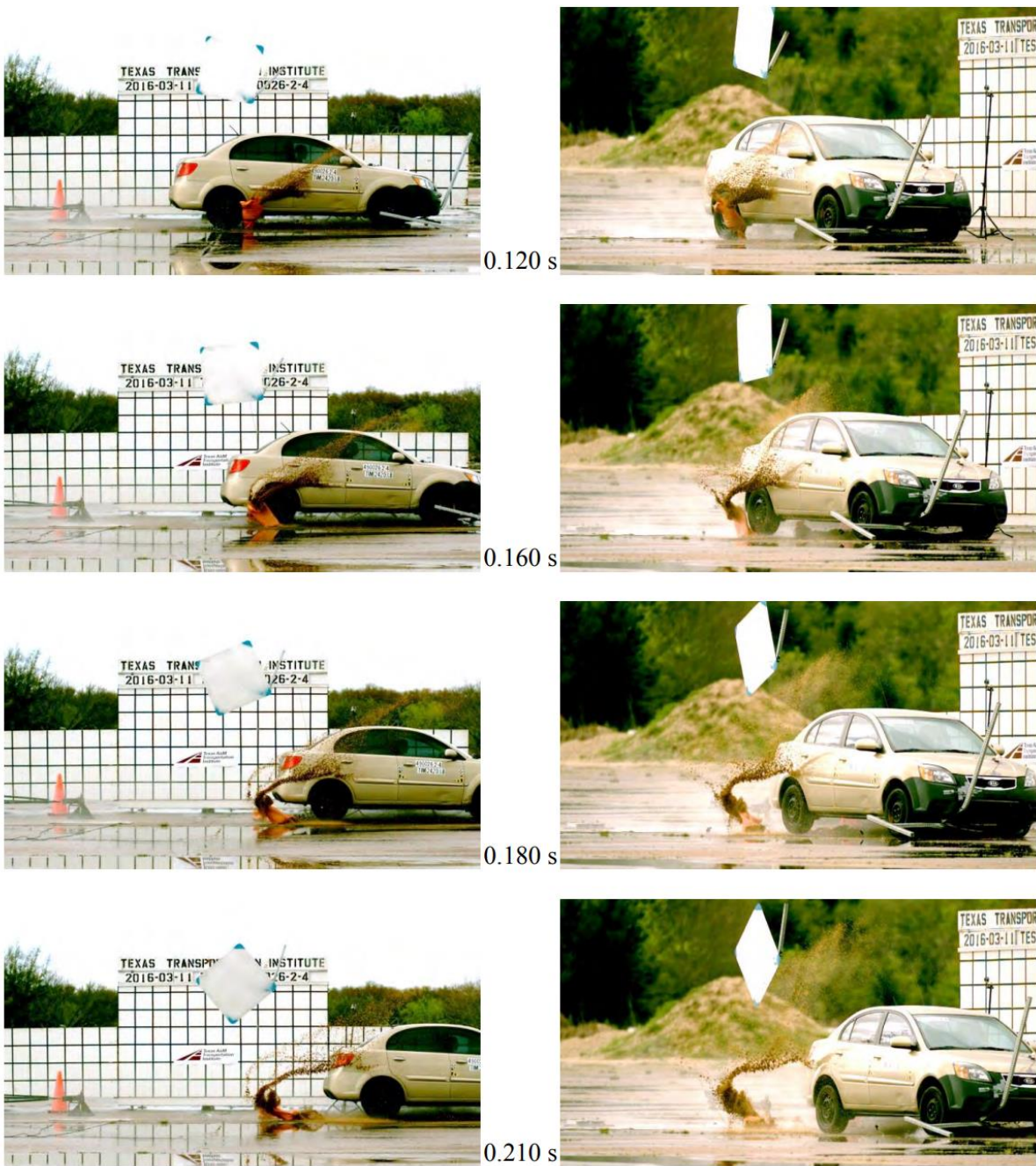
Figure 2.18. Temporary High-Mounting Sign Support, Option B Test 3-71, 90-degree Impact Sequential Photos (Continued) (2)
