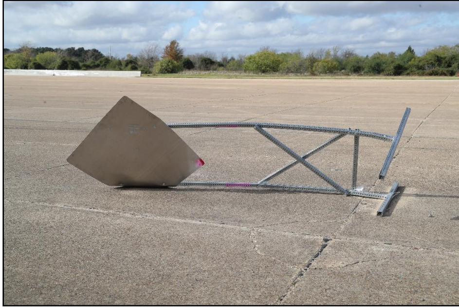
Figure 8.6. The Second Impacted Tall Sign Support for Aluminum Sign at Resting Position after Test 618901-01-2-3.
