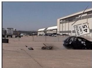
Figure 2.99. Michigan's 4x5 Portable Sign Support Test 3-71, 90-degree Impact Sequential Photos (5)
