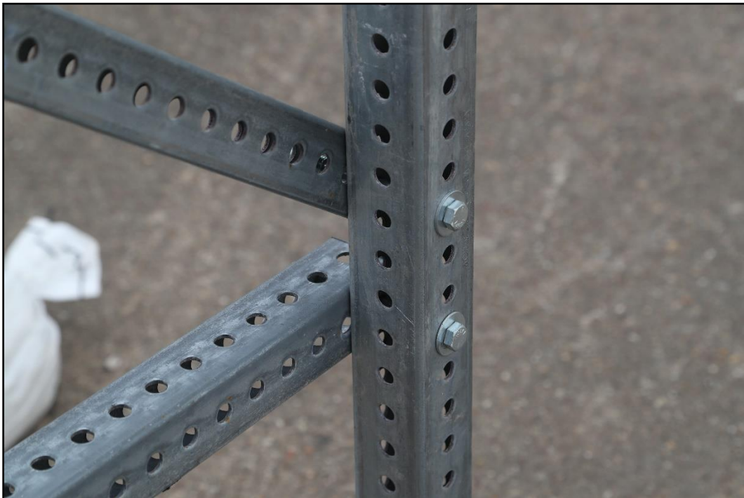
Figure 3.21. Oblique View of Cross Section of Tall Sign Supports for Aluminum Signs prior to Test 618901-01-2-7.
