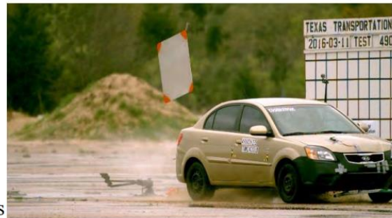
Figure 2.41. Temporary High-Mounting Sign Support, Option C Test 3-71, 0-degree Impact Sequential Photos (Continued) (2)
