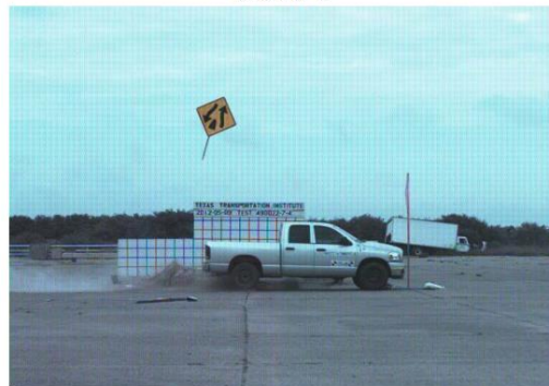
Figure 2.63. High-Mounting-Height Temporary Single Sign Support, Modified Design 2 Test 3-72, 90-degree Impact Sequential Photos (3)
