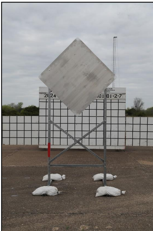
Figure 3.16. Tall Sign Supports for Aluminum Signs prior to Test 618901-01-2-7.
