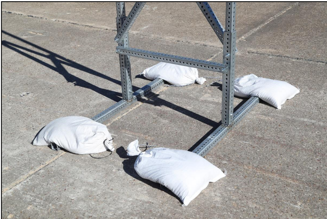
Figure 3.12. Oblique View of Cross Section of Tall Sign Supports for Aluminum Signs prior to Tests 618901-01-2-4 - 6.
