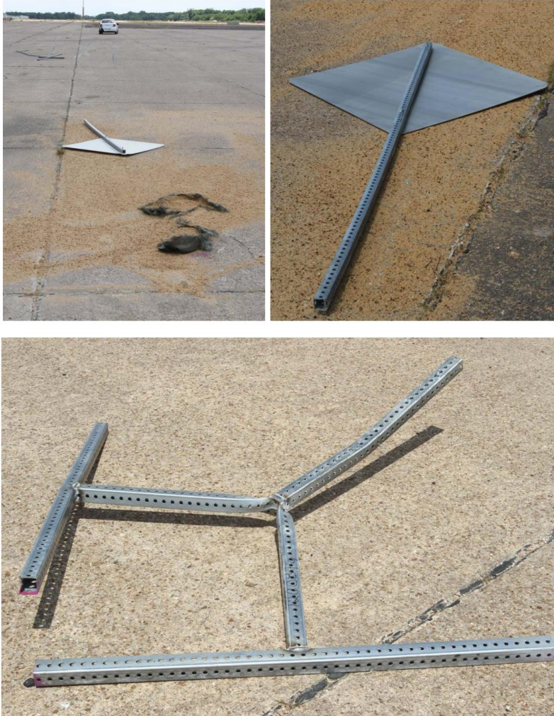
Figure 2.75. High-Mounting-Height Temporary Single Sign Support, Modified Design 4 Test 3-71, 0-degree Impact System Damage (3)
