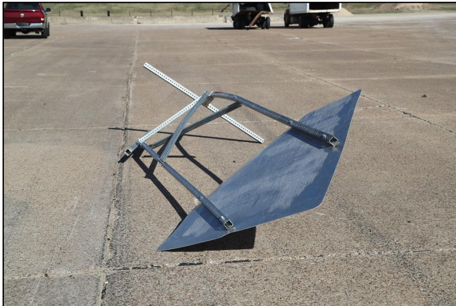
Figure 10.5. Tall Sign Supports for Aluminum Signs at Resting Position after Test 618901-01-2-5.
