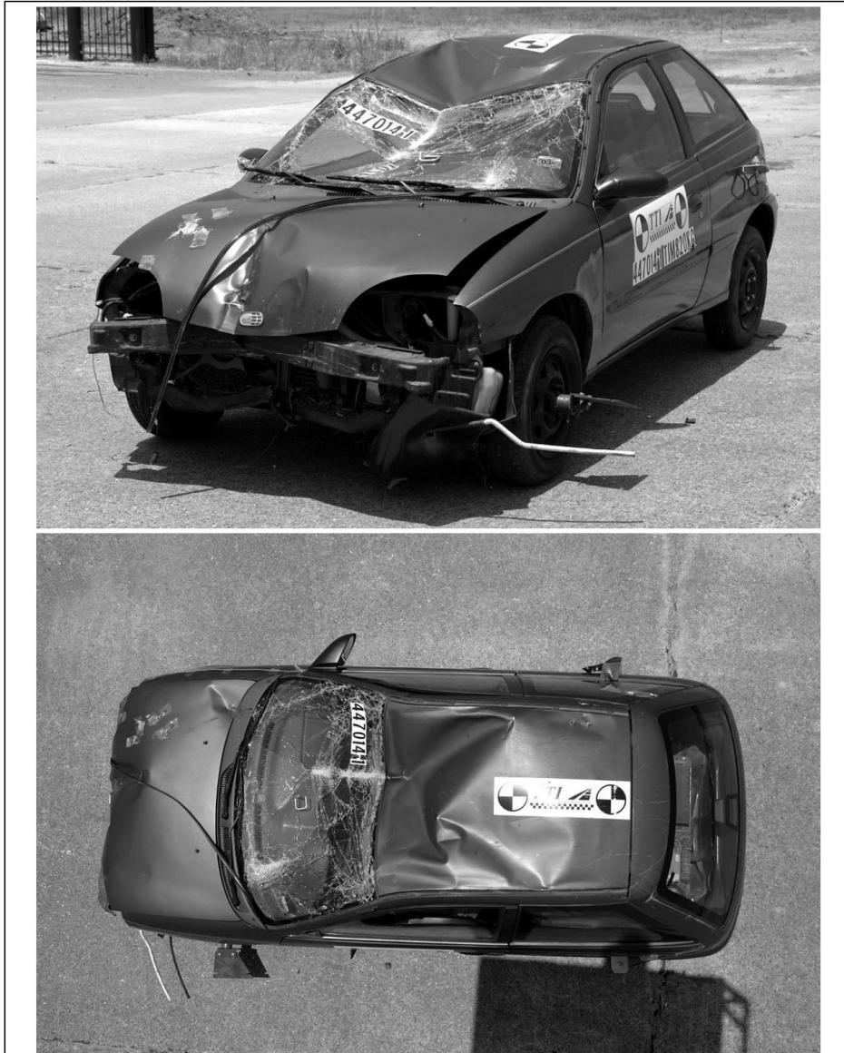
Figure 2.106. Work Zone Sign Support Test 3-71 Vehicle Damage (7)
