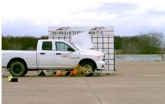
Figure 2.92. Skid-Mounted Single-Post Perforated Steel Tube Temporary Sign Support Test 3-72, 90-degree Impact Sequential Photos (4)
