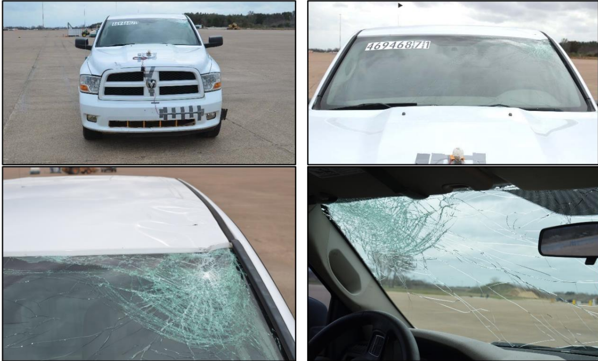
Figure 2.90. Skid-Mounted Single-Post Perforated Steel Tube Temporary Sign Support Test 3-72, 0-degree Impact Vehicle Damage (4)
