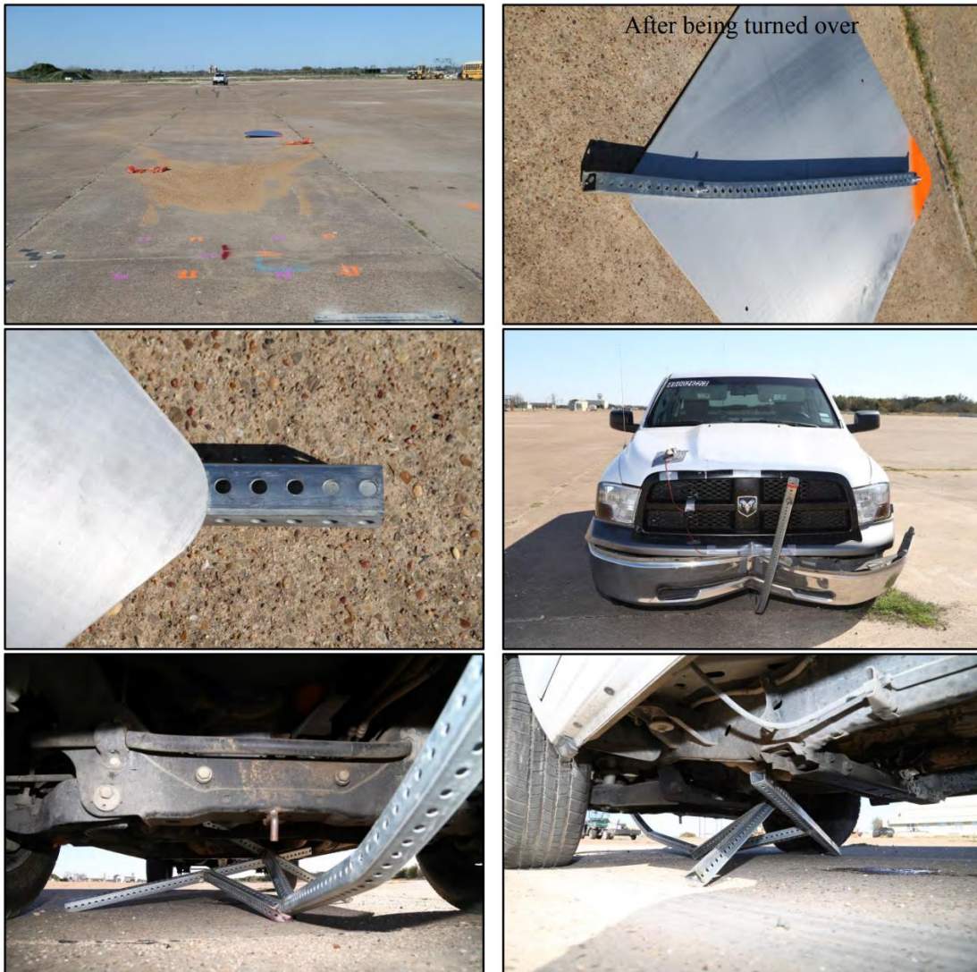
Figure 2.38. Temporary High-Mounting Sign Support, Option C Test 3-72, 90-degree Impact System Damage (2)
