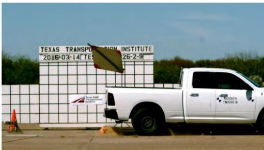
Figure 2.49. Temporary High-Mounting Sign Support, Option C Test 3-72, 0-degree Impact Sequential Photos (Continued) (2)
