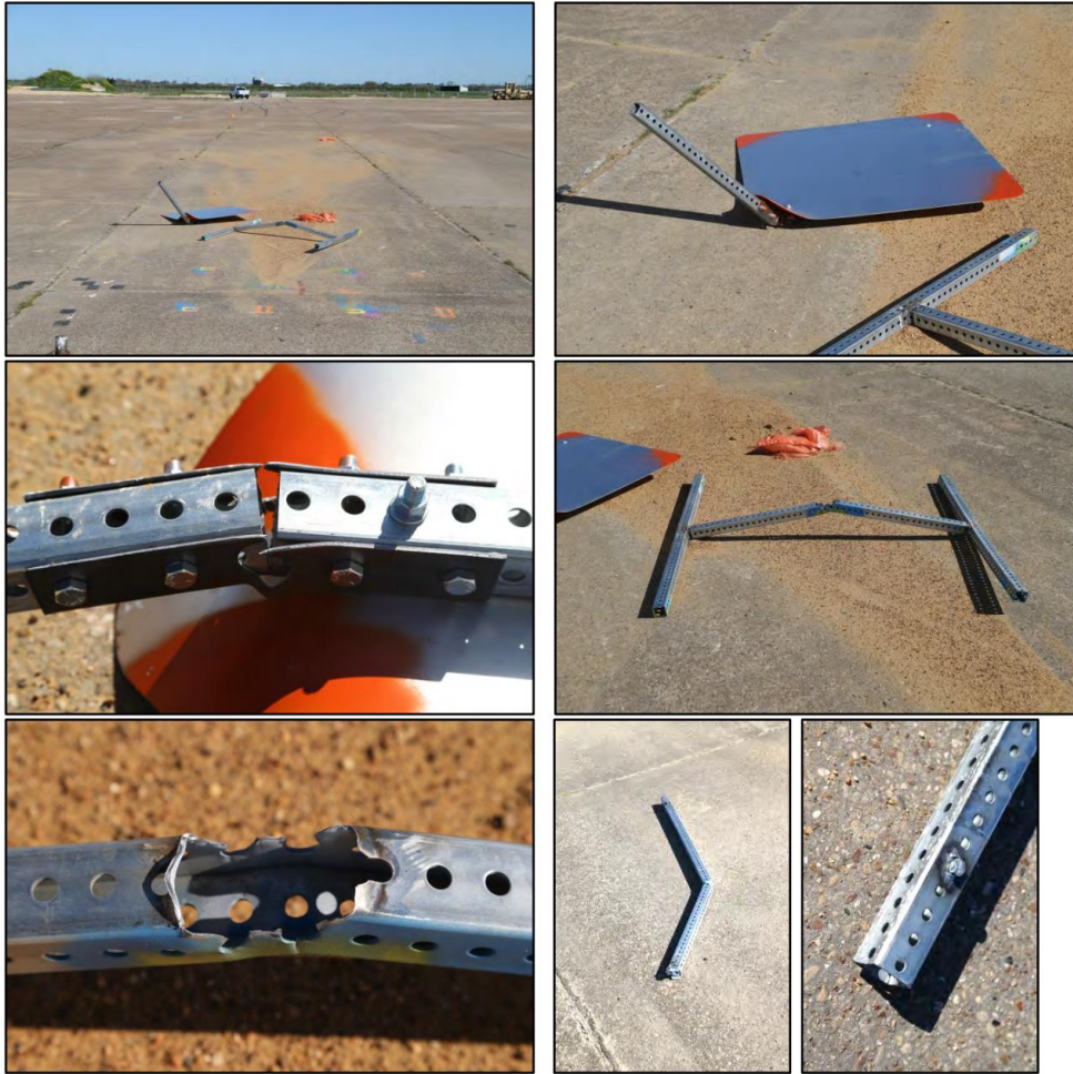
Figure 2.27. Temporary High-Mounting Sign Support, Option B Test 3-72, 0-degree Impact System Damage (2)
