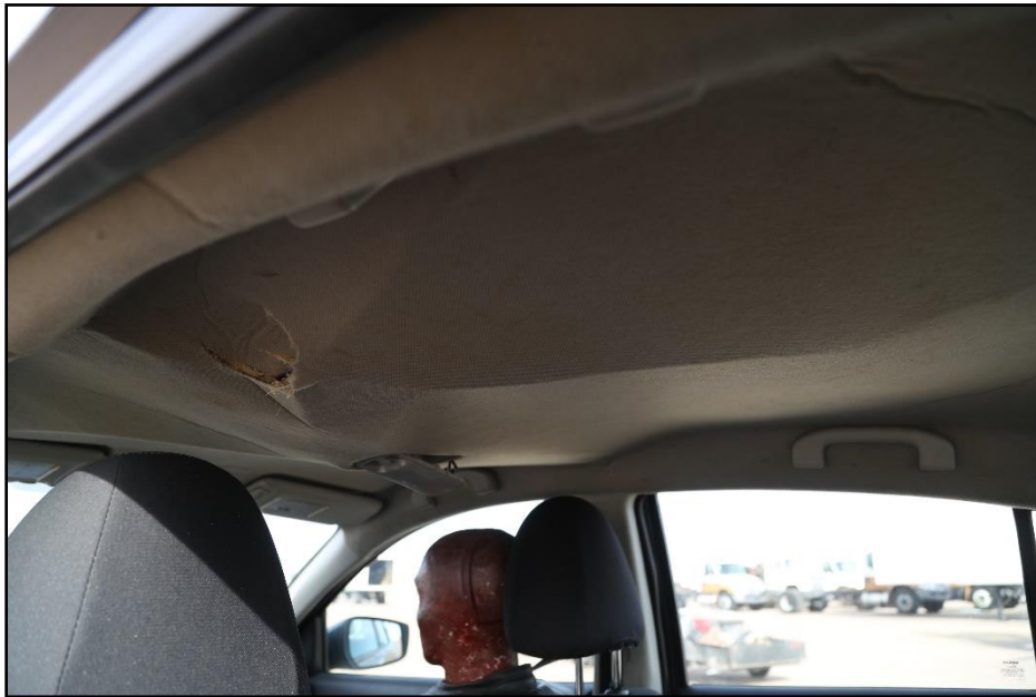
Figure 11.9. Interior Roof of Test Vehicle after Test 618901-01-2-6.
