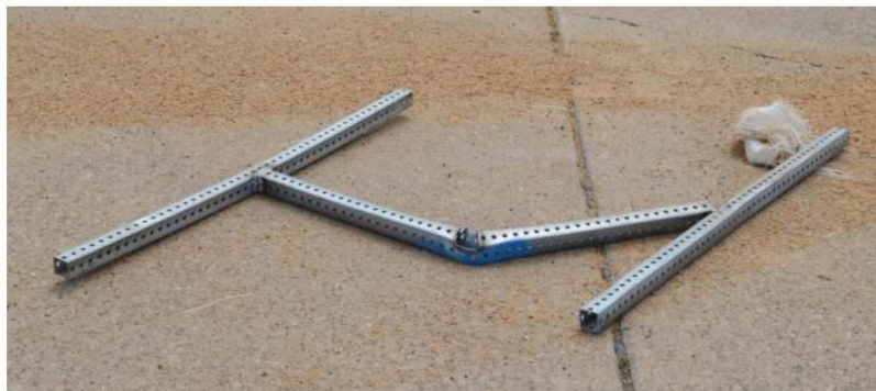
Figure 2.65. High-Mounting-Height Temporary Single Sign Support, Modified Design 2 Test 3-72 System Damage (3)
