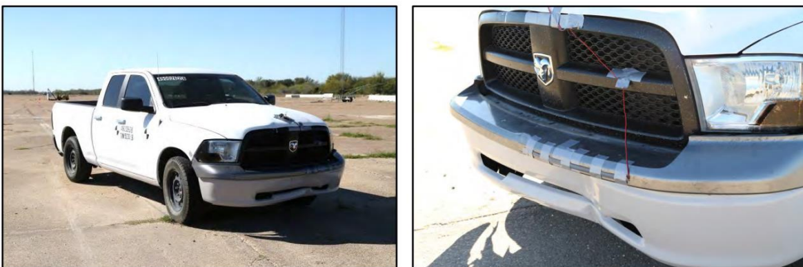
Figure 2.28. Temporary High-Mounting Sign Support, Option B Test 3-72, 0-degree Impact Vehicle Damage (2)
