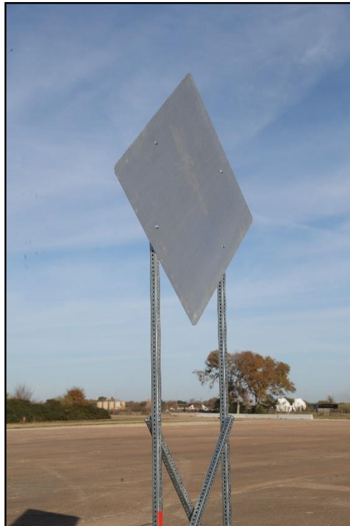
Figure 3.3. Tall Sign Supports for Aluminum Signs prior to Tests 618901-01-2-1-3.
