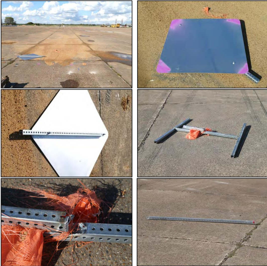
Figure 2.46. Temporary High-Mounting Sign Support, Option C Test 3-71, 0-degree Impact System Damage (2)
