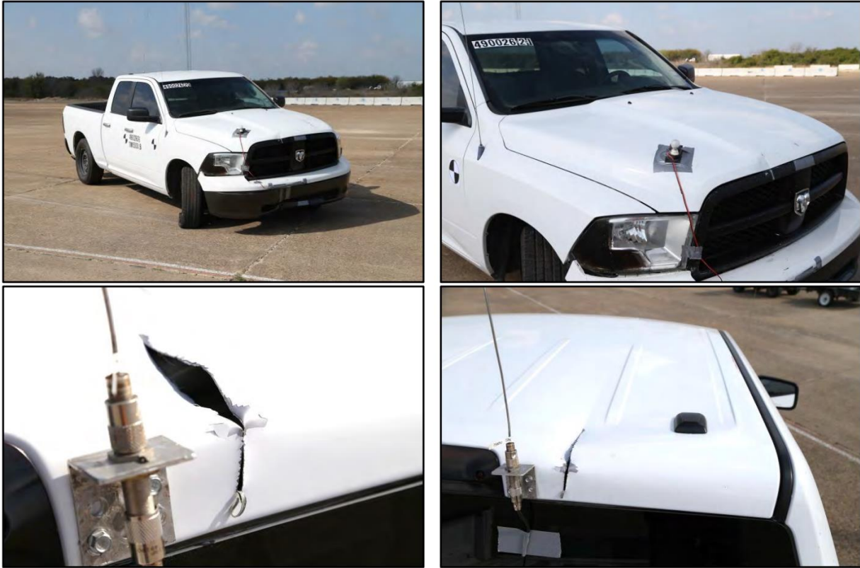
Figure 2.7. Temporary High-Mounting Sign Support, Option A Test 3-72, 90-degree Impact Vehicle Damage (2)
