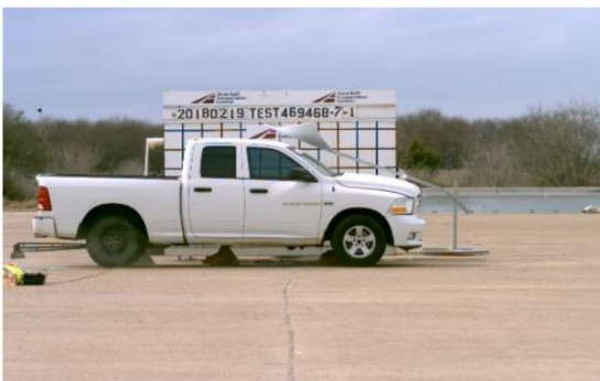
Figure 2.87. Skid-Mounted Single-Post Perforated Steel Tube Temporary Sign Support Test 3-72, 0-degree Impact Sequential Photos (4)
