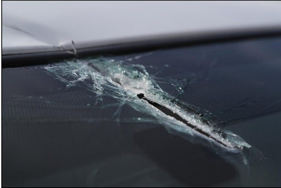
Figure 12.8. Closeup of Tear in Windshield of Test Vehicle after Test 618901-01-2-7.
