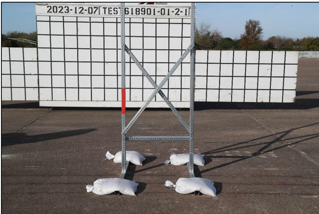
Figure 3.5. Cross Section of Tall Sign Supports for Aluminum Signs prior to Tests 618901-01-2-1-3.
