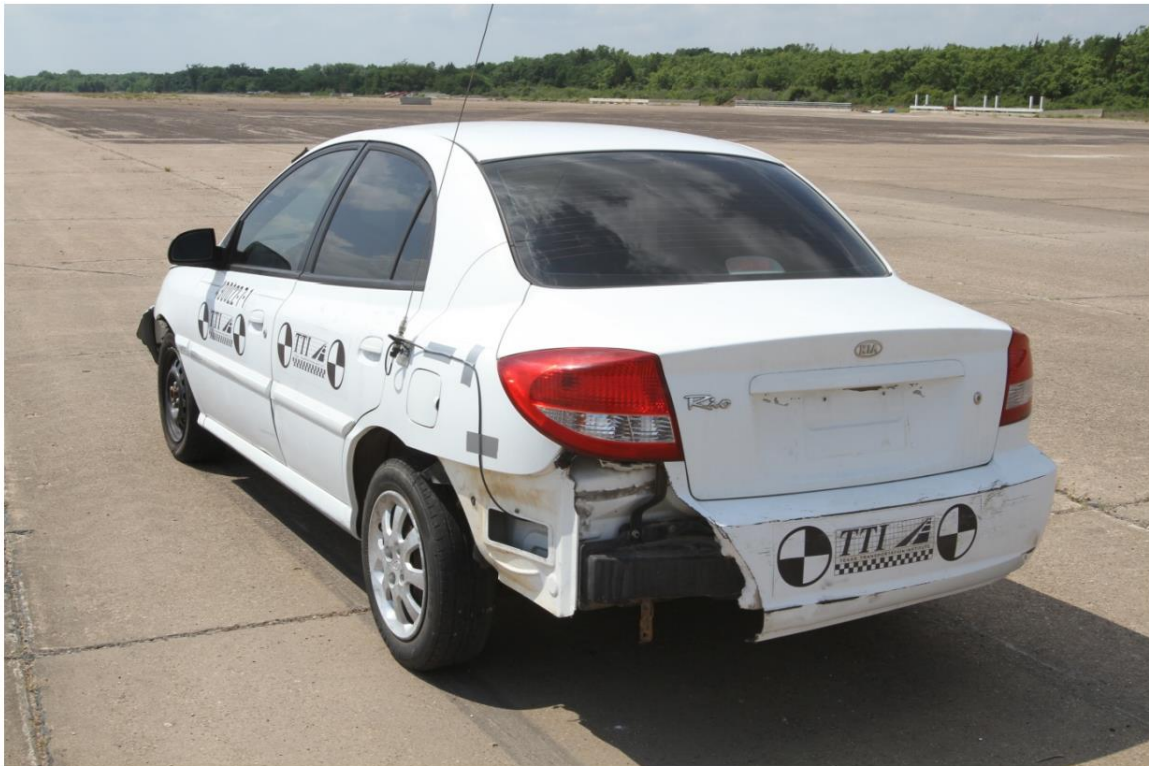
Figure 2.62. High-Mounting-Height Temporary Single Sign Support, Modified Design 2 Test 3-71, 90-degree Impact Vehicle Damage (3)
