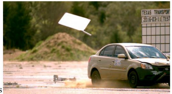
Figure 2.22. Temporary High-Mounting Sign Support, Option B Test 3-71, 0 degree Impact Sequential Photos (Continued) (2)
