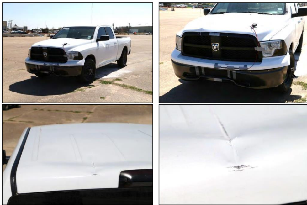
Figure 2.16. Temporary High-Mounting Sign Support, Option B Test 3-72, 90-degree Impact Vehicle Damage (2)
