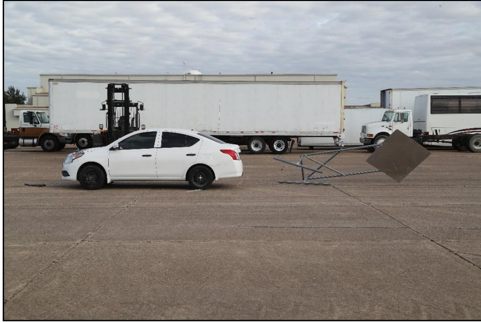
Figure 7.5. Tall Sign Supports for Aluminum Signs at Resting Position after Test 618901-01-2-2.
