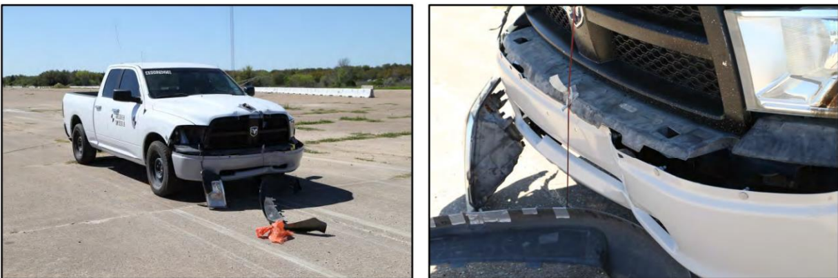
Figure 2.51. Temporary High-Mounting Sign Support, Option C Test 3-72, 0-degree Impact Vehicle Damage (2)
