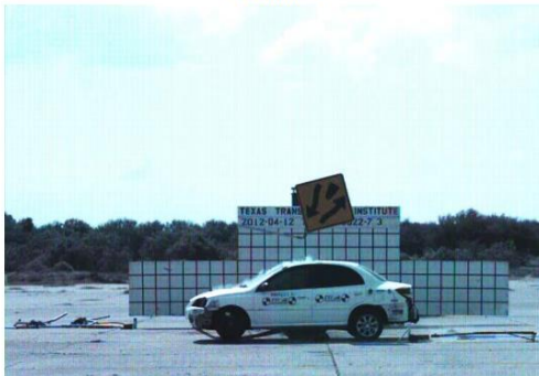
Figure 2.81. High-Mounting-Height Temporary Single Sign Support, Modified Design 8 Test 3-71, 90-degree Impact Sequential Photos (3)
