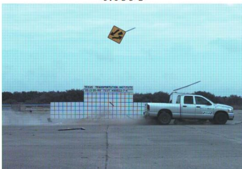
Figure 2.64. High-Mounting-Height Temporary Single Sign Support, Modified Design 2 Test 3-72, 0-degree Impact Sequential Photos (3)
