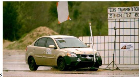
Figure 2.40. Temporary High-Mounting Sign Support, Option C Test 3-71, 90-degree Impact Sequential Photos (2)
