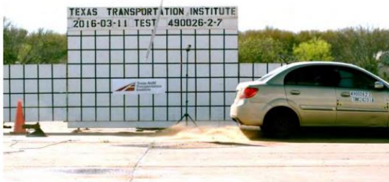
Figure 2.45. Temporary High-Mounting Sign Support, Option C Test 3-71, 0-degree Impact Sequential Photos (Continued) (2)
