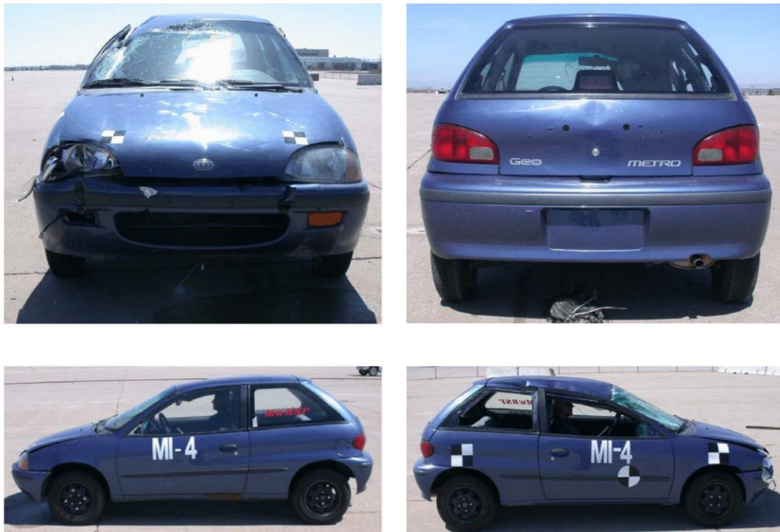
Figure 2.101. Michigan's 4x5 Portable Sign Support Test 3-71 Vehicle Damage (5)
