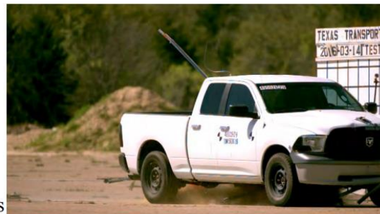
Figure 2.49. Temporary High-Mounting Sign Support, Option C Test 3-72, 0-degree Impact Sequential Photos (Continued) (2)
