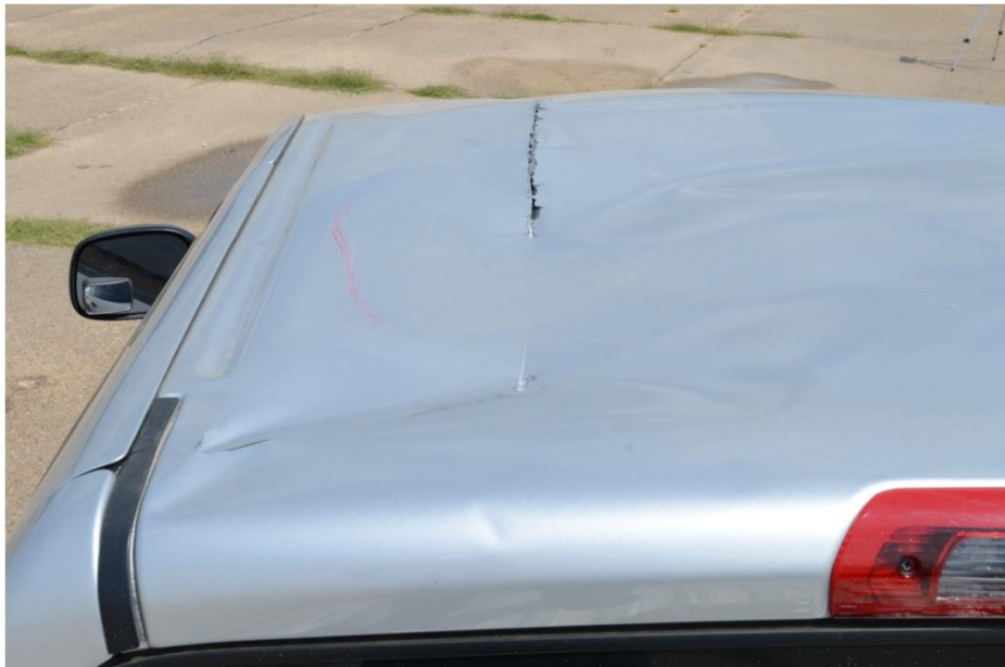
Figure 2.66. High-Mounting-Height Temporary Single Sign Support, Modified Design 2 Test 3-72 Vehicle Damage (3)
