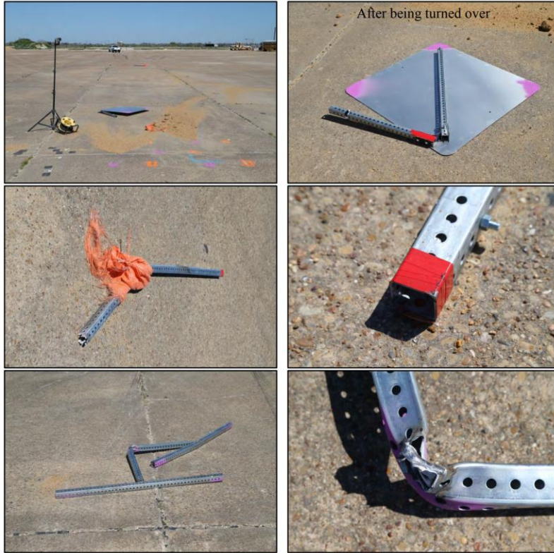
Figure 2.15. Temporary High-Mounting Sign Support, Option B Test 3-72, 90-degree Impact System Damage (2)
