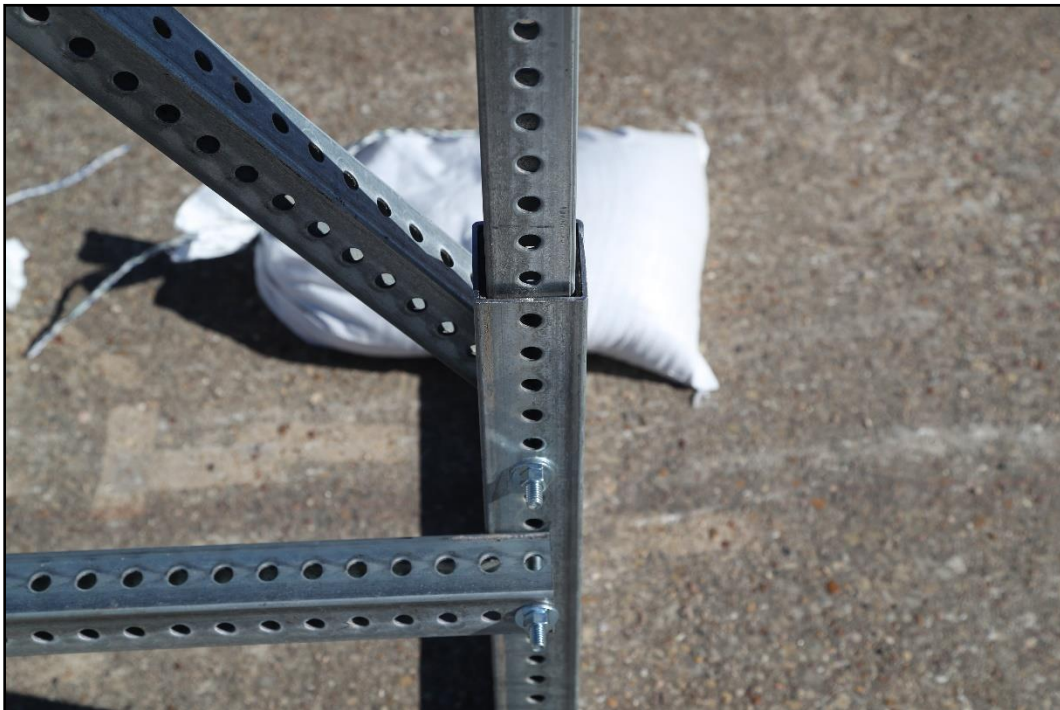
Figure 3.14. Cross Section of Tall Sign Supports for Aluminum Signs prior to Tests 618901-01-2-4 - 6.
