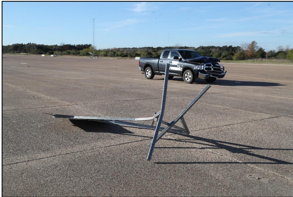
Figure 9.5. Tall Sign Supports for Aluminum Signs at Resting Position after Test 618901-01-2-4.
