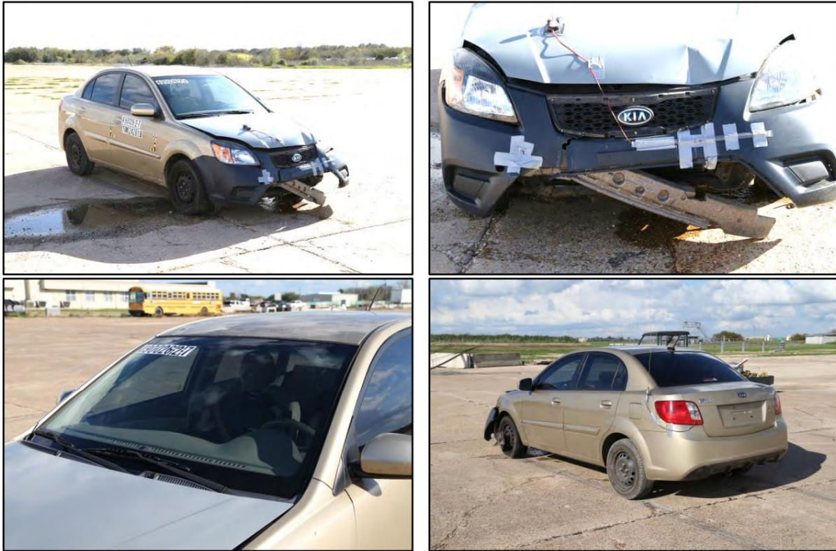
Figure 2.47. Temporary High-Mounting Sign Support, Option C Test 3-71, 0-degree Impact Vehicle Damage (2)
