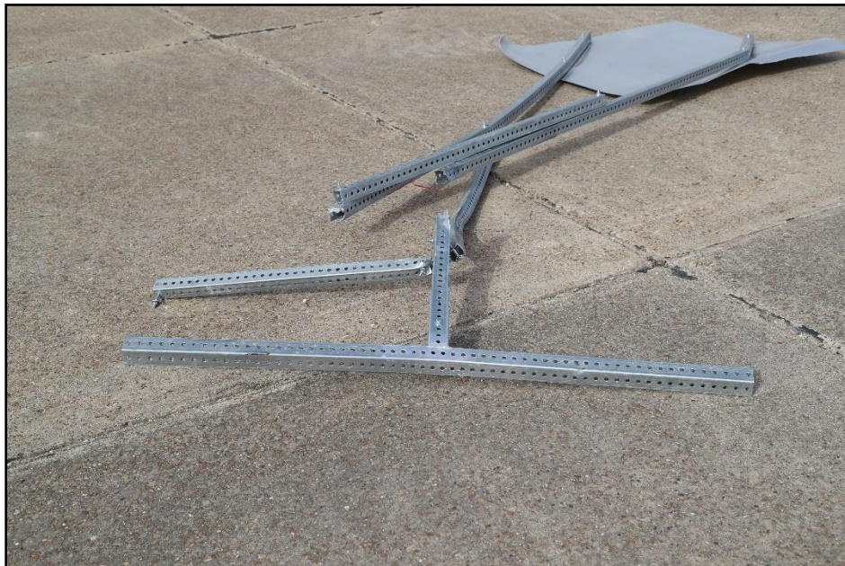
Figure 8.5. The First Impacted Tall Sign Support for Aluminum Sign at Resting Position after Test 618901-01-2-3.
