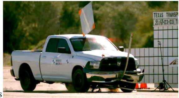
Figure 2.36. Temporary High-Mounting Sign Support, Option C Test 3-72, 90-degree Impact Sequential Photos (2)
