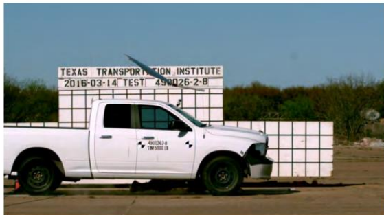
Figure 2.25. Temporary High-Mounting Sign Support, Option B Test 3-72, 0-degree Impact Sequential Photos (2)
