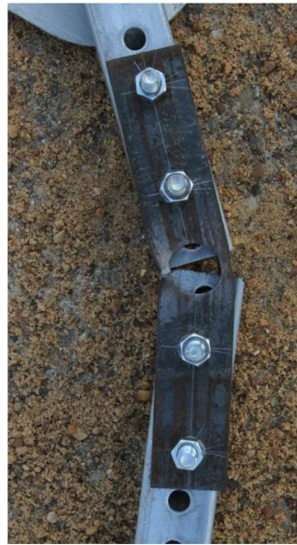
Figure 2.82. High-Mounting-Height Temporary Single Sign Support, Modified Design 8 Test 3-71, 90-degree Impact System Damage (3)
