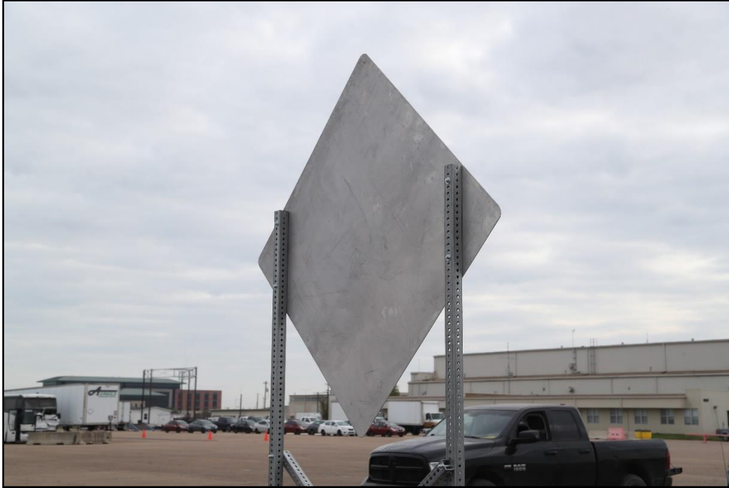
Figure 3.18. Field Side View of Tall Sign Supports for Aluminum Signs prior to Test 618901-01-2-7.
