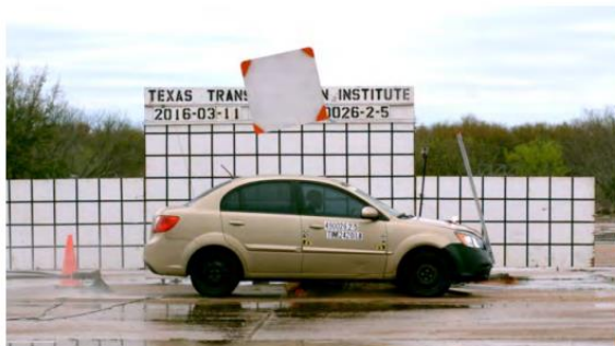
Figure 2.40. Temporary High-Mounting Sign Support, Option C Test 3-71, 90-degree Impact Sequential Photos (2)
