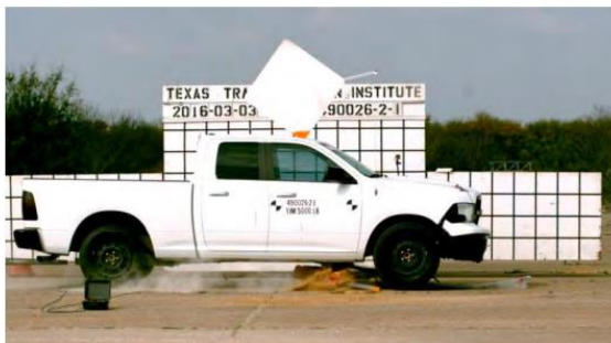
Figure 2.4. Temporary High-Mounting Sign Support, Option A Test 3-72, 90-degree Impact Sequential Photos (2)
