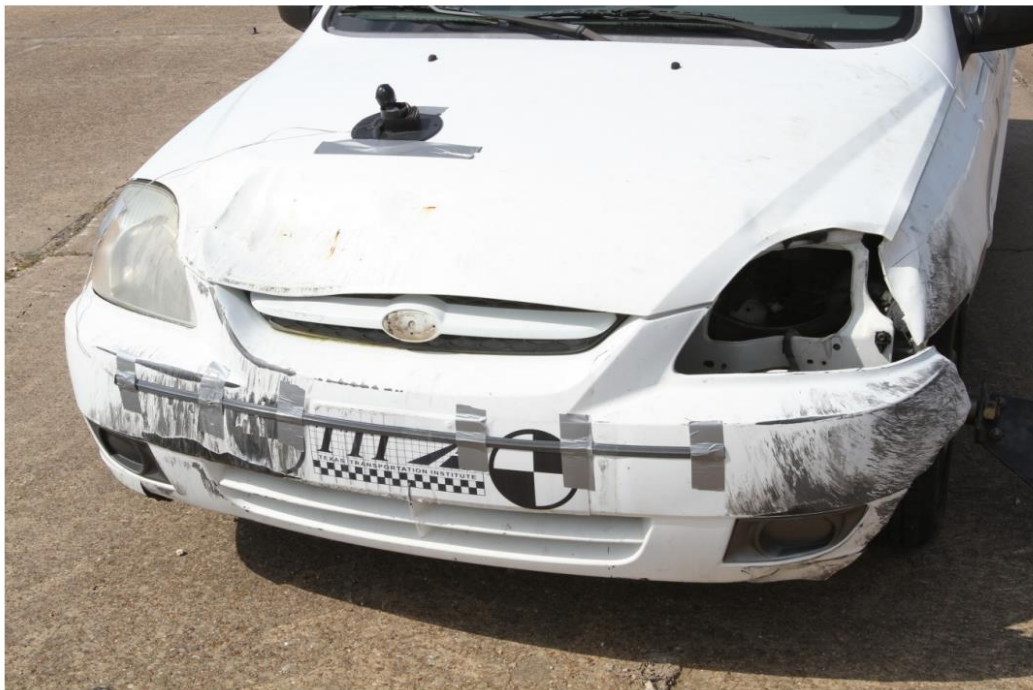
Figure 2.83. High-Mounting-Height Temporary Single Sign Support, Modified Design 8 Test 3-71, 90-degree Impact Vehicle Damage (3)
