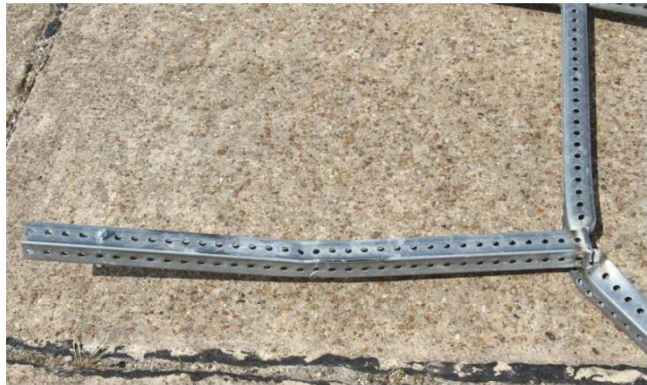
Figure 2.61. High-Mounting-Height Temporary Single Sign Support, Modified Design 2 Test 3-71, 90-degree Impact System Damage (3)
