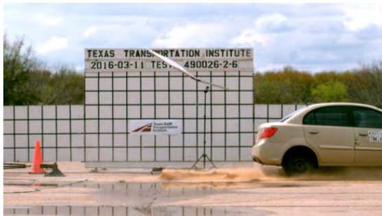
Figure 2.22. Temporary High-Mounting Sign Support, Option B Test 3-71, 0 degree Impact Sequential Photos (Continued) (2)
