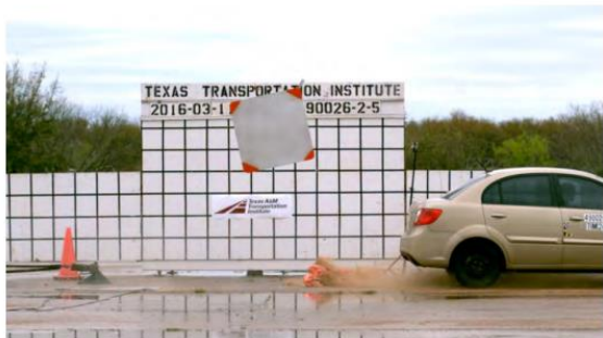
Figure 2.41. Temporary High-Mounting Sign Support, Option C Test 3-71, 0-degree Impact Sequential Photos (Continued) (2)
