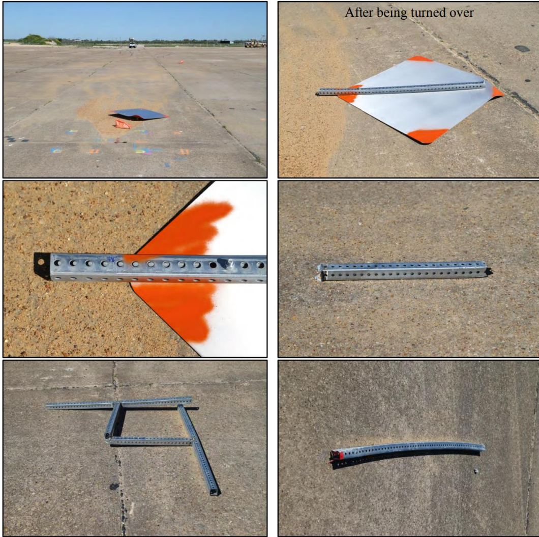
Figure 2.50. Temporary High-Mounting Sign Support, Option C Test 3-72, 0-degree Impact System Damage (2)
