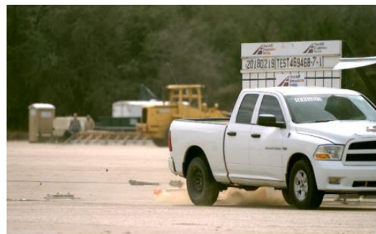
Figure 2.88. Skid-Mounted Single-Post Perforated Steel Tube Temporary Sign Support Test 3-72, 0-degree Impact Sequential Photos (Continued) (4)
