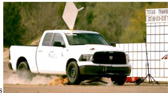
Figure 2.4. Temporary High-Mounting Sign Support, Option A Test 3-72, 90-degree Impact Sequential Photos (2)
