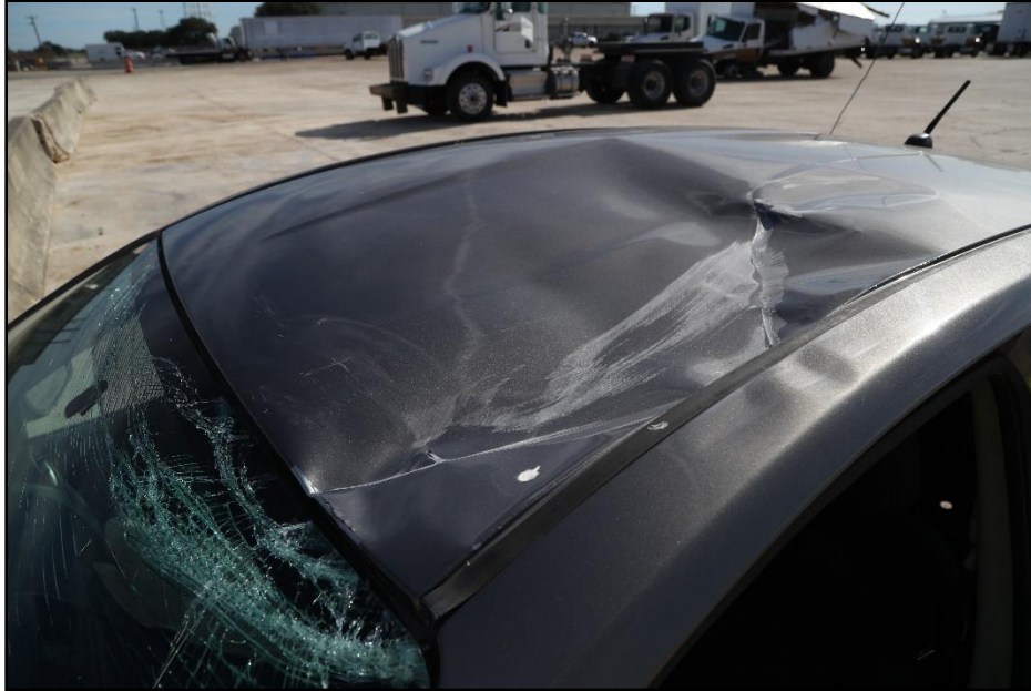
Figure 6.8. Roof of Test Vehicle after Test 618901-01-2-1.
