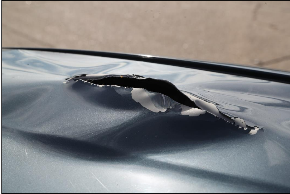
Figure 11.8. Closeup of Tear in Roof of Test Vehicle after Test 618901-01-2-6.
