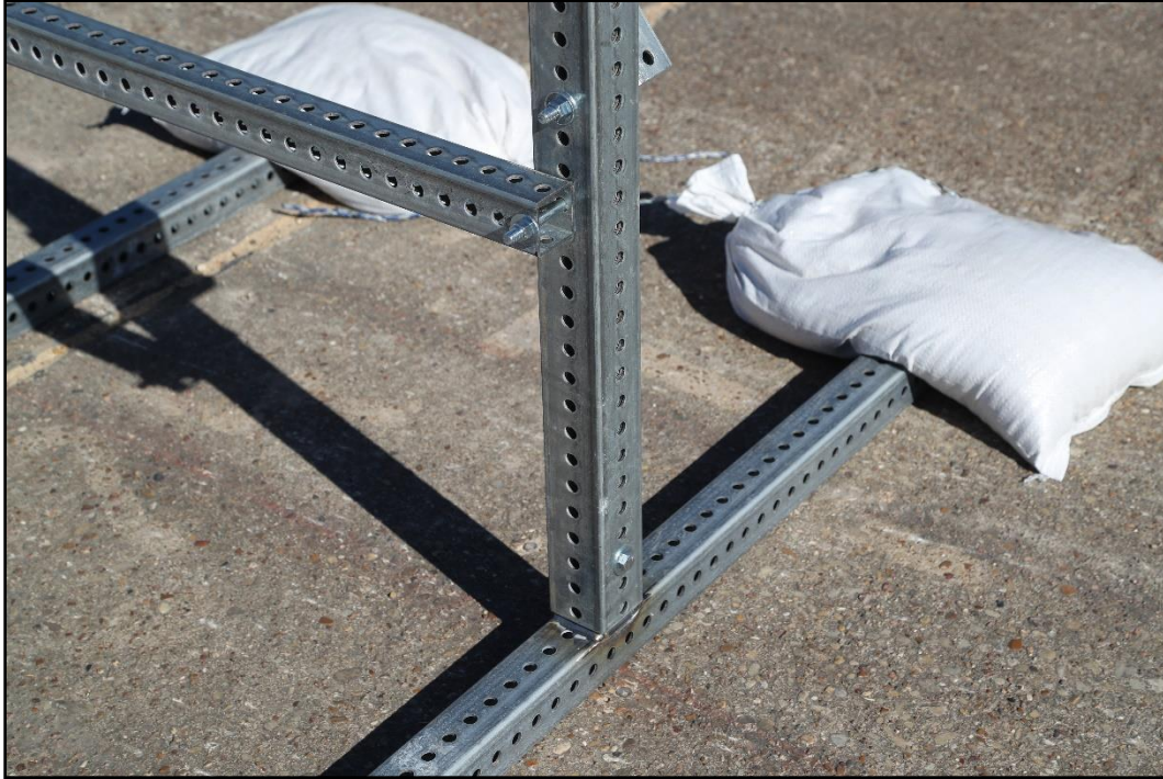
Figure 3.13. Feet with Sandbags of Tall Sign Supports for Aluminum Signs prior to Tests 618901-01-2-4 - 6.
