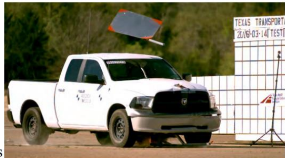
Figure 2.25. Temporary High-Mounting Sign Support, Option B Test 3-72, 0-degree Impact Sequential Photos (2)
