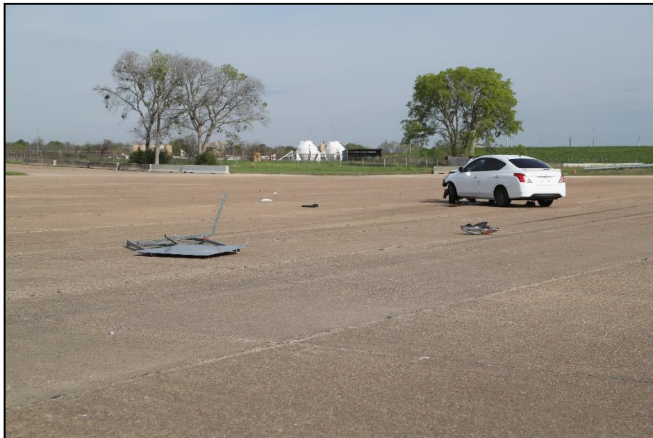
Figure 12.5. Tall Sign Supports for Aluminum Signs at Resting Position after Test 618901-01-2-7.
