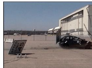
Figure 2.99. Michigan's 4x5 Portable Sign Support Test 3-71, 90-degree Impact Sequential Photos (5)
