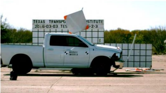
Figure 2.36. Temporary High-Mounting Sign Support, Option C Test 3-72, 90-degree Impact Sequential Photos (2)
