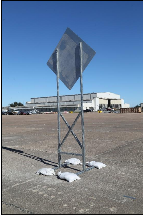
Figure 3.9. Tall Sign Supports for Aluminum Signs prior to Tests 618901-01-2-4 - 6.
